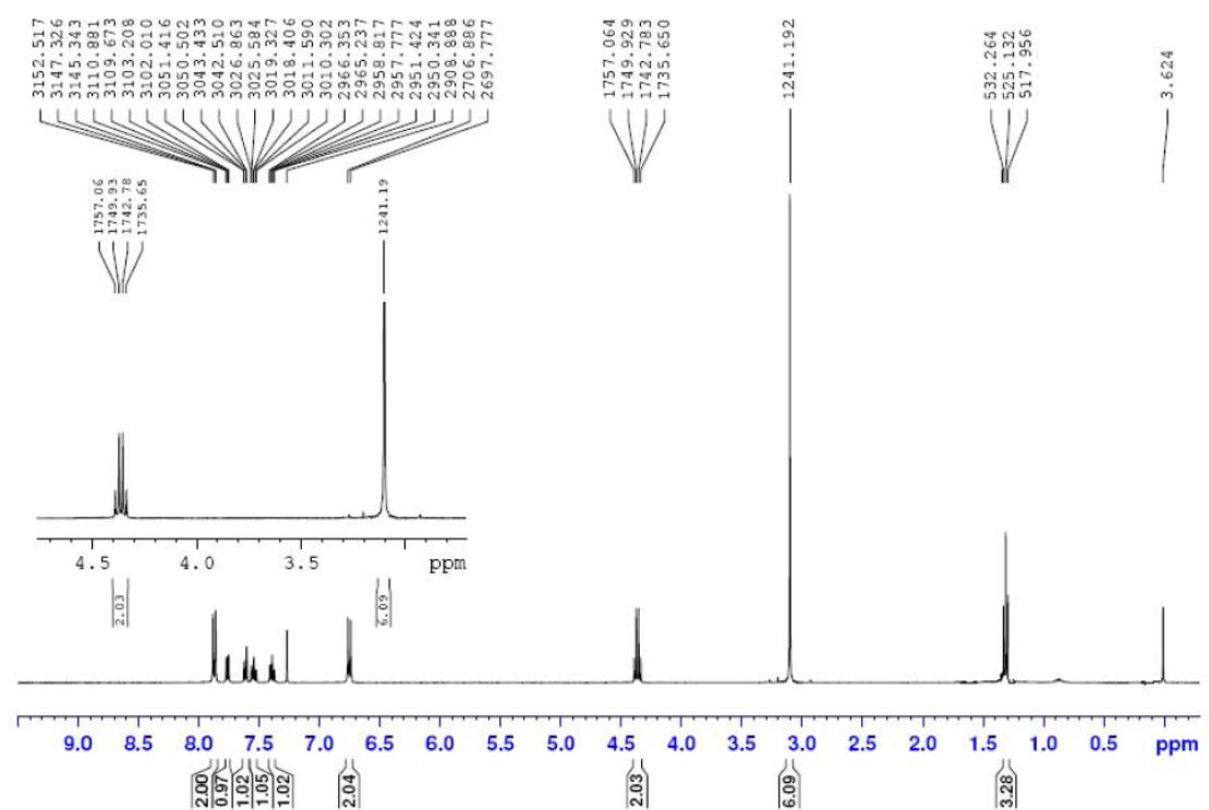
Figure 3S: <sup>1</sup>H-NMR spectrum of ethyl ester of methyl red
