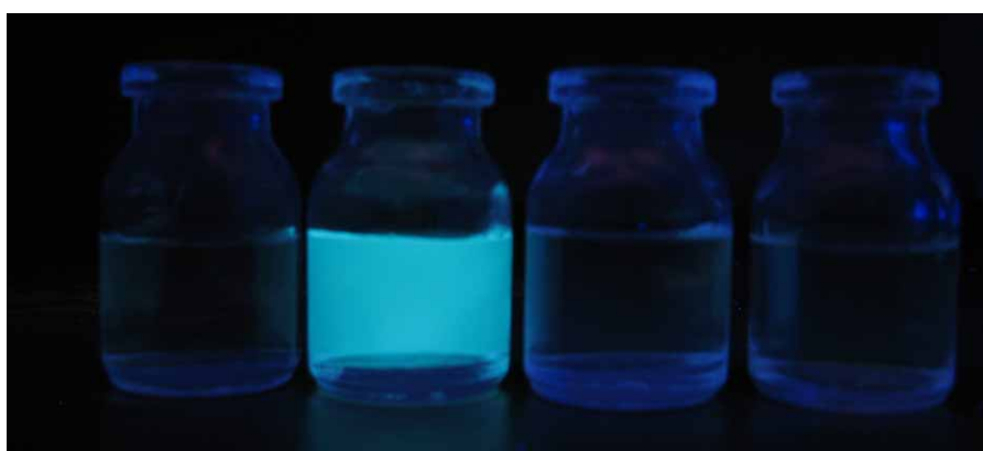
Fig. S4 Visible emission observed from samples of DHC and CB7, \beta -CD and glycoluril. Left to right: DHC, DHC + CB7, DHC + \beta -CD and P + glycoluril.
