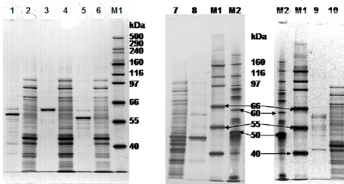
**Fig.1** SDS-PAGE: *Lane 1&2* – insoluble & soluble fraction of CBDclos-SPO0224; *Lane 3&4* – insoluble & soluble fraction of CBDclos-SPO1256; *Lane 5&6* – insoluble & soluble fraction of CBDclos-SPO1727; *Lane 7&8* – soluble & insoluble fraction of CBDclos-b0910; *Lane 9&10* – insoluble & soluble fraction of CBDclos-Hd0053; *M1&M2* – marker proteins whose molecular masses are indicated in the picture; insoluble fractions were 20-times diluted in comparison with soluble fractions.
