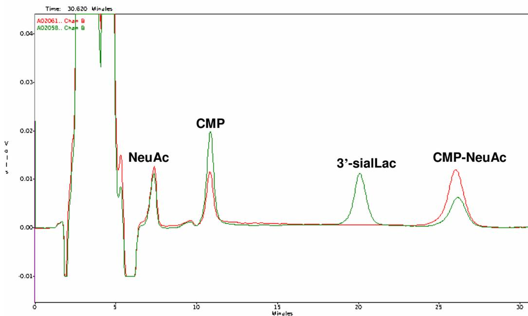
**Fig. 3** HPLC of 3'-sialyllactose synthesis. Time 0 – red line, time 3 h – green line. Isocratic elution with mobile phase composed from 60% acetonitrile and 40% acid water solution (50 mM H<sub>3</sub>PO<sub>4</sub>, 10 mM MgCl<sub>2</sub>), at a flow rate of 0.5 ml/min. RI detector.
