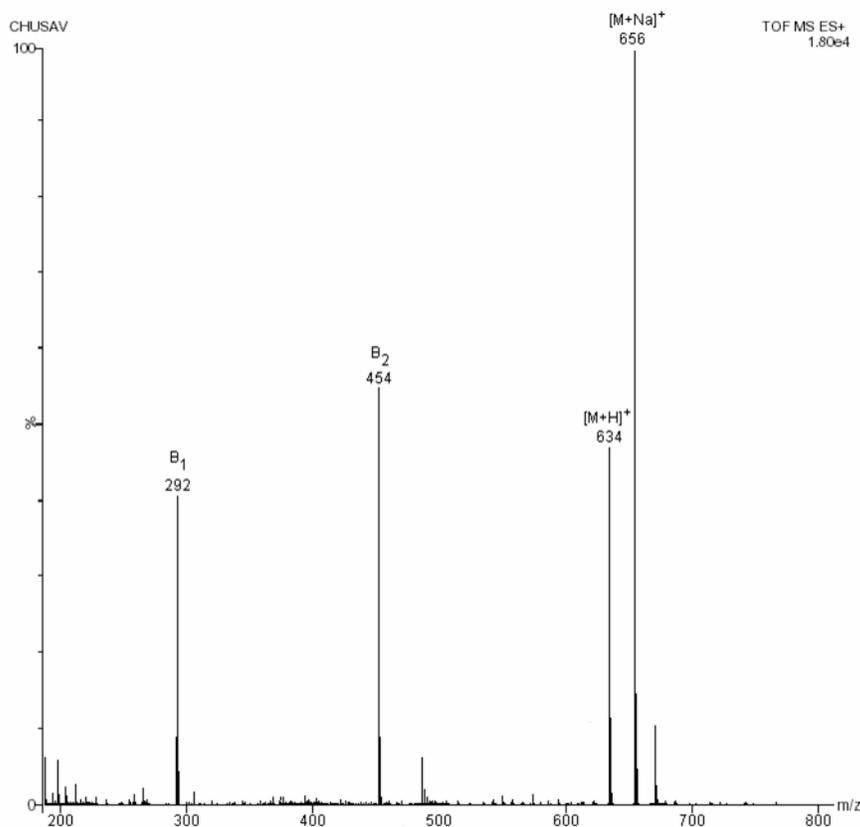
**Fig. 4** HPLC–ESI-MS of 3'-sialyllactose synthesis. NH<sub>2</sub> Phenosphere column (150 mm × 2.0 mm I.D., 5 μm) from Phenomenex, Torrance, CA, USA. Acetonitrile and water (85:15, v/v), flow 1ml.min<sup>-1</sup> was used as a mobile phase in isocratic HPLC coupled to electrospray ionization. Electrospray source in positive and negative mode was operated under experimental condition of splitting ratio 1:25, scan range 150 – 900, acceleration potential 3 500V.
