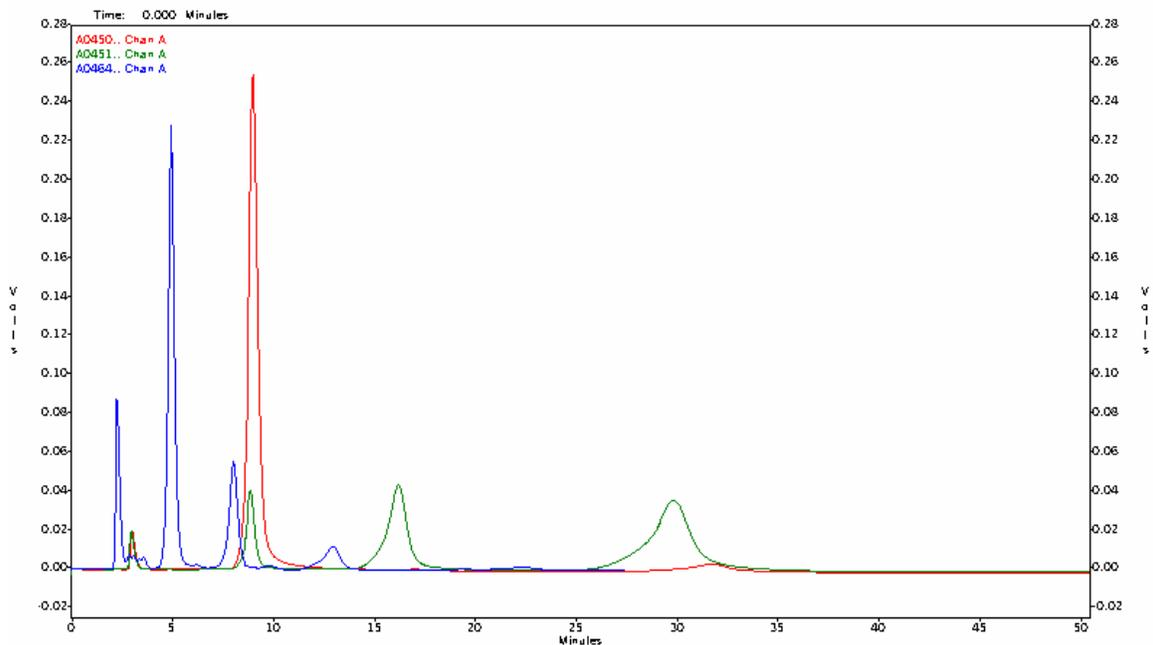
**Fig. 2** HPLC of CMP-NeuAc synthesis. Time 0 – red line; time 1 h – green line; time 12 h - blue line, 254 nm. Isocratic elution with 50 mM H<sub>3</sub>PO<sub>4</sub>, 10 mM MgCl<sub>2</sub> (pH 6.4, triethylamine) at a flow rate of 0.5 ml/min.
