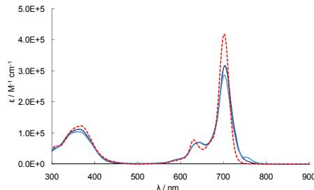
**Fig. S8** UV-vis spectra of **1** in  $CH_2Cl_2$  (deep to light blue solid lines:  $0.5 \times 10^{-5}$  to  $10^{-6}$  M, red dotted line: with 1 vol% of pyridine).
