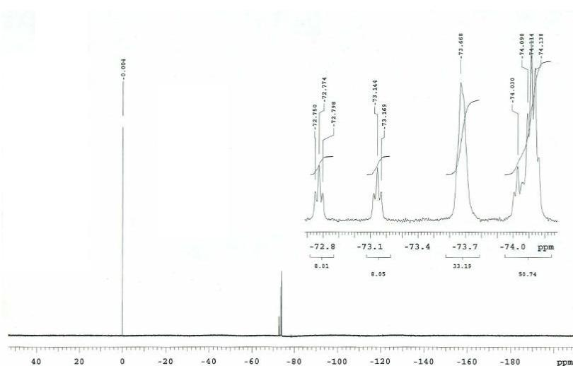
**Fig. S2** <sup>19</sup>F NMR spectra of **1** (376 MHz in acetone-*d*<sub>6</sub>).
