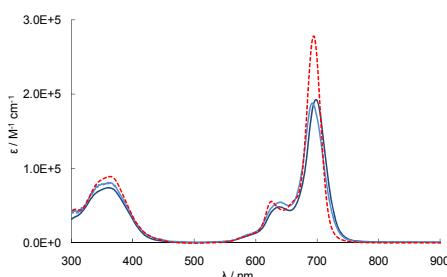
**Fig. S11** UV-vis spectra of **1** in Solkane® (CF<sub>3</sub>CH<sub>2</sub>CF<sub>2</sub>CH<sub>3</sub>) (deep to light blue solid lines: 0.5 × 10<sup>-4</sup> to 10<sup>-6</sup> M, red dotted line: with 1 vol% of pyridine).
