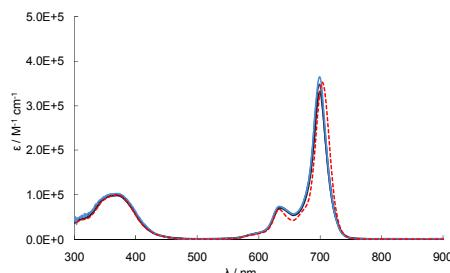
**Fig. S9** UV-vis spectra of **1** in PhCN (deep to light blue solid lines:  $0.5 \times 10^{-4}$  to  $10^{-6}$  M, red dotted line: with 1 vol% of pyridine).
