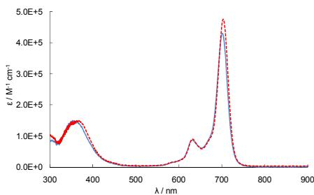
**Fig. S14** UV-vis spectra of **6** in  $\text{CHCl}_3$  (light blue:  $3.0 \times 10^{-7}$  M, red dotted: with 1 vol% of pyridine).
