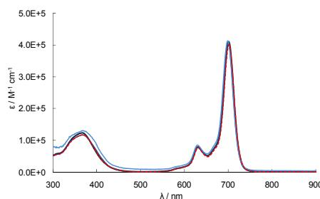
**Fig. S7** UV-vis spectra of **1** in DMF (deep to light blue solid lines:  $0.5 \times 10^{-4}$  to  $10^{-6}$  M, red dotted line: with 1 vol% of pyridine).
