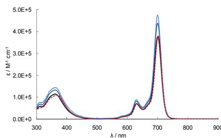
**Fig. S5** UV-vis spectra of **1** in THF (deep to light blue solid lines:  $0.5 \times 10^{-4}$  to  $10^{-6}$  M, red dotted line: with 1 vol% of pyridine).
