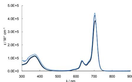
**Fig. S6** UV-vis spectra of **1** in pyridine (deep to light blue solid lines:  $0.5 \times 10^{-4}$  to  $10^{-6}$  M).
