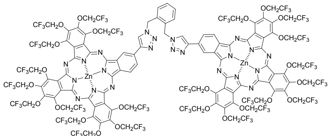
A mixture of **3** (40.2 mg, 0.0226 mmol), 1,2-bis(azidomethyl)benzene **5a** (1.7 mg, 0.009 mmol), CuI (1.0 mg, 0.005 mmol), Et<sub>3</sub>N (0.05 ml) and DMSO (0.8 ml) was freeze dried to remove oxygen, and stirred at 60 °C for 2 h. After cooling it to rt, water and dil. sulfuric acid were added and the precipitates were filtered. Purification by silica gel column chromatography (hexane : acetone = 70: 30 to 60 : 40) gave green solids. 32.1 mg, 95%.
