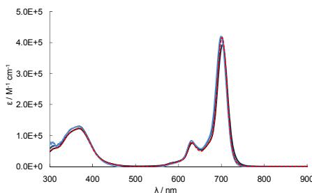
**Fig. S10** UV-vis spectra of **1** in *m*-C<sub>6</sub>H<sub>4</sub>F<sub>2</sub> (deep to light blue solid lines: 0.5 × 10<sup>-4</sup> to 10<sup>-6</sup> M, red dotted line: with 1 vol% of pyridine).
