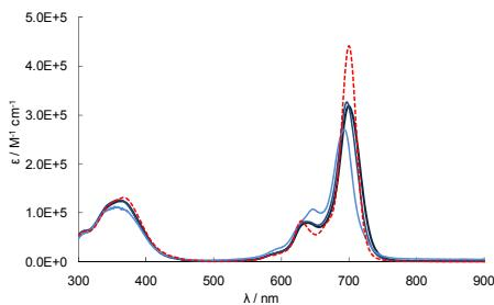
**Fig. S15** UV-vis spectra of **6** in  $\text{PhCF}_3$  (deep to light blue solid lines:  $0.5 \times 10^{-4}$  to  $10^{-6}$  M, red dotted line: with 1 vol% of pyridine).
