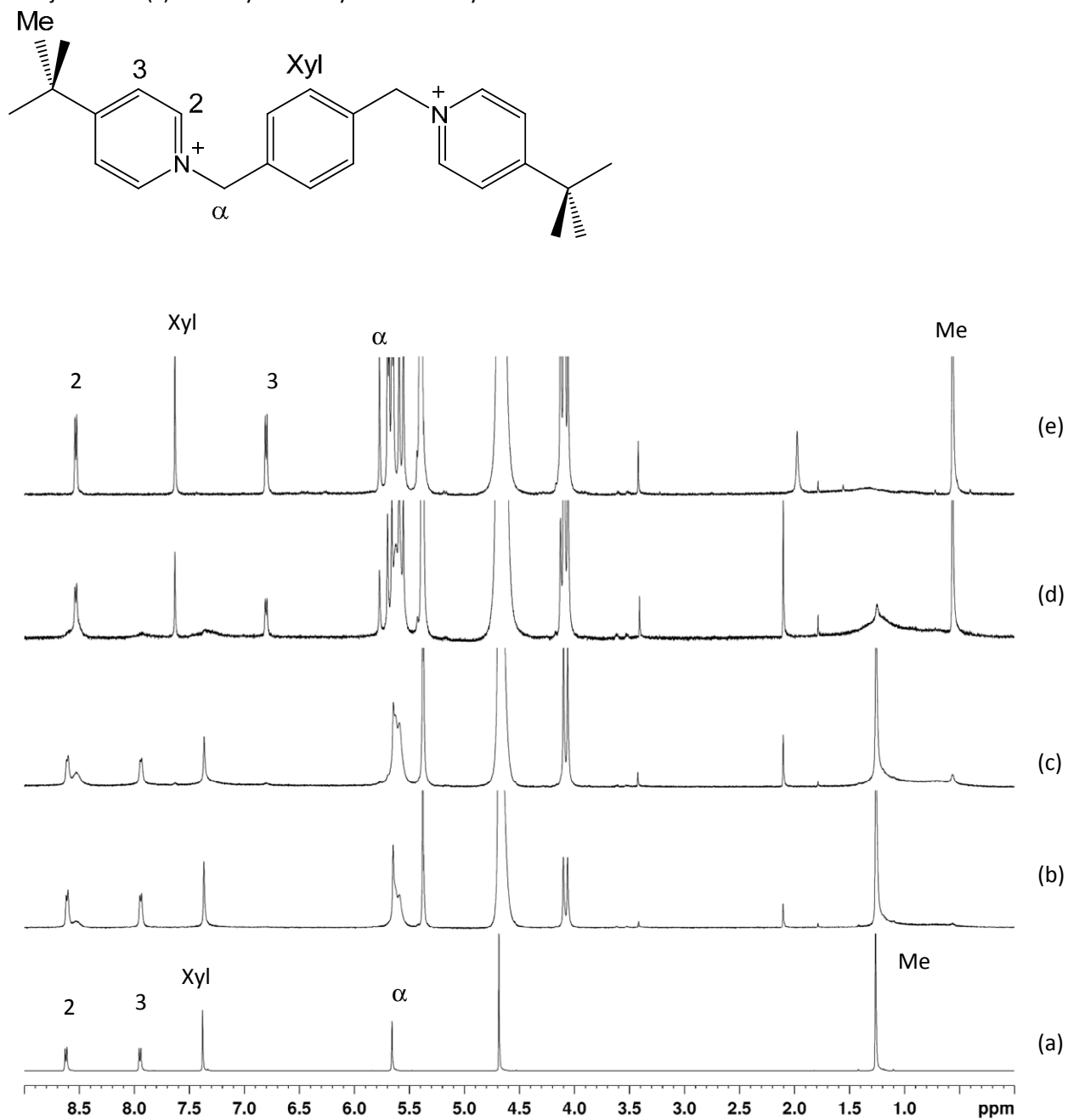
Figure S9. 1 H NMR spectra of BBPX 2+ ( 0.51 \times 10^{-3} \text{ mol dm}^{-3} ) in the presence of (a) 0.00 equiv, (b) 0.34 equiv, (c) 0.90 equiv, (d) 1.57 equiv, and (e) 2.48 equiv of CB[7] in D 2 O.
