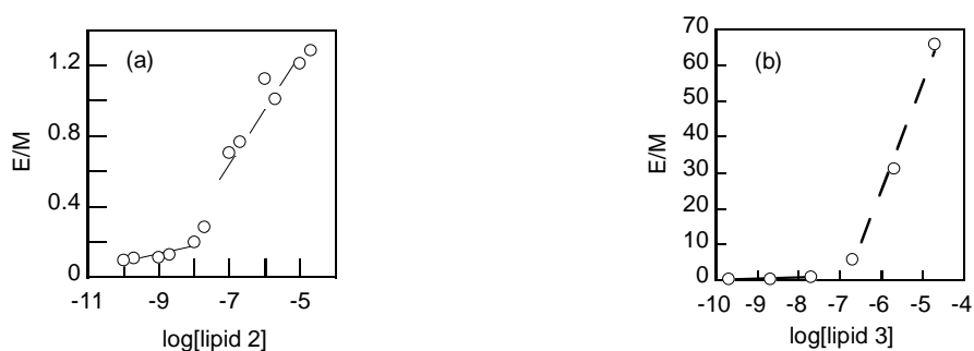
Fig S4. E/M of (a) lipid 2 and (b) lipid 3 vs. log[lipid] for critical aggregation concentration (CAC) determination. The intercept of the two linear fits corresponds to the CAC value.
