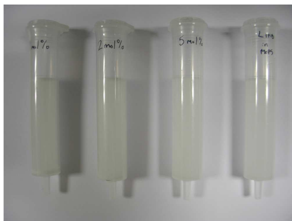
Fig S9. GPC columns after elution of lipid 3 with 10 ml buffer. From left to right; 1 % mol/mol, 2 % mol/mol and 5 % mol/mol in DMPC vesicles and as a micellar suspension in buffer.
