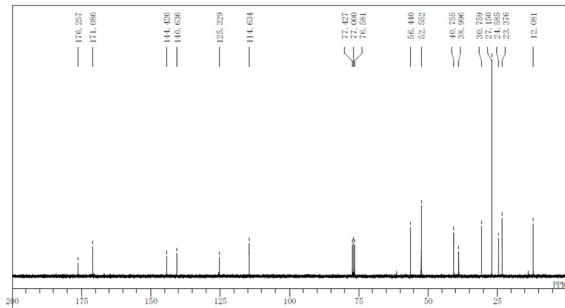
**3-[1-(2-Hydroxybenzoyloxy)ethylidene]-4-methylenecyclopentane-1,1-dicarboxylic dimethyl ester (3ag)**
