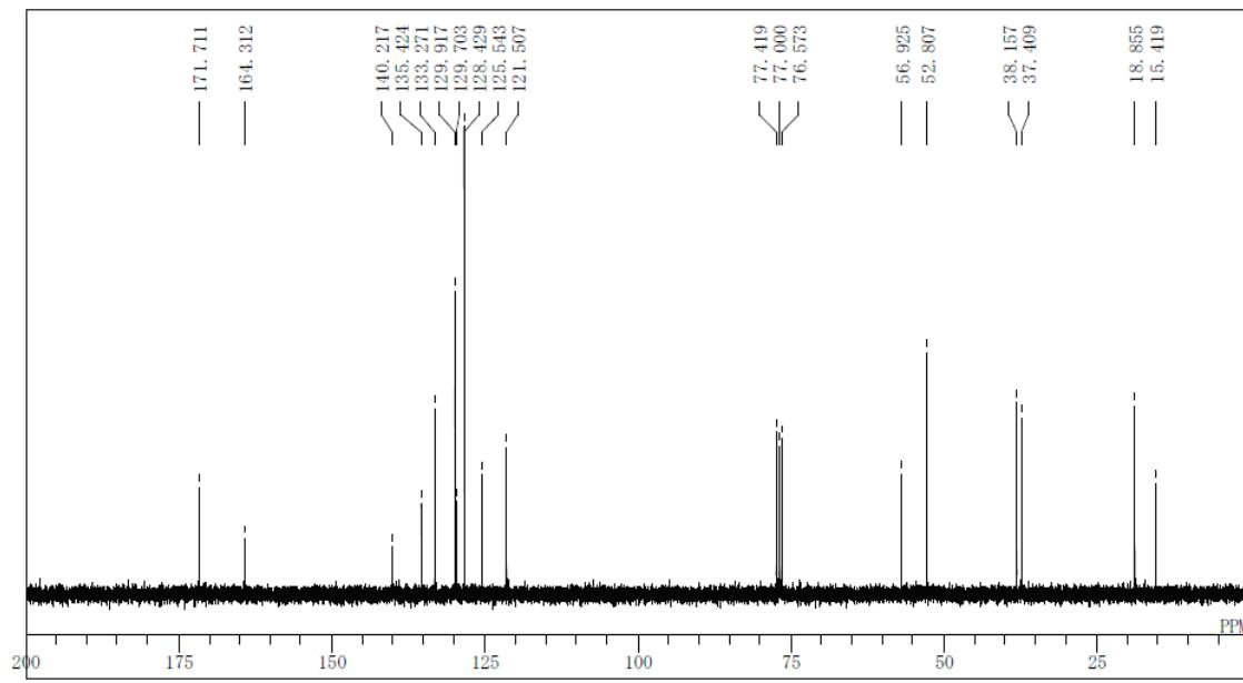
**4-[1-(2,2-Dimethylpropionyloxy)propylidene]-3-methylenecyclohexane-1,1-dicarboxylic acid dimethyl ester (3gd)**
