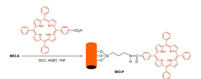
**BIO-P. BIO-A** was dried in vacuo at room temperature for 4 h. A mixture of **BIO-A** (300 mg), 5-(4-carboxyphenyl)-10,15,20-triphenylporphyrin (100 mg, 0.152 mmol), DCC (78.5 mg, 0.380 mmol), and HOBT (51 mg, 0.377 mmol) in dry THF (4 mL) under N<sub>2</sub> was stirred at room temperature for 72 h. The mixture was filtered and washed with THF, EtOH, hot EtOH, and then hexane. The resulting **BIO-P** was dried in vacuo. Elemental analysis
