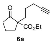
Following GP1 using ethyl 2-oxocyclopentanecarboxylate (403 mg, 2.58 mmol) **6a** was obtained as a colourless liquid (426 mg, 74%).  $\nu_{\max}$  /cm<sup>-1</sup> (neat) 3282,
