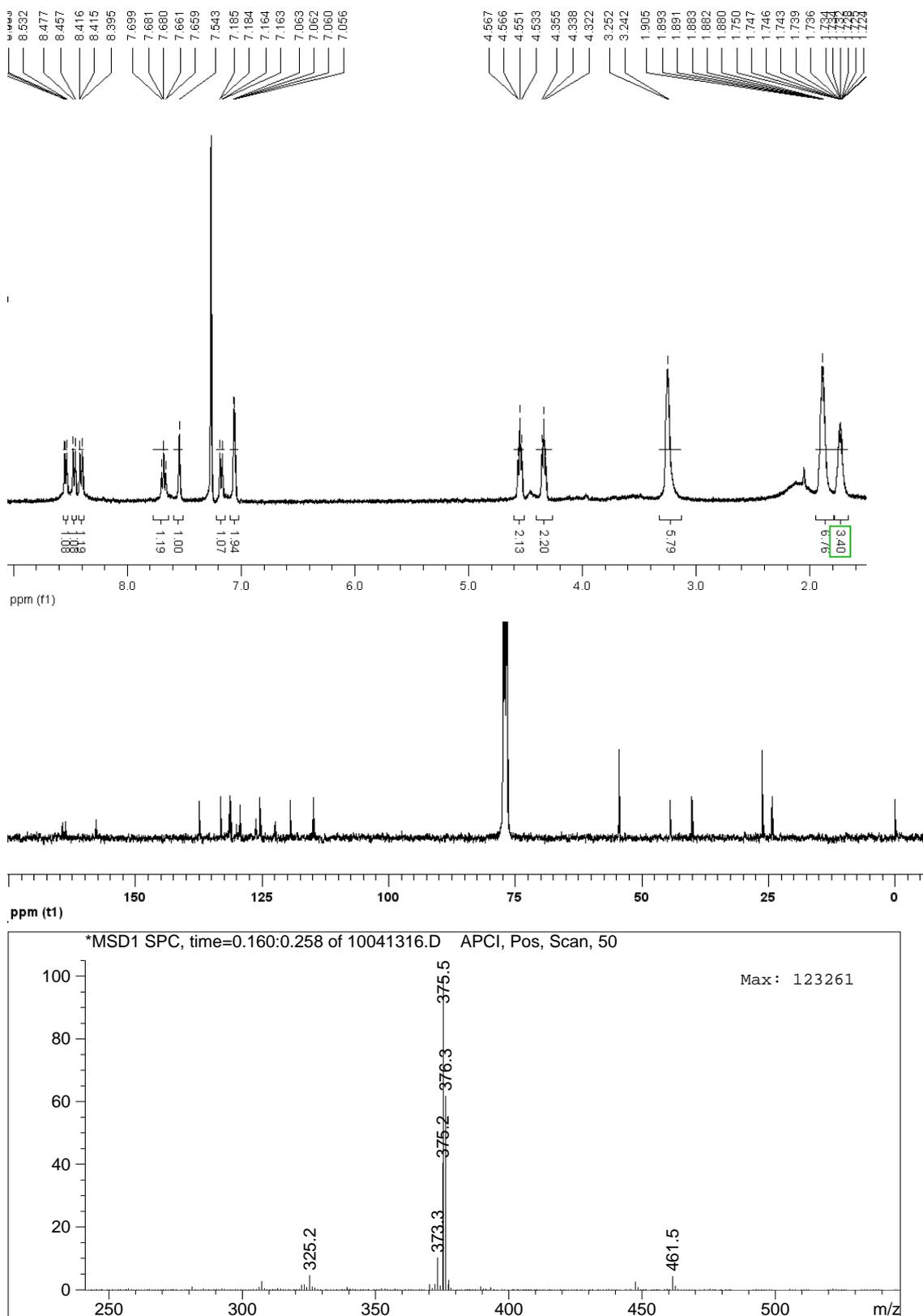
20. Figure S19.  $^1\text{H}$ -NMR (top picture),  $^{13}\text{C}$ -NMR (middle picture) and Mass (bottom picture) spectra of the 7.
