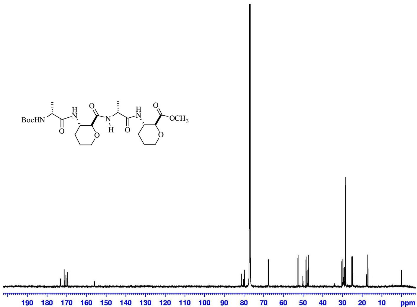
Supporting Figure 23. <sup>13</sup>C NMR spectrum of peptide 8 (150 MHz, CDCl<sub>3</sub>).
