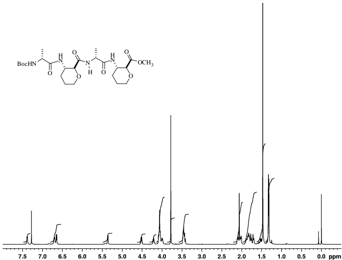
Supporting Figure 22. <sup>1</sup>H NMR spectrum of peptide 8 (600 MHz, CDCl<sub>3</sub>, 278 K).
