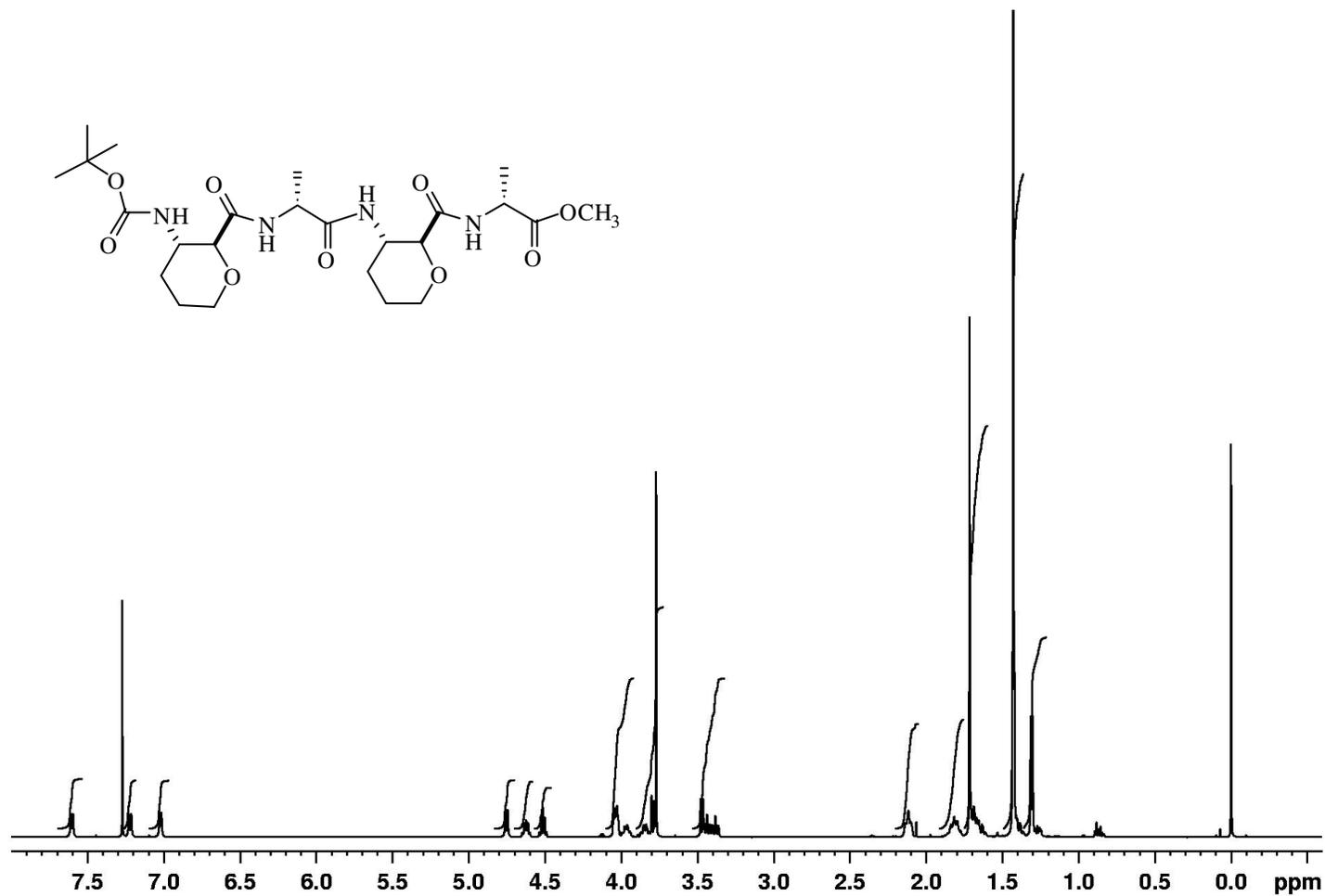
Supporting Figure 6. <sup>1</sup>H NMR spectrum of peptide 4 (600 MHz, CDCl<sub>3</sub>, 278 K)
