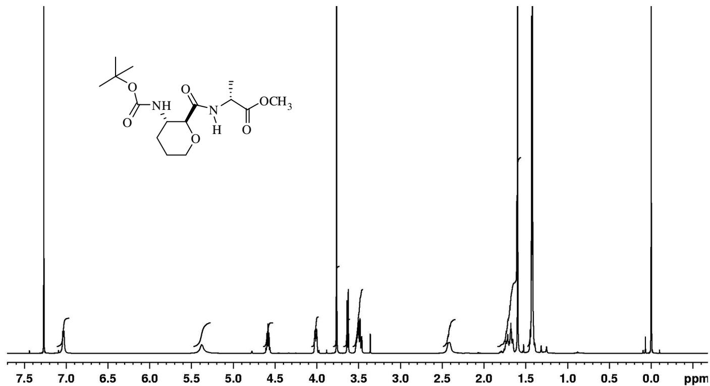
Supporting Figure 2. <sup>1</sup>H NMR spectrum of peptide 3 (600 MHz, CDCl<sub>3</sub>, 298 K).
