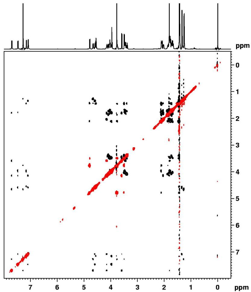
Supporting Figure 17. ROESY spectrum of peptide 6 (600 MHz, CDCl<sub>3</sub>, 278 K)
