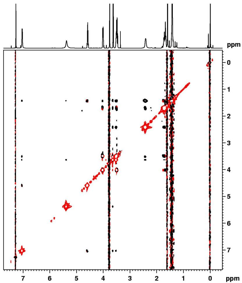
Supporting Figure 5. ROESY spectrum of peptide 3 (600 MHz, CDCl<sub>3</sub>, 298 K)
