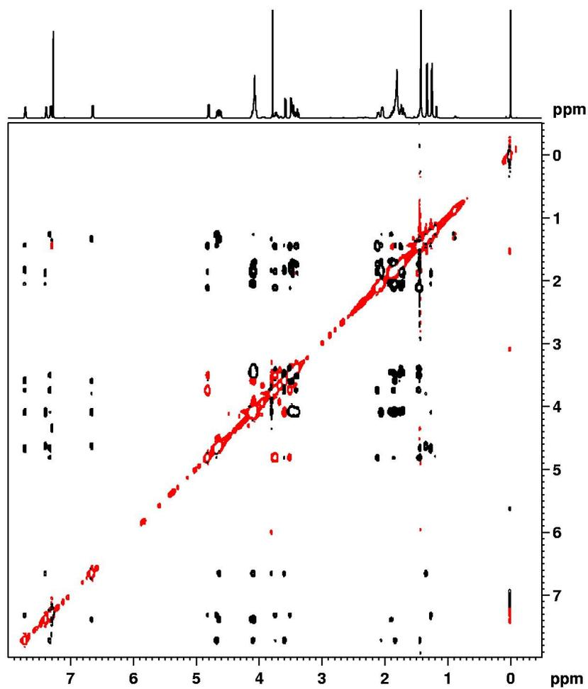
Supporting Figure 13. ROESY spectrum of peptide 5 (600 MHz, CDCl<sub>3</sub>, 288 K).
