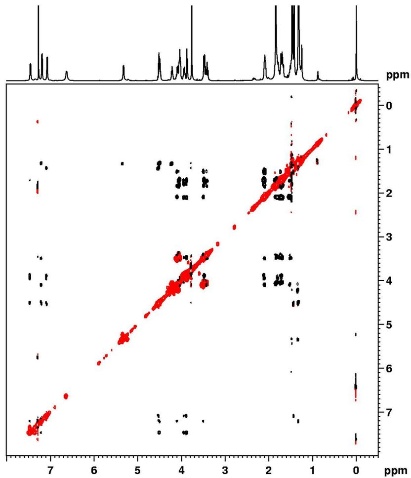
Supporting Figure 29. ROESY spectrum of peptide 9 (600 MHz, CDCl<sub>3</sub>, 278 K).
