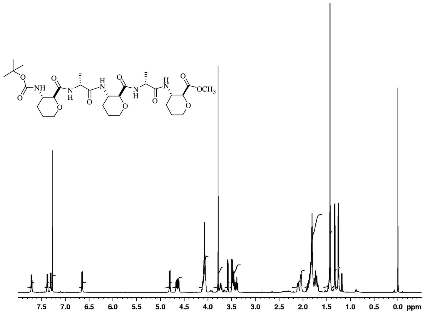
**Supporting Figure 10.** <sup>1</sup>H NMR spectrum of peptide 5 (600 MHz, CDCl<sub>3</sub>, 288 K).
