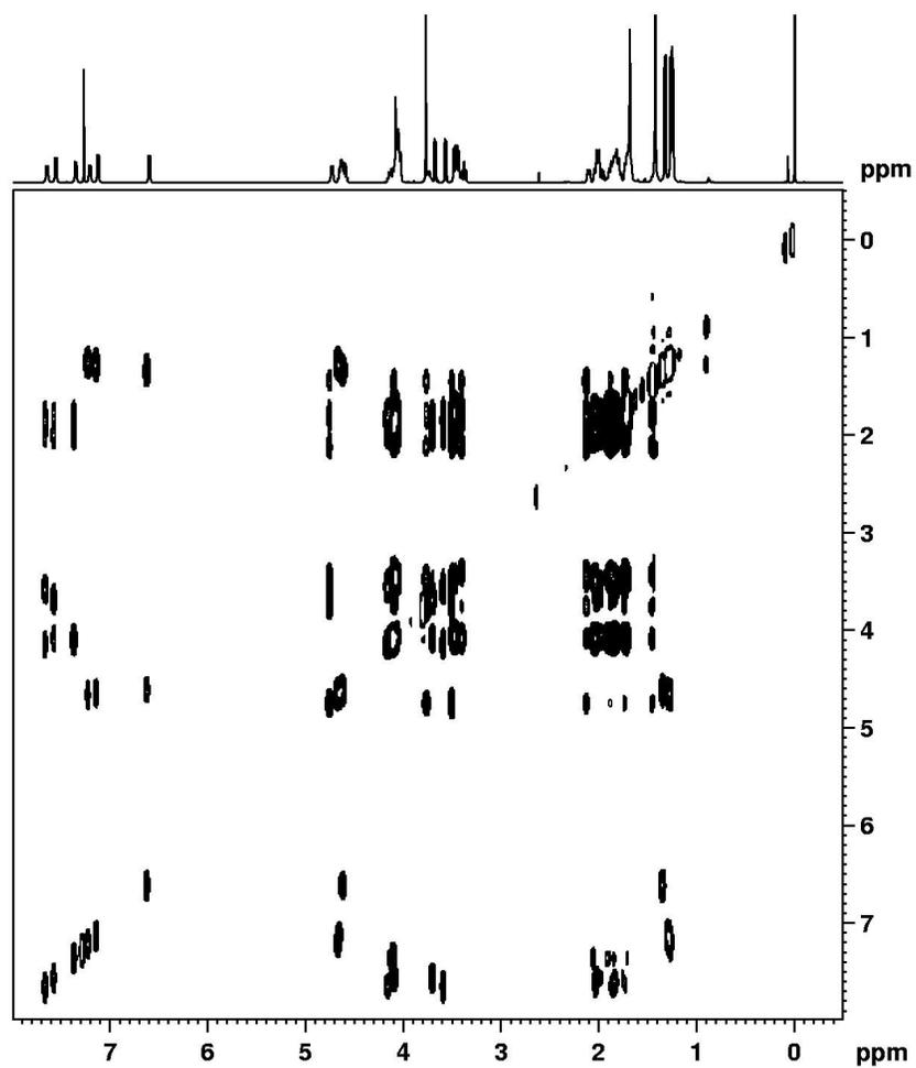
Supporting Figure 20. TOCSY spectrum of peptide 7 (600 MHz, CDCl<sub>3</sub>, 288 K).
