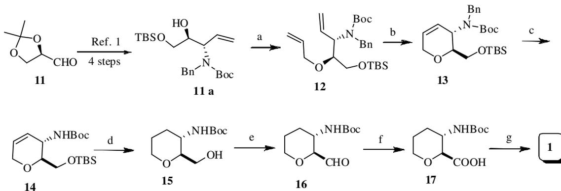
*Reagents and conditions:* a) Allyl bromide, NaH, DMF, 0 °C - rt, 4 h; b) Grubb's-I catalyst, Toluene, Reflux, 8 h; c) Li, Liq NH<sub>3</sub>, THF, -78 °C, 1 h; d) 10% Pd-C, MeOH, H<sub>2</sub>, 6 h; e) (COCl)<sub>2</sub>, DMSO, CH<sub>2</sub>Cl<sub>2</sub>, -78 °C; f) NaClO<sub>2</sub>, 30% H<sub>2</sub>O<sub>2</sub>, t-BuOH:H<sub>2</sub>O (7:3); g) CH<sub>2</sub>N<sub>2</sub>, ether, 1 h.
