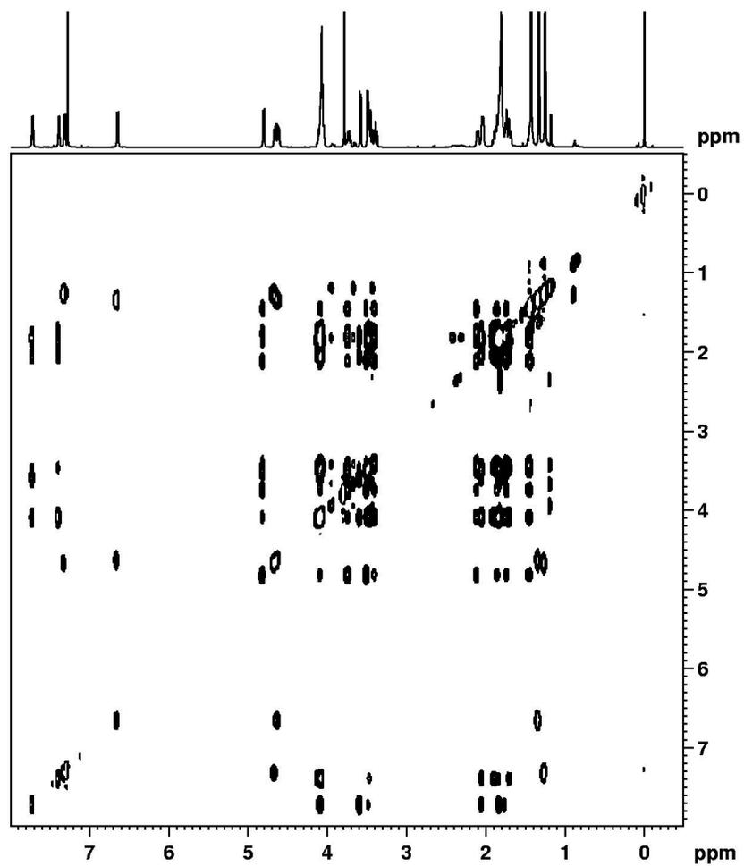
Supporting Figure 12. TOCSY spectrum of peptide 5 (600 MHz,  $\text{CDCl}_3$ , 288 K).
