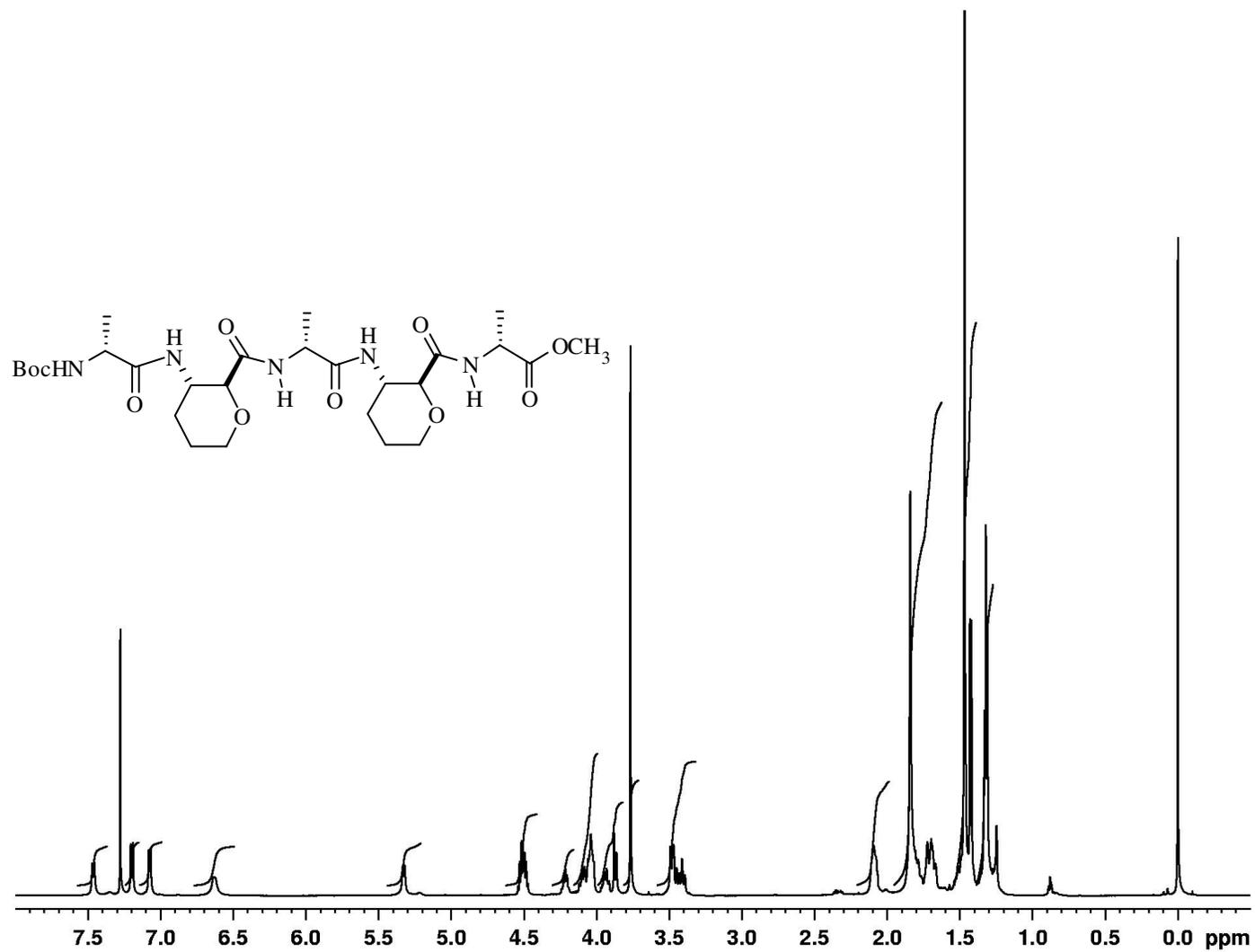
Supporting Figure 26. <sup>1</sup>H NMR spectrum of peptide 9 (600 MHz, CDCl<sub>3</sub>, 278 K).
