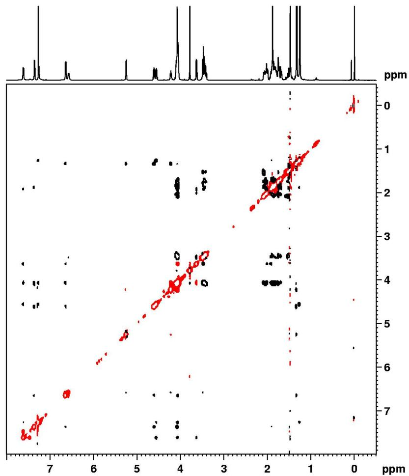
**Supporting Figure 34. ROESY spectrum of peptide 10 (600 MHz, CDCl<sub>3</sub>, 278 K).**
