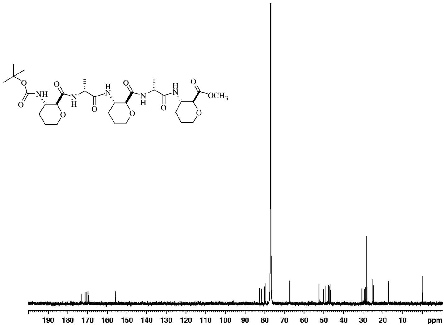
Supporting Figure 11. <sup>13</sup>C NMR spectrum of peptide 5 (150 MHz, CDCl<sub>3</sub>).
