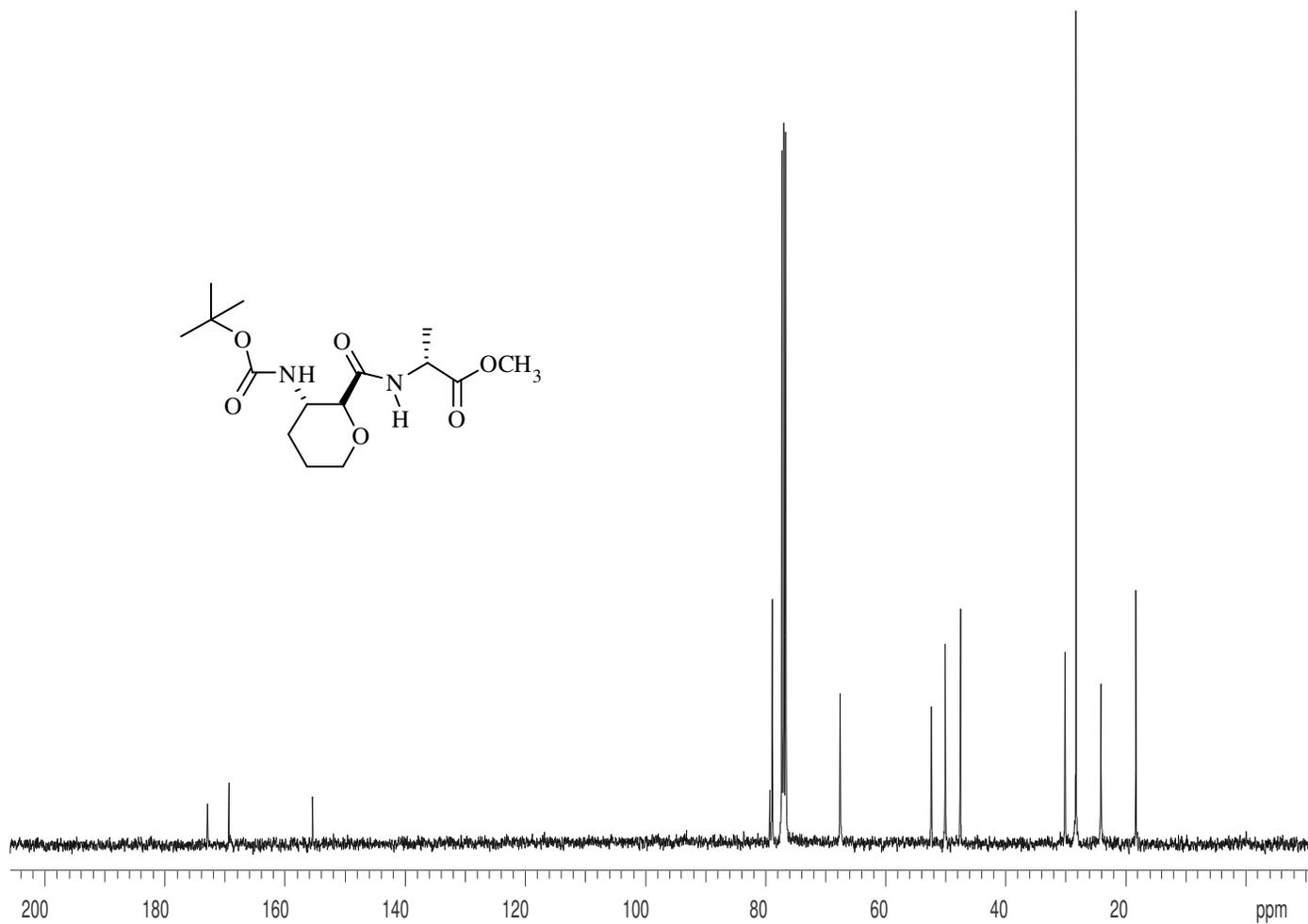
**Supporting Figure 3.** <sup>13</sup>C NMR spectrum of peptide 3 (100 MHz, CDCl<sub>3</sub>).
