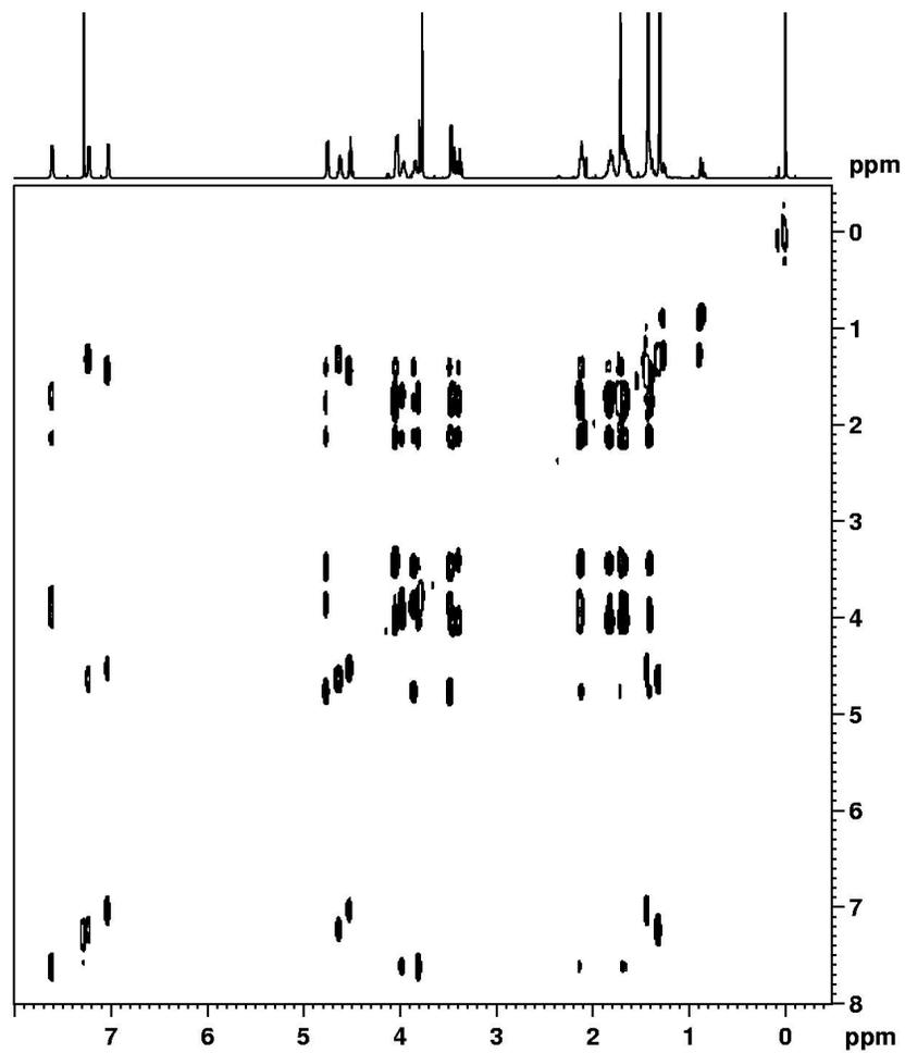
**Supporting Figure 8. TOCSY spectrum of peptide 4 (600 MHz, CDCl<sub>3</sub>, 278 K).**
