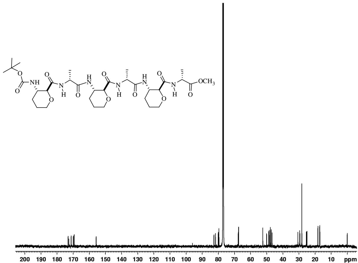
Supporting Figure 15. <sup>13</sup>C NMR spectrum of peptide 6 (150 MHz, CDCl<sub>3</sub>).
