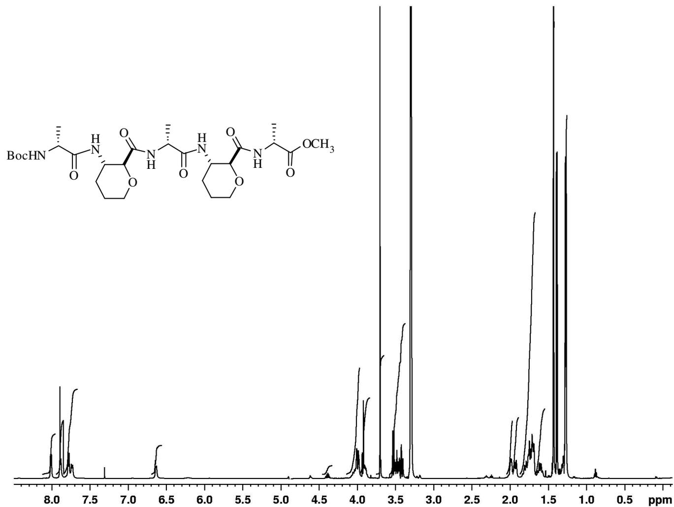
Supporting Figure 35. <sup>1</sup>H NMR spectrum of peptide 9 (600 MHz, CD<sub>3</sub>OH, 298 K).
