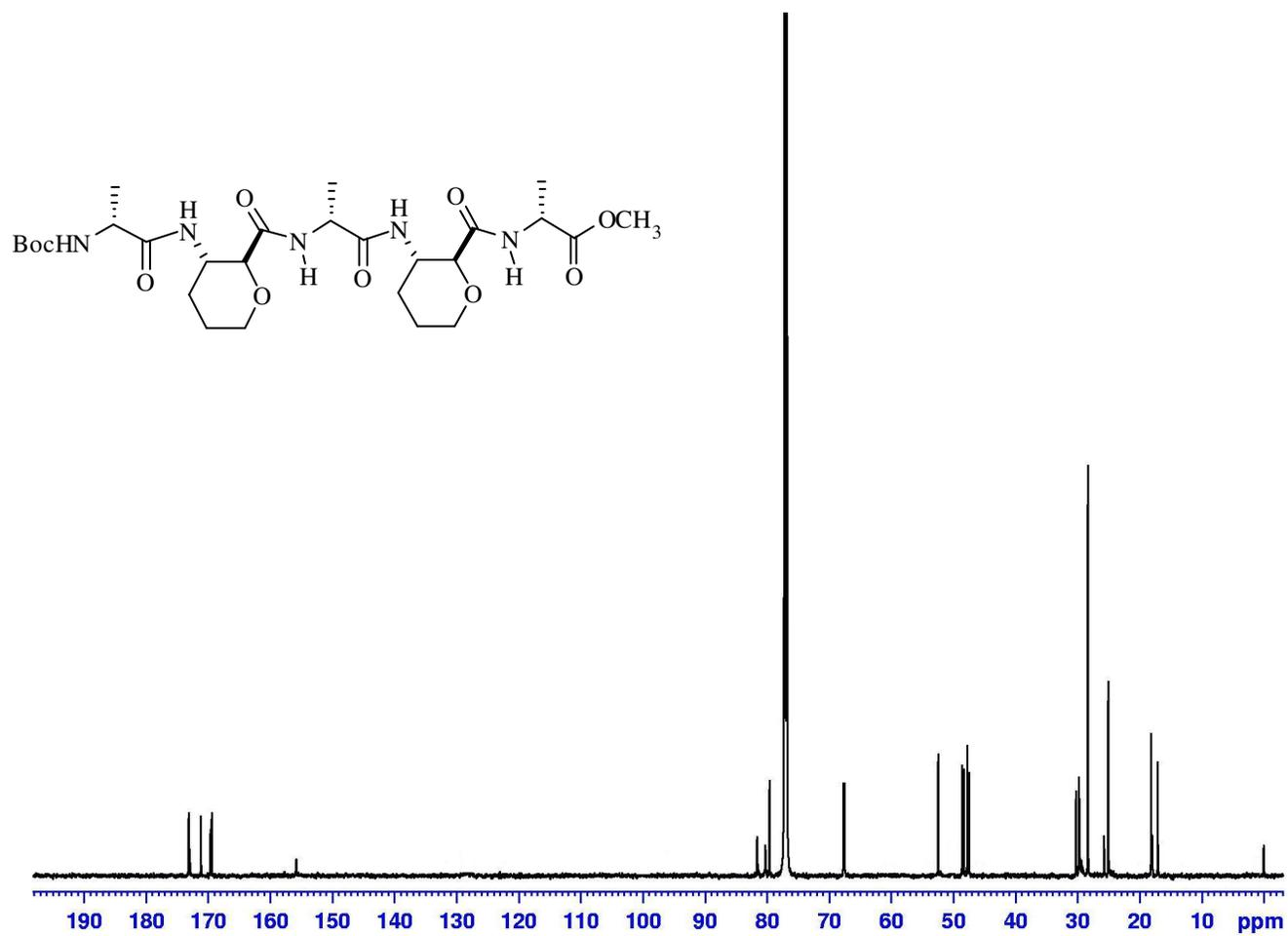
Supporting Figure 27. <sup>13</sup>C NMR spectrum of peptide 9 (150 MHz, CDCl<sub>3</sub>).
