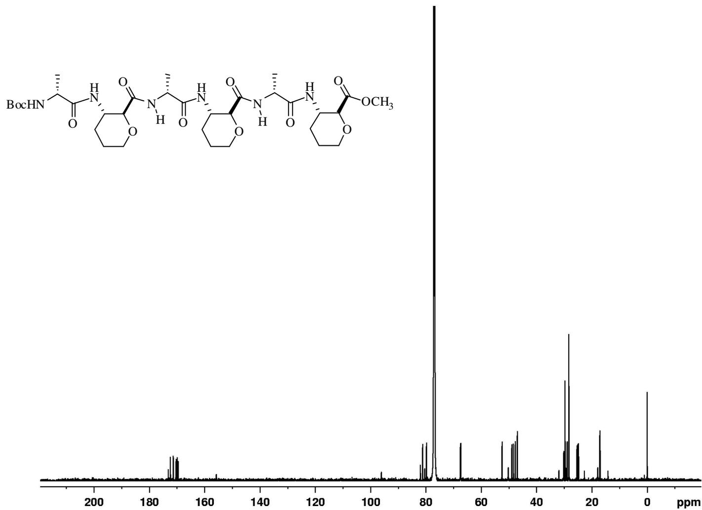
Supporting Figure 32. <sup>13</sup>C NMR spectrum of peptide 10 (150 MHz, CDCl<sub>3</sub>).
