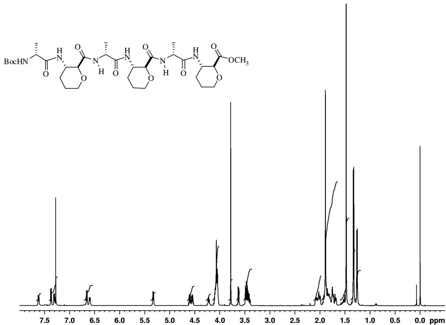
Supporting Figure 31. <sup>1</sup>H NMR spectrum of peptide 10 (600 MHz, CDCl<sub>3</sub>, 278 K).
