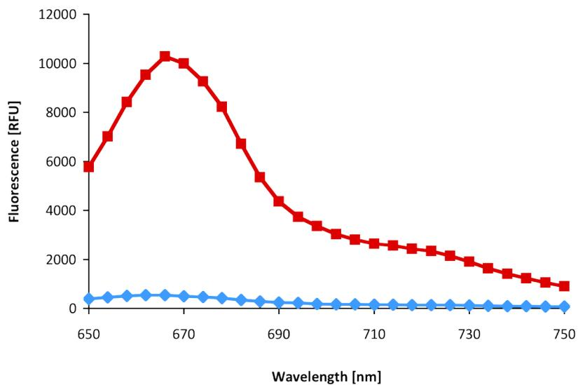
**Figure 7:** Fluorescence spectrum ( $\lambda_{\text{ex}}=600$  nm) of probe **5** (blue), **Cy5** (red), [30  $\mu\text{M}$ ] 20% DMSO in PBS buffer pH=8.3.
