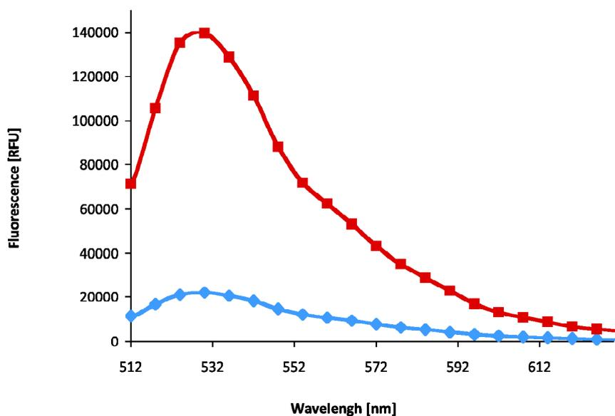
**Figure 6:** Fluorescence spectrum ( $\lambda_{\text{ex}}=490$  nm) of probe **4** (blue), mixture (1:1) of compound **4a** and **DR1** (red), [40  $\mu\text{M}$ ] in 12% DMSO in PBS buffer pH=7.2.
