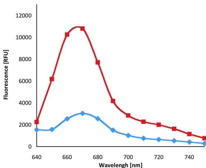
**Figure 5:** Fluorescence spectrum ( $\lambda_{\text{ex}}=640$  nm) of probe **2** (blue) [ $10 \mu\text{M}$ ], **Cy5** (red), [ $20 \mu\text{M}$ ] in PBS buffer pH=7.4.
