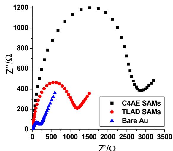
**Figure S3.** Impedance values ( $R_{ct}$ ) of 5.0 mM  $\text{Fe}(\text{CN})_6^{3/4-}$  in 0.10 M  $\text{KNO}_3$  aqueous solution on bare gold surface, TLAD SAMs and C4AE SAMs electrode with the frequency ranging from 100 KHz to 1.0 Hz , scan rate: 0.10 v/s, indicating that C4AE successfully modified on gold surface by clicking reaction in situ.
