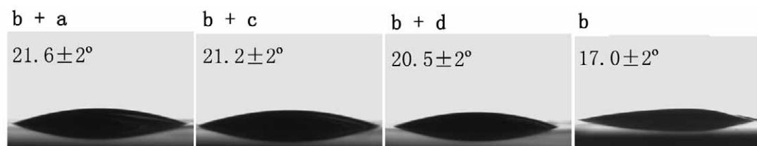
**Figure S5.** CA relationship images of C4AE SAMs responding to paraquat in presence and absence of solutions of compound **a**, **c** and **d**, respectively. The result of experiments indicates that the guests of **a**, **c** and **d** can not obviously affect contact angle of C4AE SAMs when it exposes into the solution of **b** compound.
