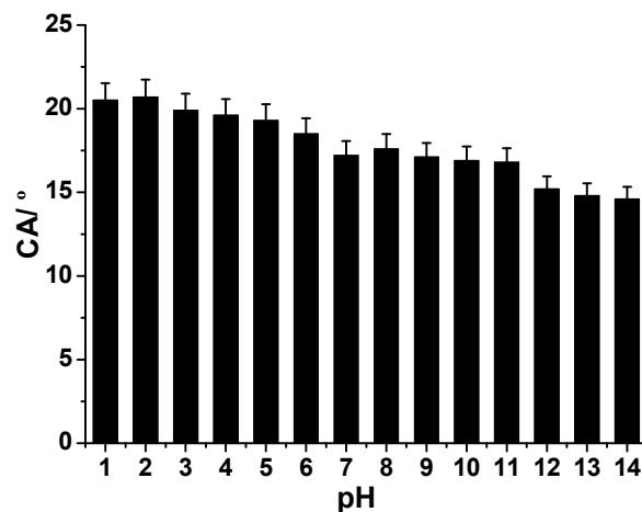
**Figure S6.** Contact angles which C4AE SAMs interacting with paraquat in different pH (1.0 – 14.0).
