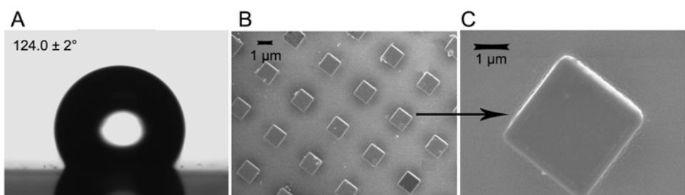
**Figure S2.** (A) Water-drop profiles on micro-nano gold surface (bare gold surface); (B) Scanning electron microscope image (SEM) of the micro-nano surface; (C) The detail morphology in B.
