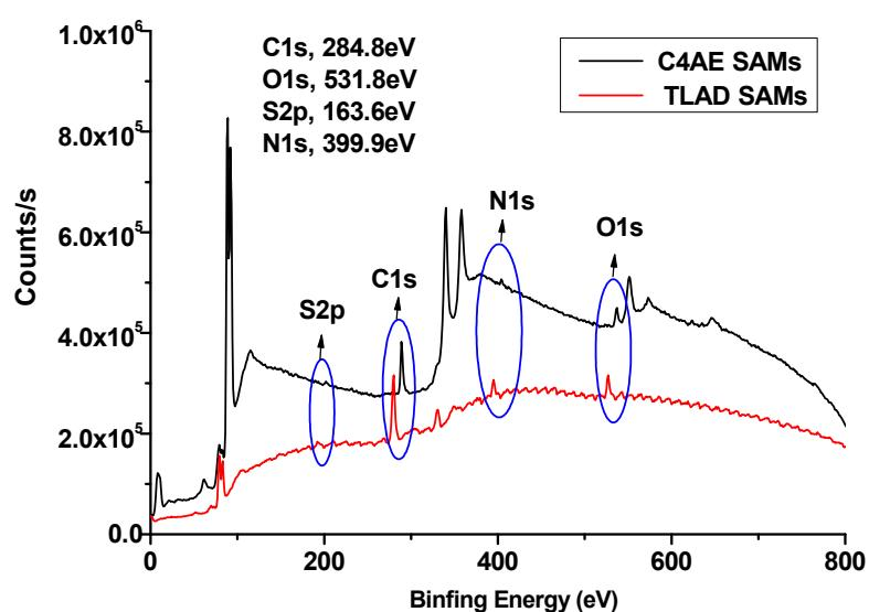
**Figure S1.** X-ray photoelectron spectroscopy (XPS) of C4AE and TLAD modified on surface.
