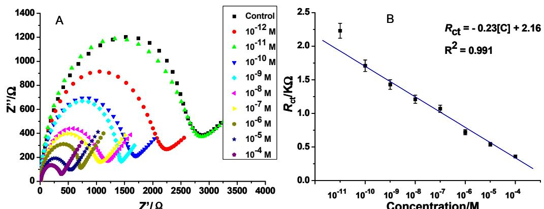
**Figure S4.** A) Impedance spectroscopy of  $\text{Fe}(\text{CN})_6^{3-/4-}$  as redox probe in the presence of increasing concentrations of paraquat ( $1.0 \times 10^{-12} - 1.0 \times 10^{-4} \text{ M}$ ); B) a plot of the  $R_{ct}$  versus concentrations of paraquat ( $1.0 \times 10^{-11} - 1.0 \times 10^{-4} \text{ M}$ ), indicating that  $R_{ct}$  value is good linear relationship with the increasing concentration of paraquat.
