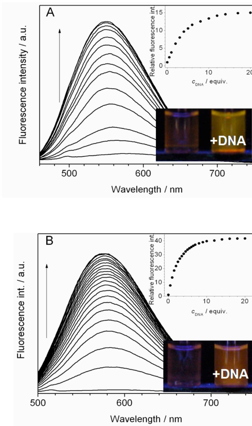
**Fig. S2 (Fig. 6A and 6B in main manuscript)** Spectrofluorimetric titrations of **2a** (A,  $\lambda_{\text{ex}} = 425$  nm), **2b** (B,  $\lambda_{\text{ex}} = 438$  nm) with ct DNA in BPE buffer ( $c = 10 \mu\text{M}$ ). The arrows indicate the changes of the bands upon addition of ct DNA. Insets: plot of the relative emission intensity versus  $c_{\text{DNA}}$ , and picture of the emission color of **2a** and **2b** in the absence and in the presence of ct DNA.
