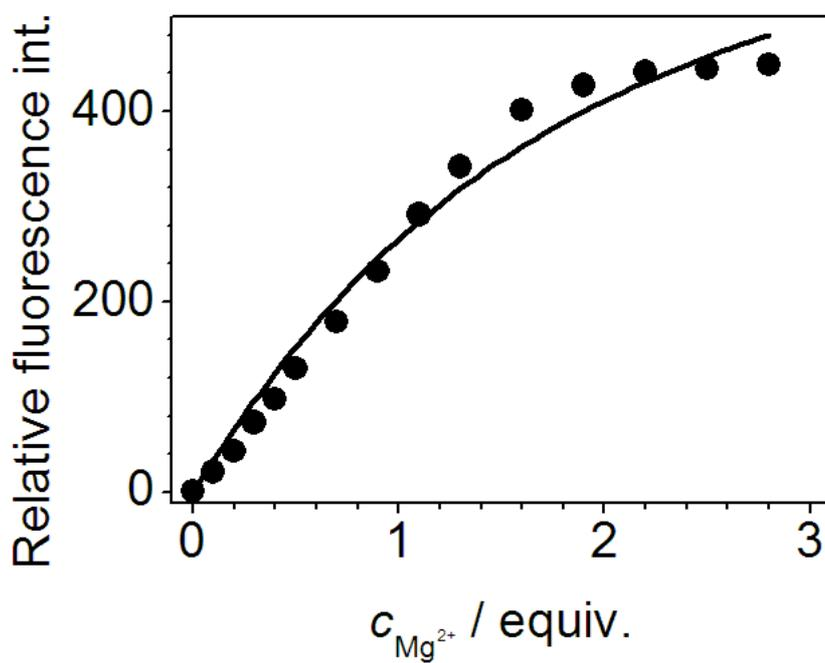
**Fig. S3** Spectrofluorimetric titration of Mg<sup>2+</sup> to compound **2a** ( $c = 10 \mu\text{M}$ ,  $\lambda_{\text{ex}} = 395 \text{ nm}$ ) in MeCN; plot of the emission intensity versus Mg<sup>2+</sup> concentration and fit of the experimental data to the theoretical model; numerical fit calculated for  $K = 0.9 \times 10^5 \text{ M}^{-1}$ .
