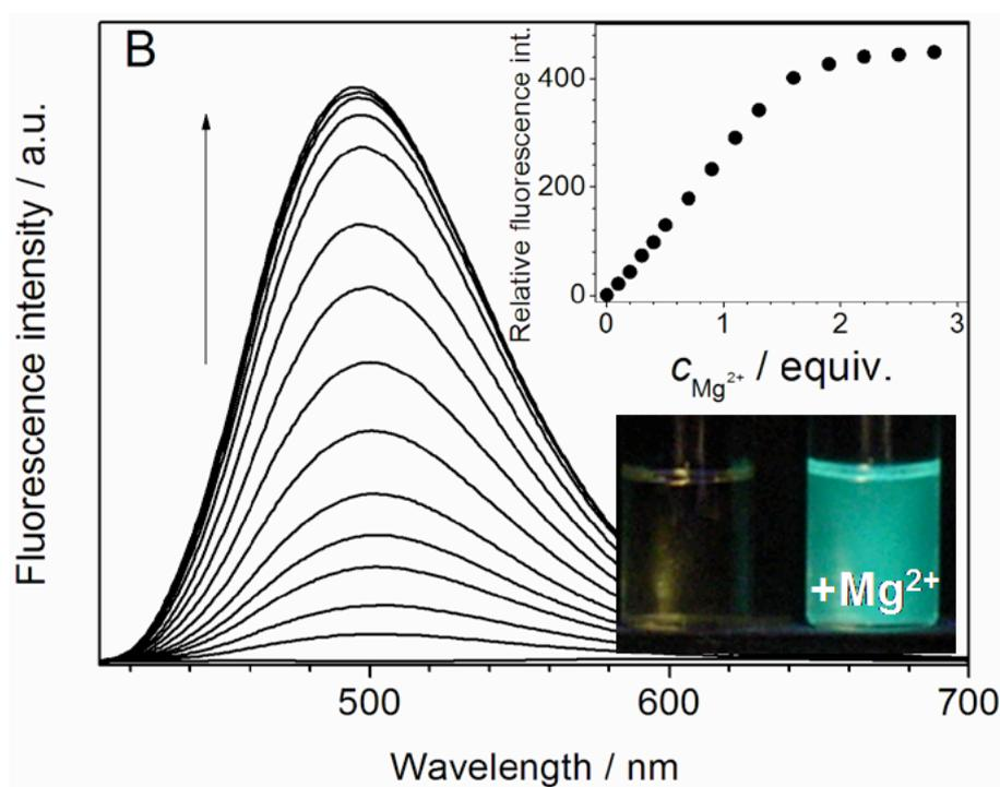
**Fig. S1 (Fig. 3B in main manuscript)** Spectrofluorimetric titration of  $Mg^{2+}$  to compound **2a** ( $c = 10 \mu M$ ,  $\lambda_{ex} = 395 \text{ nm}$ ) in MeCN. The arrows indicate the changes of emission upon addition of  $Mg^{2+}$ . Insets: Plot of the emission intensity at 495 nm versus  $Mg^{2+}$  concentration, and picture of the emission color of **2a** in the absence and in the presence of  $Mg^{2+}$ .
