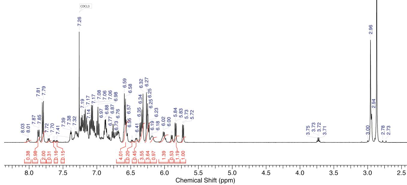
Fig. S4 <sup>1</sup>H NMR spectrum (500 MHz, 0 °C, CDCl<sub>3</sub>) of oP(DA)<sup>6</sup>.
