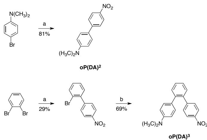
**Scheme S1** Reagents and conditions: (a) 4-nitrophenoxyboronic acid pinacol ester, Pd(PPh<sub>3</sub>)<sub>4</sub>, Na<sub>2</sub>CO<sub>3</sub>(aq), toluene, EtOH; (b) 4-dimethylaminophenoxyboronic acid, Pd(OAc)<sub>2</sub>, SPhos, K<sub>3</sub>PO<sub>4</sub>, THF, water.
