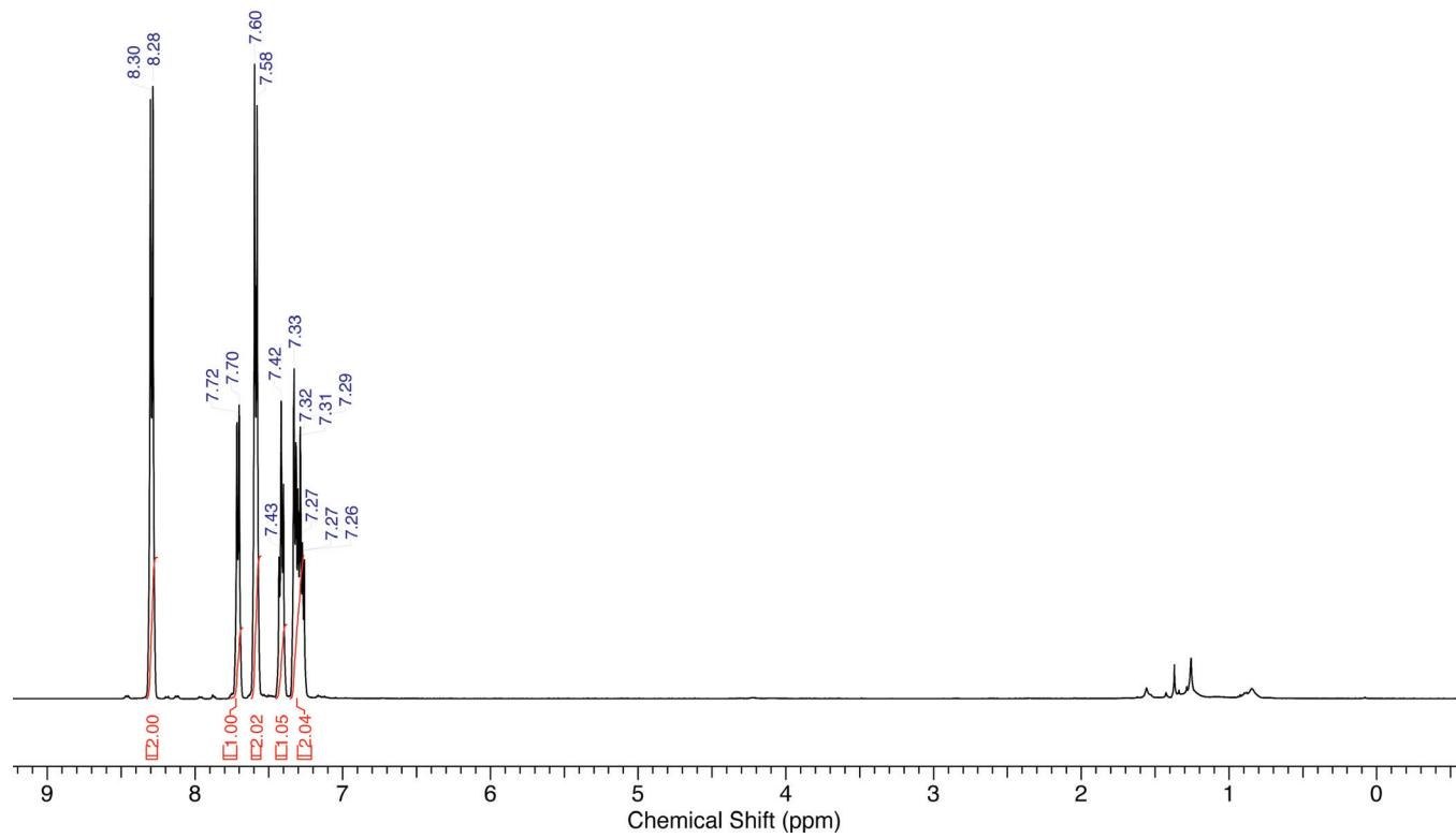
Fig. S22 <sup>1</sup>H NMR spectrum (500 MHz, CDCl<sub>3</sub>) of 2-bromo-4'-nitrobiphenyl.
