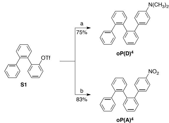
**Scheme S2** Reagents and conditions: (a) 4-dimethylaminophenylboronic acid, Pd(OAc)<sub>2</sub>, SPhos, K<sub>3</sub>PO<sub>4</sub>, THF, water; (b) 4-nitrophenylboronic acid, Pd(OAc)<sub>2</sub>, SPhos, K<sub>3</sub>PO<sub>4</sub>, THF, water.
