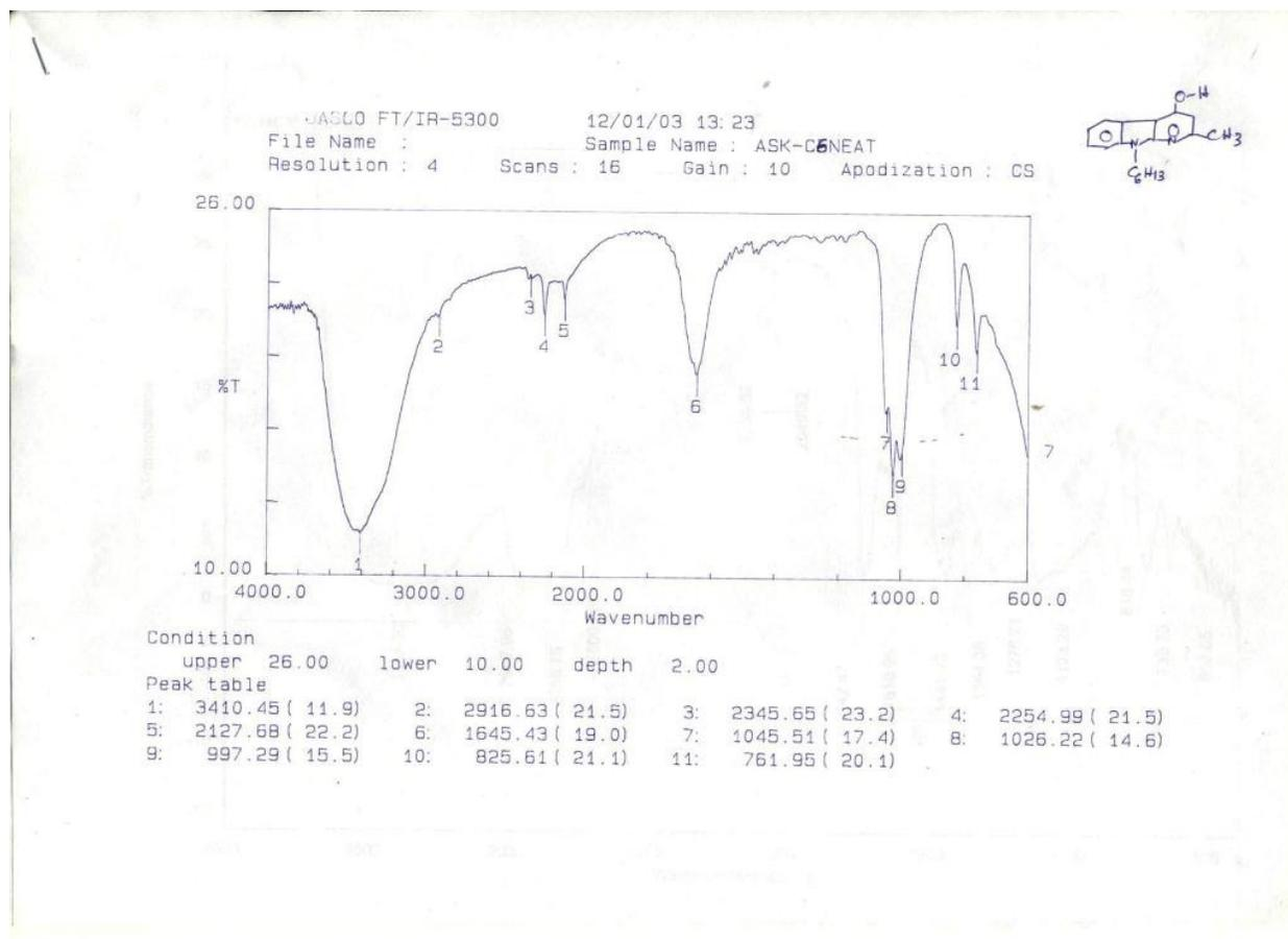
**Figure S4.** IR Spectrum of **2f**
