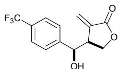
Following procedure A, using 4-trifluoromethylbenzaldehyde (170mg, 0.98mmol), afforded the above alcohol 2e (242mg, 91%) via column chromatography (petroleum ether/ethyl acetate, 1:1).
