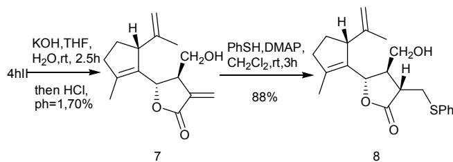
Synthesis of 4-Hydroxymethyl-5-(5-isopropenyl-2-methyl-1-en-cyclopentyl)-3-methylenedihydrofuran-2(3H)-one (5,7)
