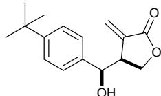
Following procedure A, using 4-tert-butylbenzaldehyde (161mg, 0.99mmol), afforded the above alcohol 2f (233mg, 90%) via column chromatography (petroleum ether/ethyl acetate, 1:1).
