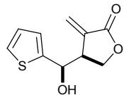
Following procedure A, using 2-thiophenaldehyde (115mg, 1.03mmol), afforded the above alcohol 2j (184mg, 85%) via column chromatography (petroleum ether/ethyl acetate, 1:1).
