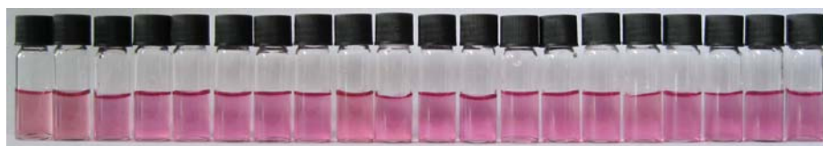
Color changes of sensor 2·Zn (50 \mu M) in 50 mM aqueous HEPES buffer solution (pH 7.4). Anions (1 mM) from left to right: none, PPI, AMP, ADP, ATP, \text{PO}_4^{3-} , \text{HPO}_4^{2-} , PhPi, \text{F}^- , \text{Cl}^- , \text{Br}^- , \text{I}^- , \text{NO}_3^- , \text{SO}_4^{2-} , \text{HCO}_3^- , \text{CH}_3\text{CO}_2^- , Citrate, \text{N}_3^- , \text{S}_2\text{O}_7^{2-} , \text{ClO}_4^- .
