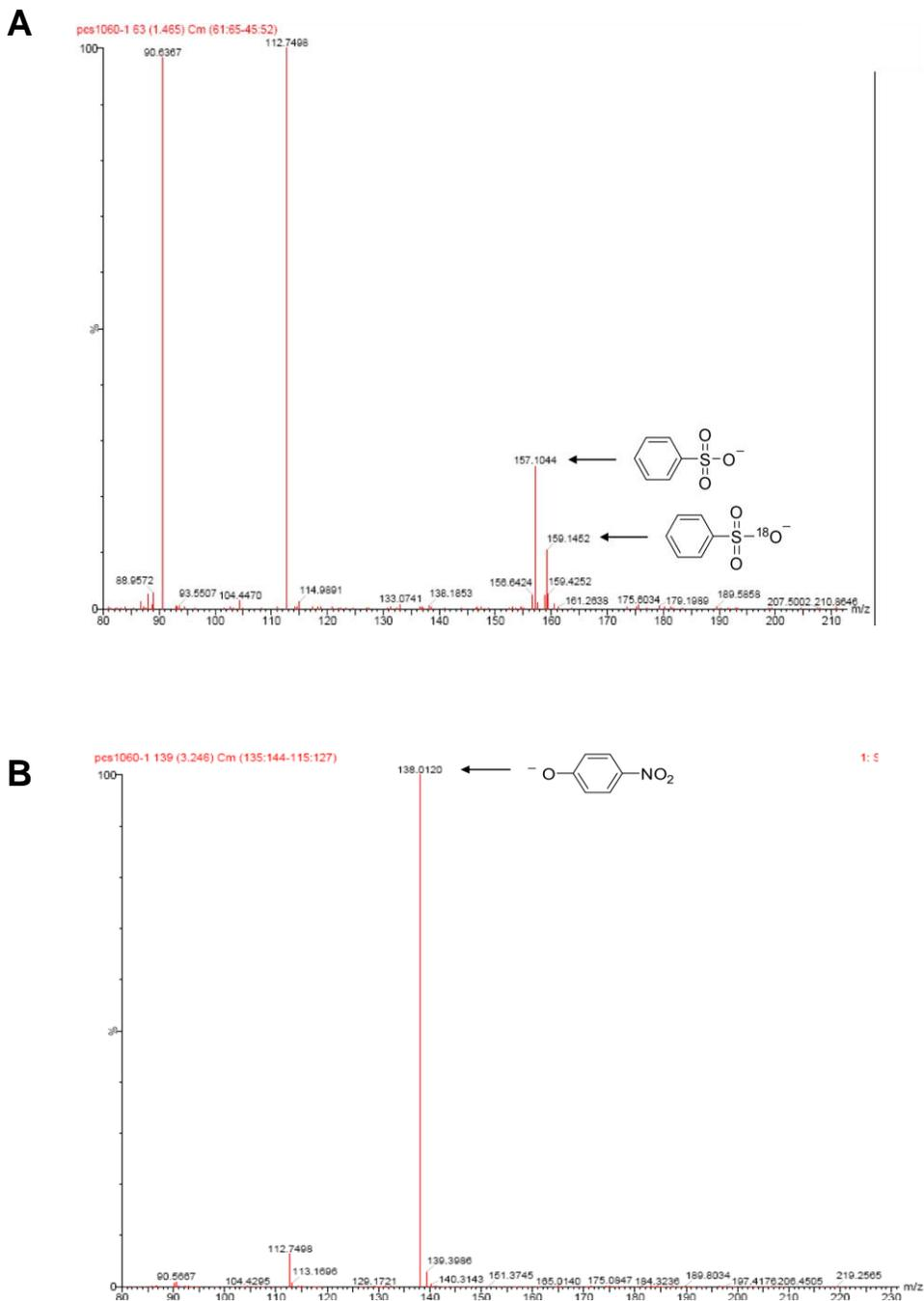
**Figure S2:** LC-MS of products of 4-nitrophenyl benzene sulfonate hydrolysis in the presence of 38 %  $\text{H}_2^{18}\text{O}$ .  $^{18}\text{O}$  was only detected in the  $\text{PhSO}_3^-$  product (A); the  $(\text{O}_2\text{N})\text{C}_6\text{H}_4\text{O}^-$  product was unlabelled (B).
