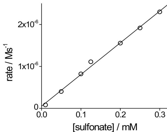
**Figure S3.** Kinetic plots for the hydrolysis of 4-nitrophenyl benzenesulfonate **1**. (A) The pH-rate profile of the hydrolysis of **1** is linear ( $r = 0.99$ ), establishing first order kinetics with respect to the hydroxide nucleophile. *Conditions:* 0.01-0.12 M KOH;  $T = 50^\circ\text{C}$ ; 0.25 mM sulfonate (B) The initial rate correlates linearly to sulfonate ester concentration. *Conditions:* 0.1 M KOH;  $T = 50^\circ\text{C}$ ; 0.01-0.3 mM sulfonate.
