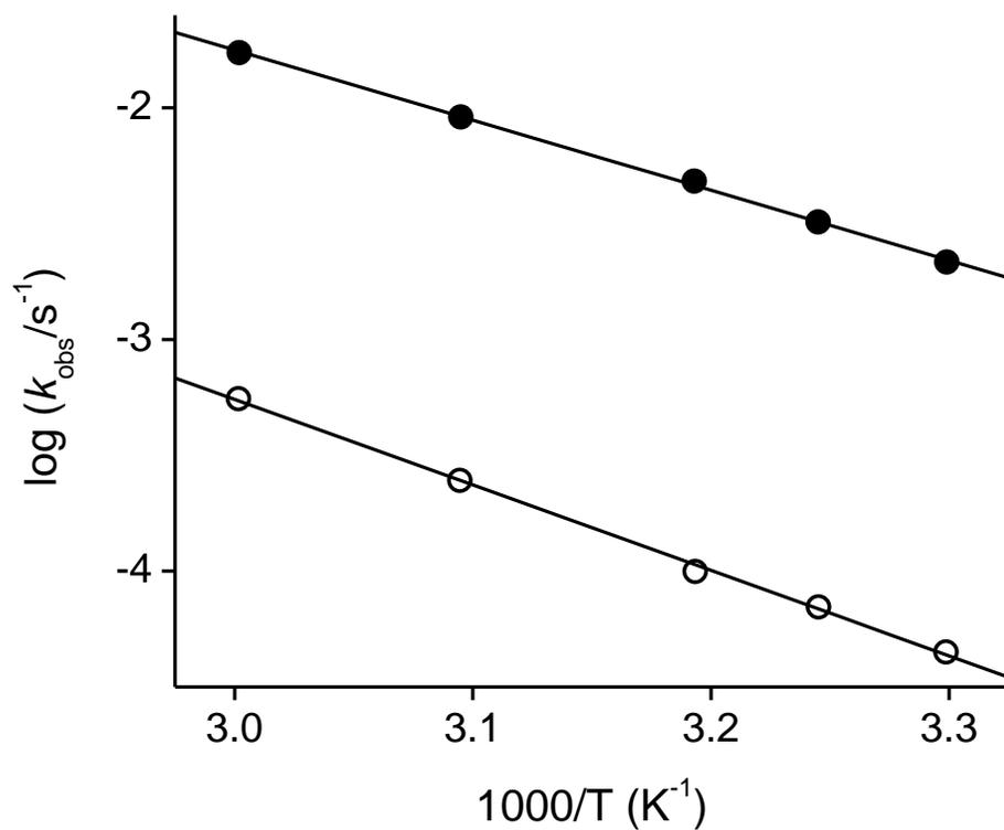
**Figure S4:** Arrhenius plots for the alkaline hydrolysis of phenyl- and *p*-nitrophenyl benzenesulfonates. Phenyl benzenesulfonate (open circles; gradient =  $-3.7 \pm 0.1$ , y-intercept =  $7.8 \pm 0.3$ ), 4-nitrophenyl benzenesulfonate (filled circles; gradient =  $-3.0 \pm 0.1$ , y-intercept =  $7.3 \pm 0.2$ ). *Conditions:* 0.1 M KOH;  $T = 30\text{--}60$  °C.
