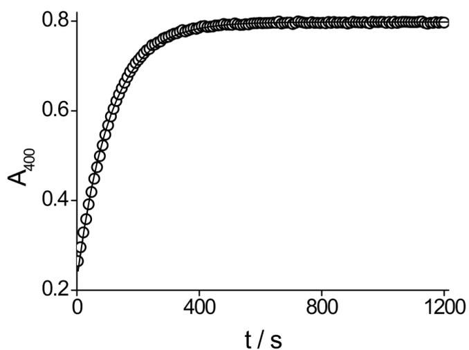
**Figure S1.** Kinetics of the reaction of 4-nitrophenyl benzenesulfonate **1**. (A) A typical progress curve ( $[4\text{-nitrophenyl benzenesulfonate}] = 0.04 \text{ mM}$ ,  $T = 50^\circ\text{C}$ ,  $0.1 \text{ M KOH}$ ). Pseudo-first order rate constants  $k_{\text{obs}}$  were obtained from exponential fits of progress curves (using  $A_t = A_\infty - (A_\infty - A_0)e^{-kt}$ )
