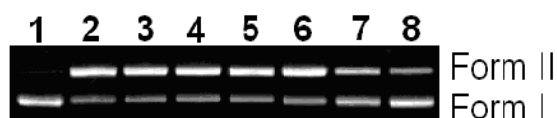
Figure S8. Agarose gel (1%) of pUC 19 DNA (0.05 mM bp) cleavage promoted by 0.05 mM 1 (incubated for 10 h at 37 °C in pH 7.25 (50 mM Tris-HCl)). Lane 1, DNA control; Lane 2, DNA + 1 ; Lane 3, DNA + 1 + 0.05 mM adenosine; Lane 4, DNA + 1 + 0.05 mM uridine; Lane 5, DNA + 1 + 0.05 mM guanosine; Lane 6, DNA + 1 + 0.05 mM cytidine; Lane 7, DNA + 1 + 0.10 mM BDNPP; Lane 8, DNA + 1 + 0.20 mM BDNPP.
