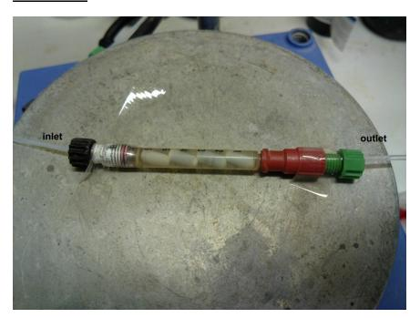
Body of mixer is cut from the barrel of a 1 mL HSW normject syringe. The thread on the inlet side was made by heating to softness then screwing in the  $\frac{1}{4}$ -28-UNF connector, which cut a thread. PTFE tape was used to improve the seal. The outlet is a simple female luer to female  $\frac{1}{4}$ -28 UNF adapter.
