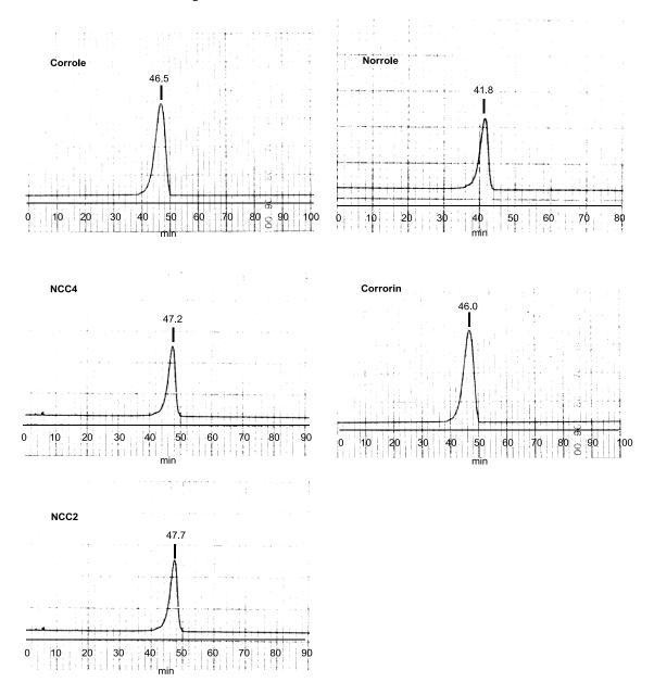
HPLC experiments were performed on a LC-9201R unit composed of a PI-50 pump 3702 UV-detector and JAIGEL-SH-043-15 column filled with silica gel (Japan Analytical Industry Co., Ltd). Eluent was  $CH_2Cl_2/CH_3OH = 99/1$ , and flow rate was 3.5 ml/min for all experiments.
