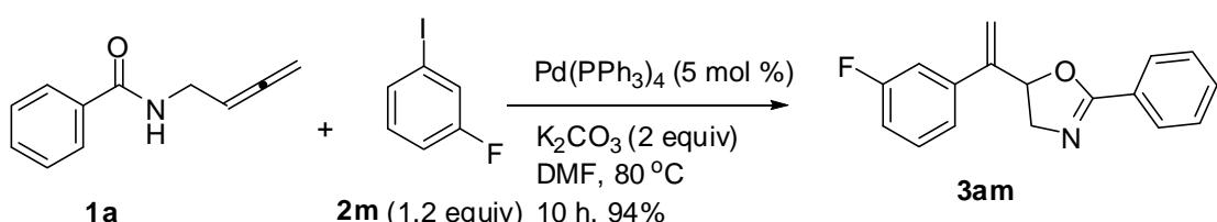
The reaction of  $\text{K}_2\text{CO}_3$  (55.4 mg, 0.4 mmol),  $\text{Pd}(\text{PPh}_3)_4$  (12.5 mg, 0.01 mmol), **1a** (34.9 mg, 0.2 mmol), **2m** (56.8 mg, 0.24 mmol), and DMF (2 mL) afforded **3am**
