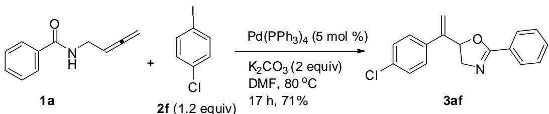
The reaction of  $\text{K}_2\text{CO}_3$  (55.6 mg, 0.4 mmol),  $\text{Pd}(\text{PPh}_3)_4$  (11.7 mg, 0.01 mmol), **1a** (36.1 mg, 0.2 mmol), **2f** (57.1 mg, 0.24 mmol), and DMF (2 mL) afforded **3af**
