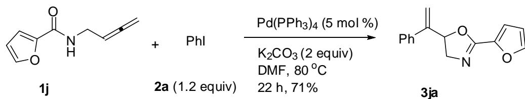
The reaction of K<sub>2</sub>CO<sub>3</sub> (56.2 mg, 0.4 mmol), Pd(PPh<sub>3</sub>)<sub>4</sub> (12.2 mg, 0.01 mmol),
