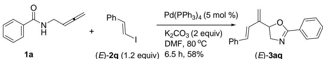
The reaction of  $\text{K}_2\text{CO}_3$  (55.5 mg, 0.4 mmol),  $\text{Pd}(\text{PPh}_3)_4$  (11.6 mg, 0.01 mmol), **1a**
