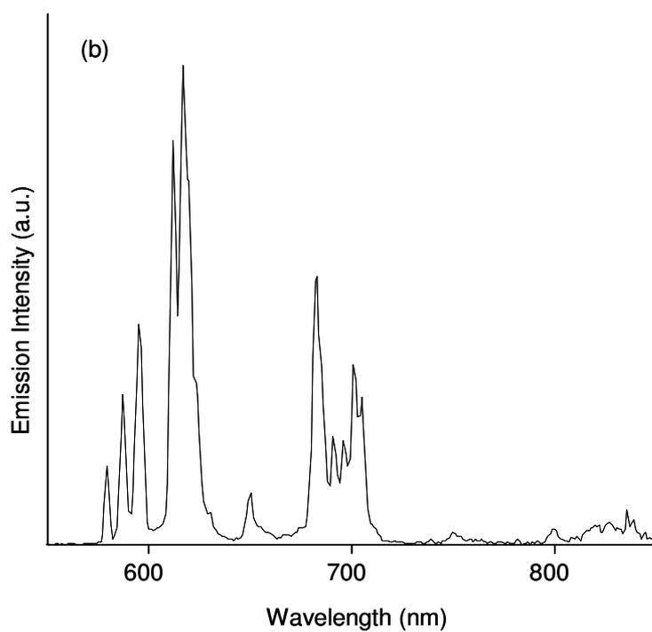
(a) excitation ( $\lambda_{em} = 617 \text{ nm}$ ) and (b) corrected emission ( $\lambda_{exc} = 350 \text{ nm}$ ) spectra of **10-GSS11** conjugate in phosphate buffered saline (100 mM with 0.1% BSA; pH 7) at 298 K. Excitation and emission band passes 20-2.5 nm respectively; delay time 0.1 ms, gate time 0.4 ms.
