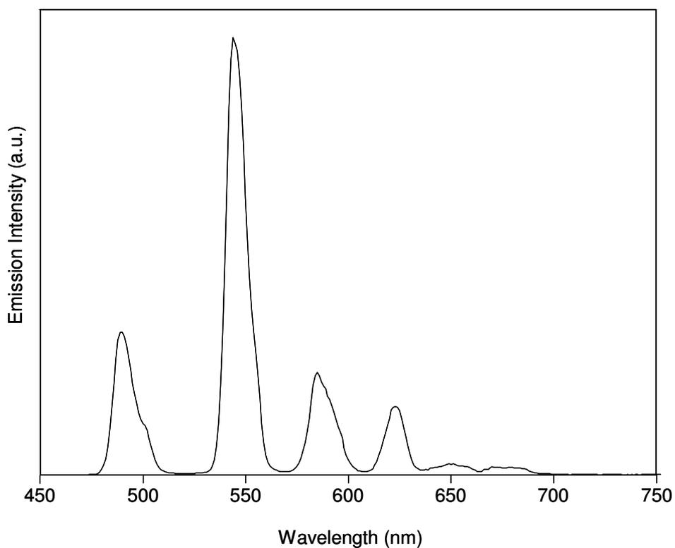
Corrected emission spectrum of terbium complex **8** ( $1 \times 10^{-6}$  M in Tris buffer 50 mM, pH 7.4) at 298K.
