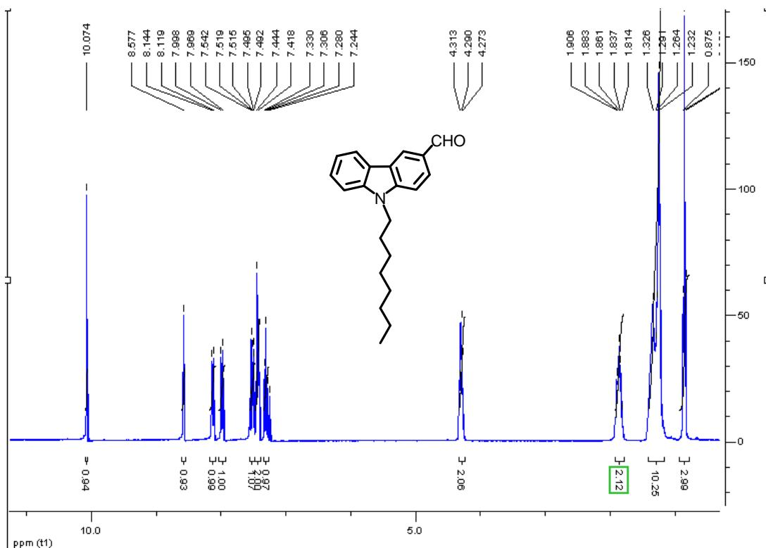
**Fig. S5** <sup>1</sup>H-NMR (300 MHz, CDCl<sub>3</sub>) spectrum of compound 3.
