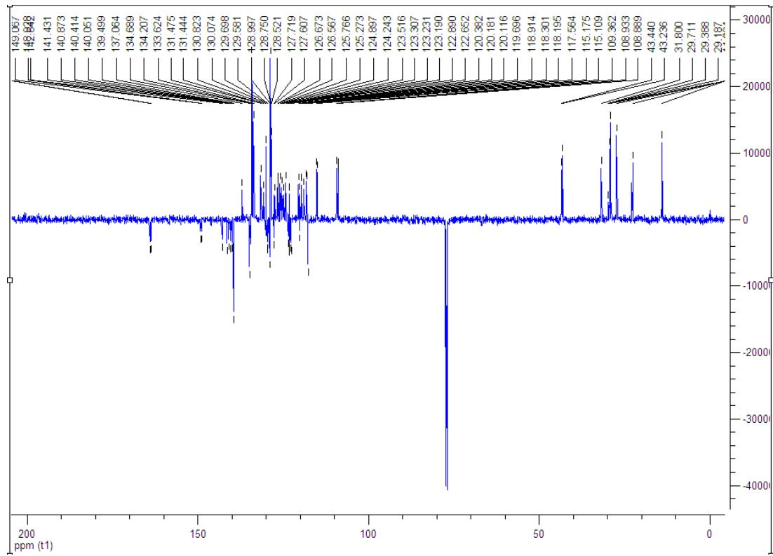
**Fig. S26** <sup>13</sup>C-NMR (125 MHz, CDCl<sub>3</sub>) spectrum of compound 2.
