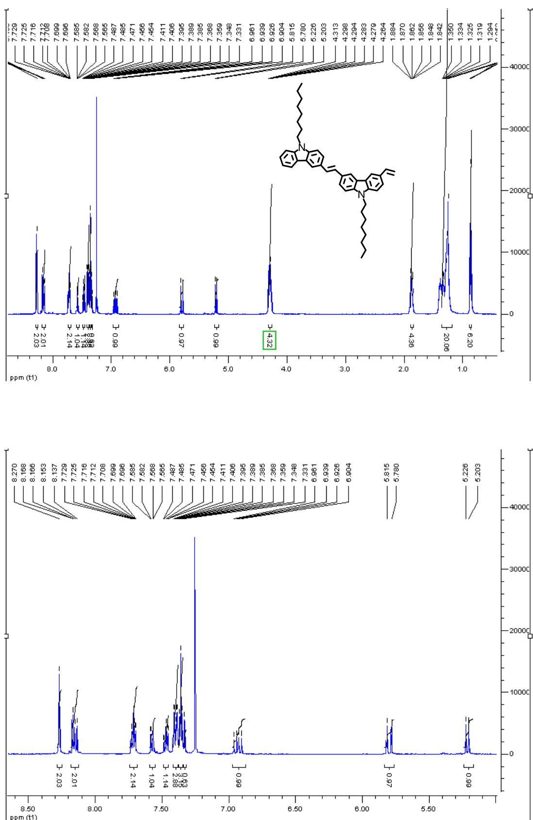
**Fig. S11**  $^1\text{H}$ -NMR (500 MHz,  $\text{CDCl}_3$ ) spectrum of compound 7.
