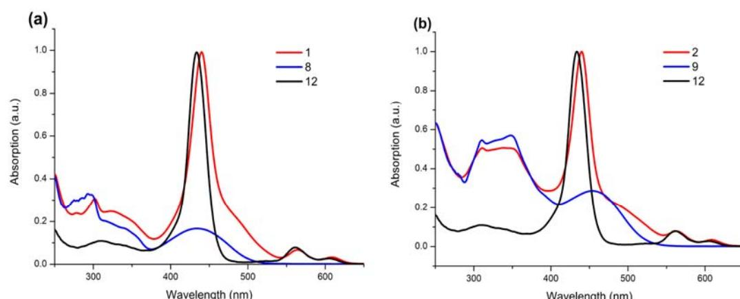
**Fig. S2** Normalized UV-vis absorption of (a) phosphorus (V) porphyrins **1** and **12** ( $5.0 \times 10^{-6}$  M), and compound **8** ( $1.0 \times 10^{-5}$  M) in chloroform; (b) phosphorus (V) porphyrins **2** and **12** ( $5.0 \times 10^{-6}$  M), and compound **9** ( $1.0 \times 10^{-5}$  M) in chloroform.
