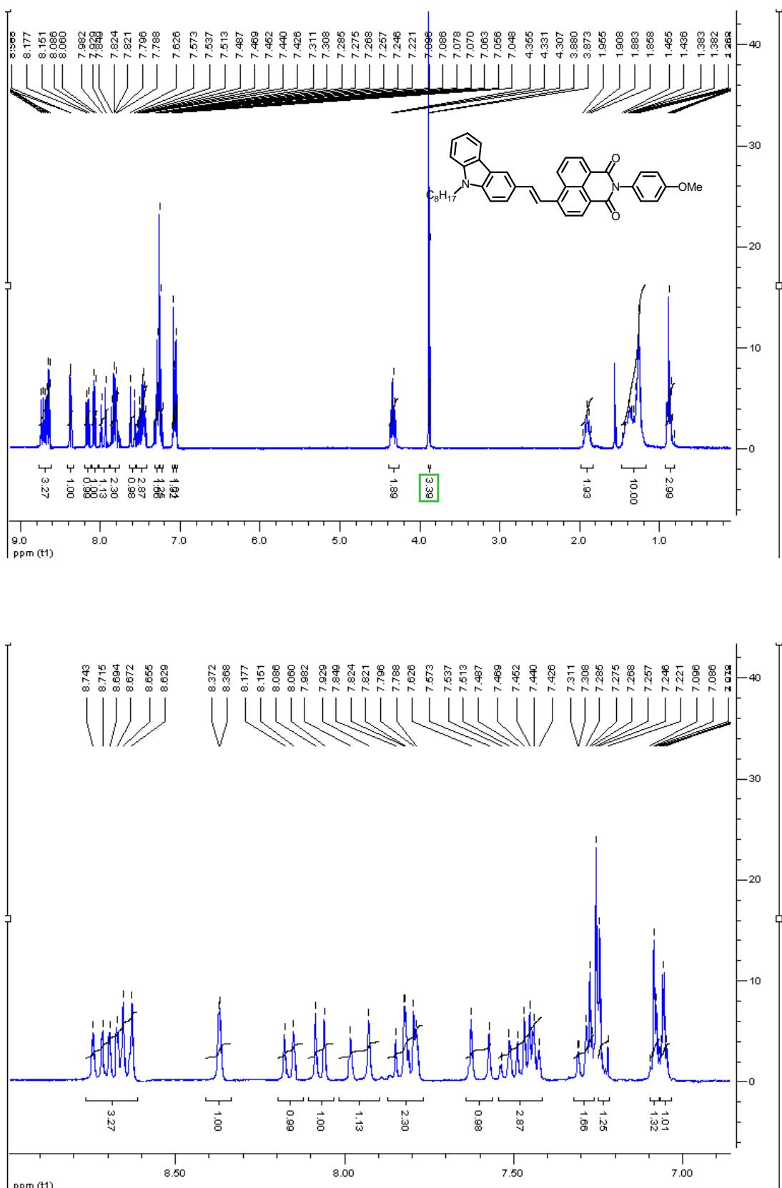
**Fig. S13** <sup>1</sup>H-NMR (300 MHz, CDCl<sub>3</sub>) spectrum of compound 8.
