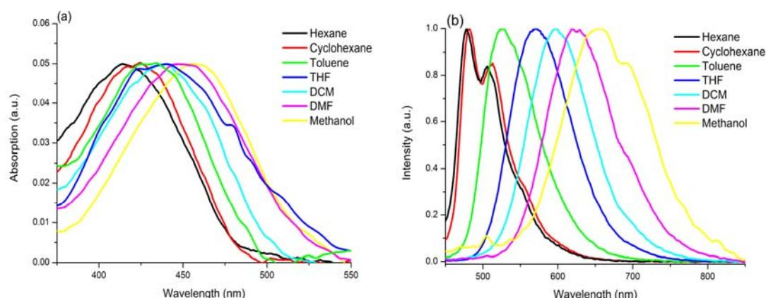
**Fig. S1** Normalized (a) UV-vis absorption and (b) Fluorescence emission spectra of compound **8** in different solvents ( $1.0 \times 10^{-6}$  M,  $\lambda_{\text{ex}} = 440$  nm).
