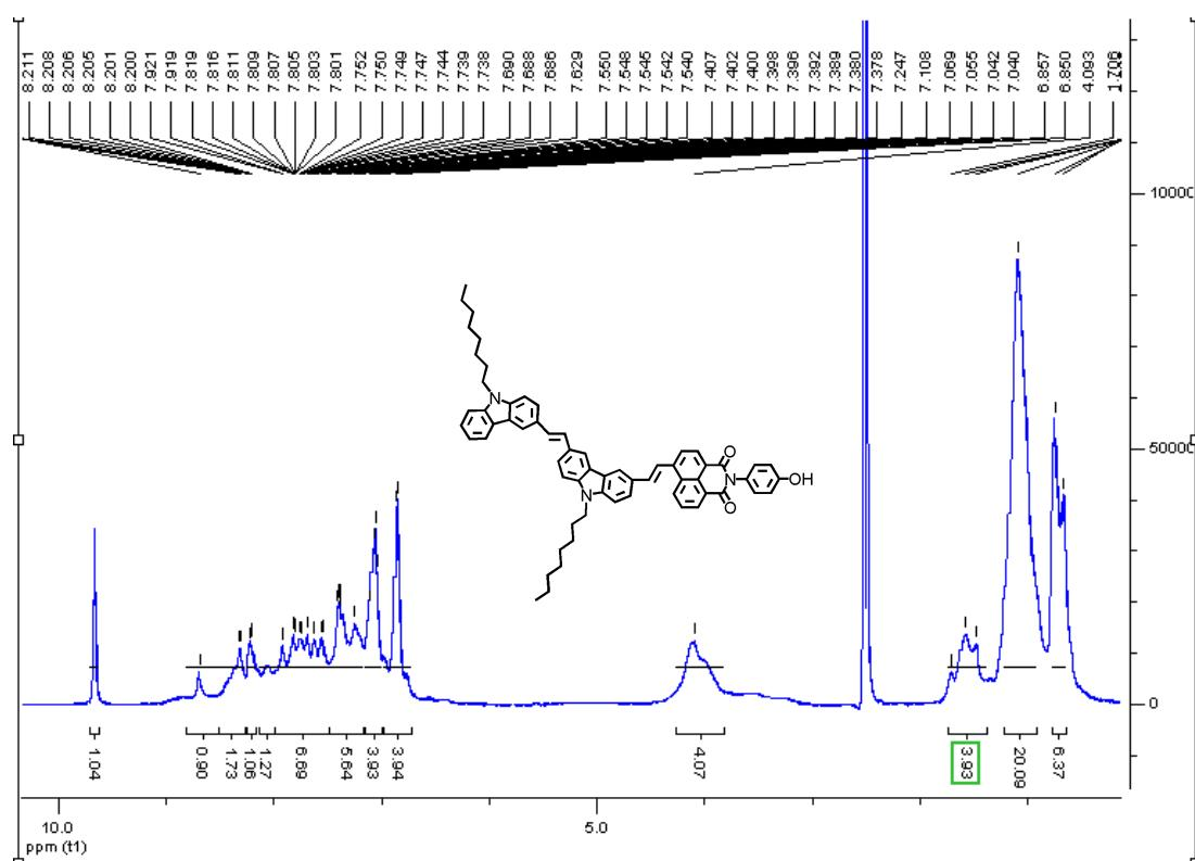
**Fig. S19**  $^1\text{H}$ -NMR (300 MHz, DMSO- $\text{d}_6$ ) spectrum of compound **11**.
