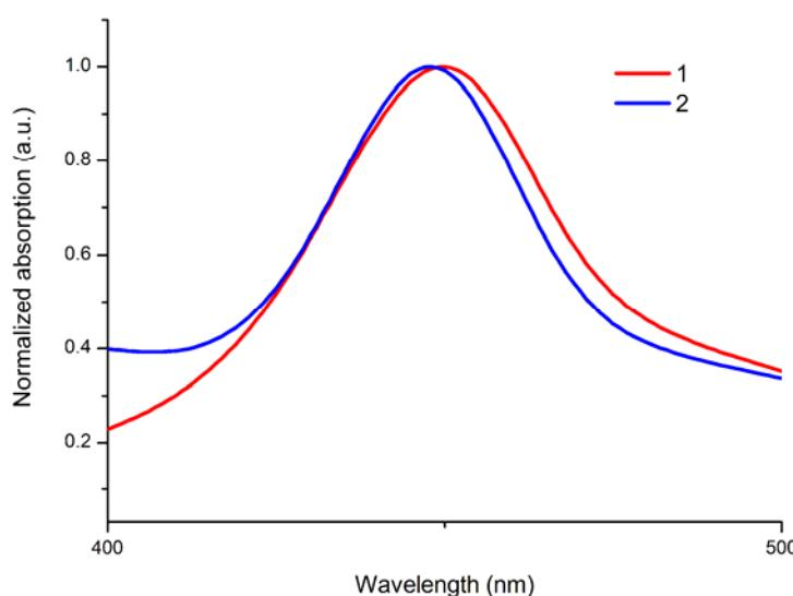
**Fig. S3** Normalized UV-vis absorption spectra of phosphorus (V) porphyrins **1** and **2** in the film.
