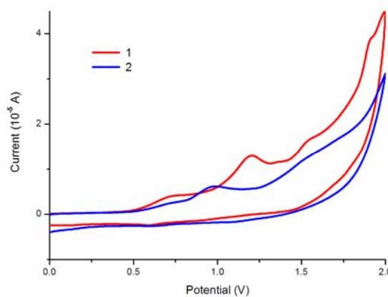
**Fig. S4** Cyclic voltammogram diagrams of phosphorus (V) porphyrins **1** and **2** in anhydrous  $\text{CH}_2\text{Cl}_2$  with 0.1 M  $\text{Bu}_4\text{NBF}_4$  as electrolyte at a scan rate of  $100 \text{ mV s}^{-1}$ .
