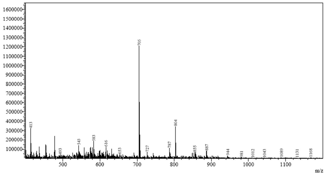
**Fig. S8** ESI mass spectra (positive ion mode) of the eluant fraction collected at 7.856 min in RP-HPLC (Fig. S5). Mass peak at  $m/z = 705$ , (calculated for  $[C_{38}H_{43}N_2O_7S_2^- + H]^+$ ) corresponding to this cyanine dye (**Cy-quinone**).
