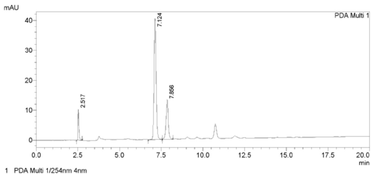
**Fig. S5** RP-HPLC (grad. 20-100% ACN in water, 20 min.) of the reaction mixture of **DNBS-Cy** and GSH in 10 mM PBS buffer medium (pH = 7.4).
