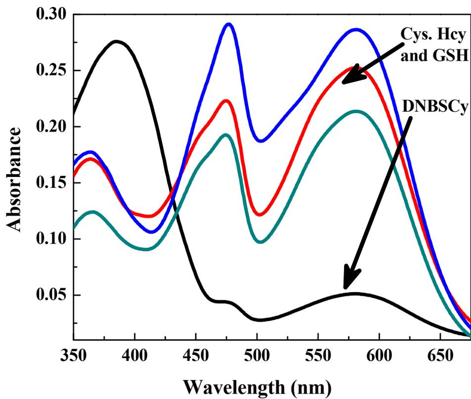
**Fig. S1** UV/Vis absorption spectra of **DNBSCy** (10.0  $\mu\text{M}$ ) and on addition of 10.0 equivalents of Cys, Hcy and GSH in 10 mM PBS buffer medium (pH = 7.4).
