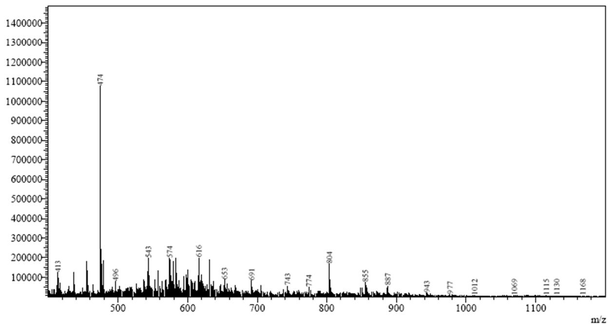
**Fig. S7** ESI mass spectra (positive ion mode) of the eluant fraction collected at 7.124 min in RP-HPLC (Fig. S5). Mass peak at  $m/z = 474.0$  corresponding to the side product  $\gamma$ -glutamyl-S-(2,4-dinitrophenyl)cysteinylglycine (calculated for  $C_{16}H_{19}N_5O_{10}S$ ).
