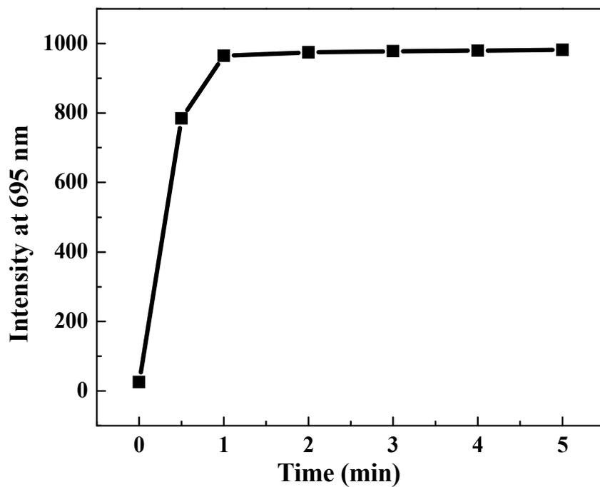
**Fig. S12** Emission intensity response of the probe **DNBSy** (10.0  $\mu$ M) upon addition of 2 mM of GSH in the 10 mM PBS buffer solution (pH 7.4).
