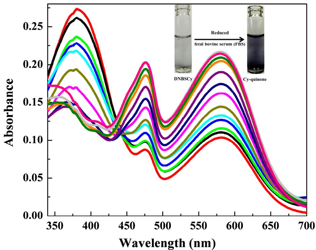
**Fig. S9** Absorption spectra of probe **DNBSy** (10.0 μM) upon addition of various amounts (0, 5, 10, 15, 20, 30, 40, 50, 60, 70, 80, 90, 100 μL) of reduced fetal bovine serum solution to the 10 mM PBS buffer solution (pH 7.4).
