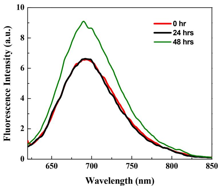
Fig. S14 Emission spectra of probe DNBSCy (10.0 μM) in water.
