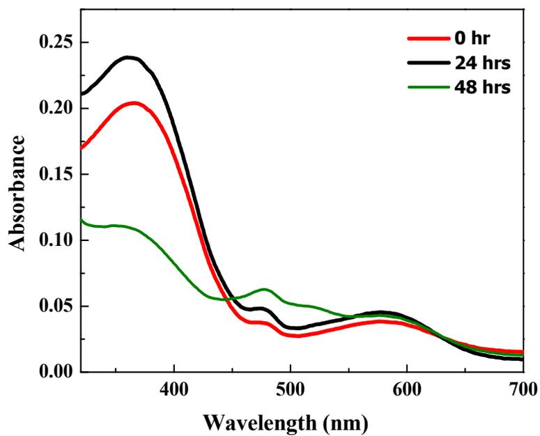
Fig. S13 Absorption spectra of probe DNBSCy (10.0 μM) in water.
