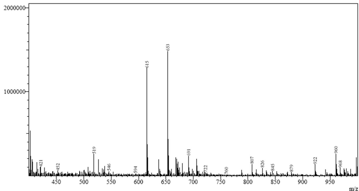
**Fig. S6** ESI mass spectra (positive ion mode) of the eluant fraction collected at 2.517 min in RP-HPLC (Fig. S5). Mass peak observed at 615 ( $[M + 2H]^+$ ) and 653 ( $[M + H + K]^+$ ) were attributed to the oxidized form of GSH (GS-SG).
