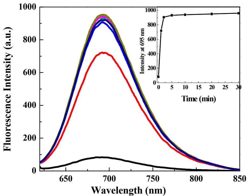
**Fig. S10** Fluorescence spectra of probe DNBSy (10.0 μM) in response to enzymatic conversion of GSSG (2 mM) to free GSH using glutathione reductase (1 unit/mL) and 0.4 mM of NADPH in the 10 mM PBS buffer solution (pH 7.4).
