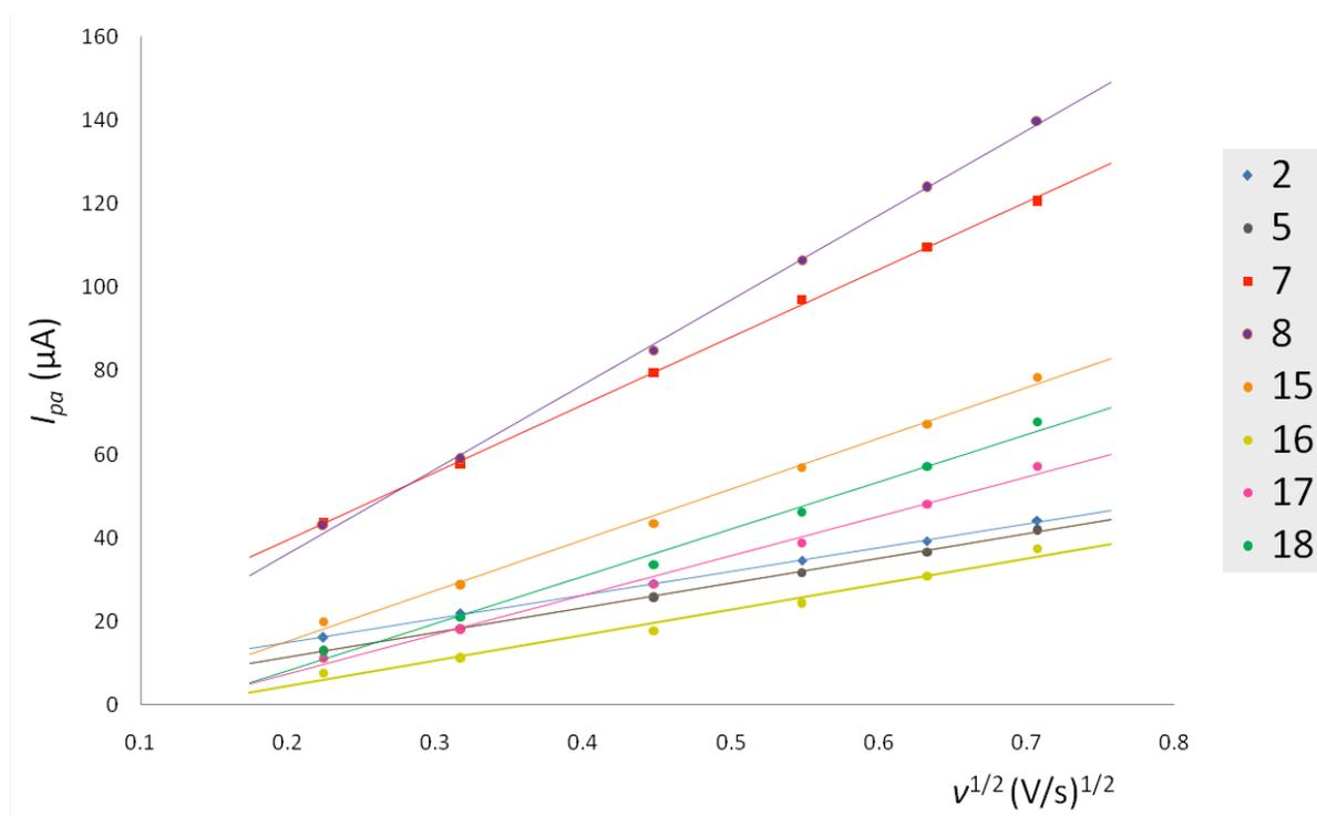
**Figure S6.** Representation of the anodic peak current ( $I_{pa}$ ) versus square root of the sweep rate ( $v^{1/2}$ ) for the ferrocene derivatives in acetonitrile. The diffusion coefficients were calculated by linear fitting of  $I_{pa}$  versus  $v^{1/2}$  in accordance with the Randles-Sevcik equation [Eq. 1].
