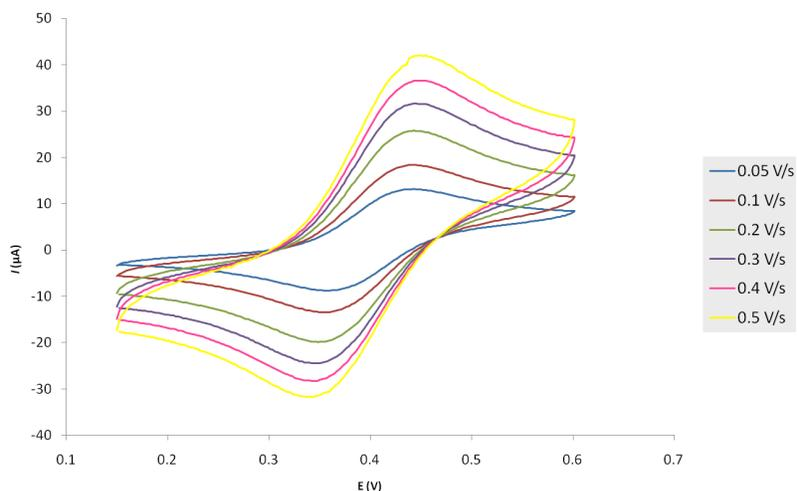
**Figure S2.** Cyclic voltammetry curves (5 scans) of the ferrocene derivative **5** (0.2 mM) in 50mM NaClO<sub>4</sub> acetonitrile solution at 25°C and different sweep rates (from 0.05 to 0.5 V/s).
