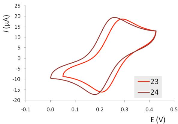
**Figure S5.** Cyclic voltammetry curves (5 scans; sweep rate = 0.2V/s) of the ferrocene derivatives **23** and **24** (0.2 mM) in 50mM  $\text{NaClO}_4$  aqueous solution at 25°C.
