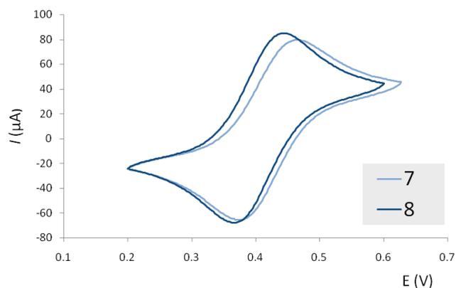
**Figure S3.** Cyclic voltammetry curves (5 scans; sweep rate = 0.2V/s) of the ferrocene derivatives **7** and **8** (0.2 mM) in 50mM  $\text{NaClO}_4$  acetonitrile solution at 25°C.
