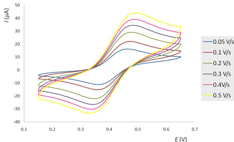
**Figure S1.** Cyclic voltammetry curves (5 scans) of the ferrocene derivative **2** (0.2 mM) in 50mM NaClO<sub>4</sub> acetonitrile solution at 25°C and different sweep rates (from 0.05 to 0.5 V/s).
