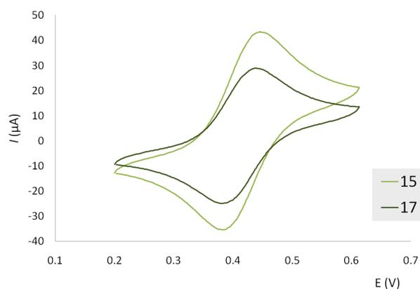
**Figure S4.** Cyclic voltammetry curves (5 scans; sweep rate = 0.2V/s) of the ferrocene derivatives **15** and **17** (0.2 mM) in 50mM  $\text{NaClO}_4$  acetonitrile solution at 25°C.
