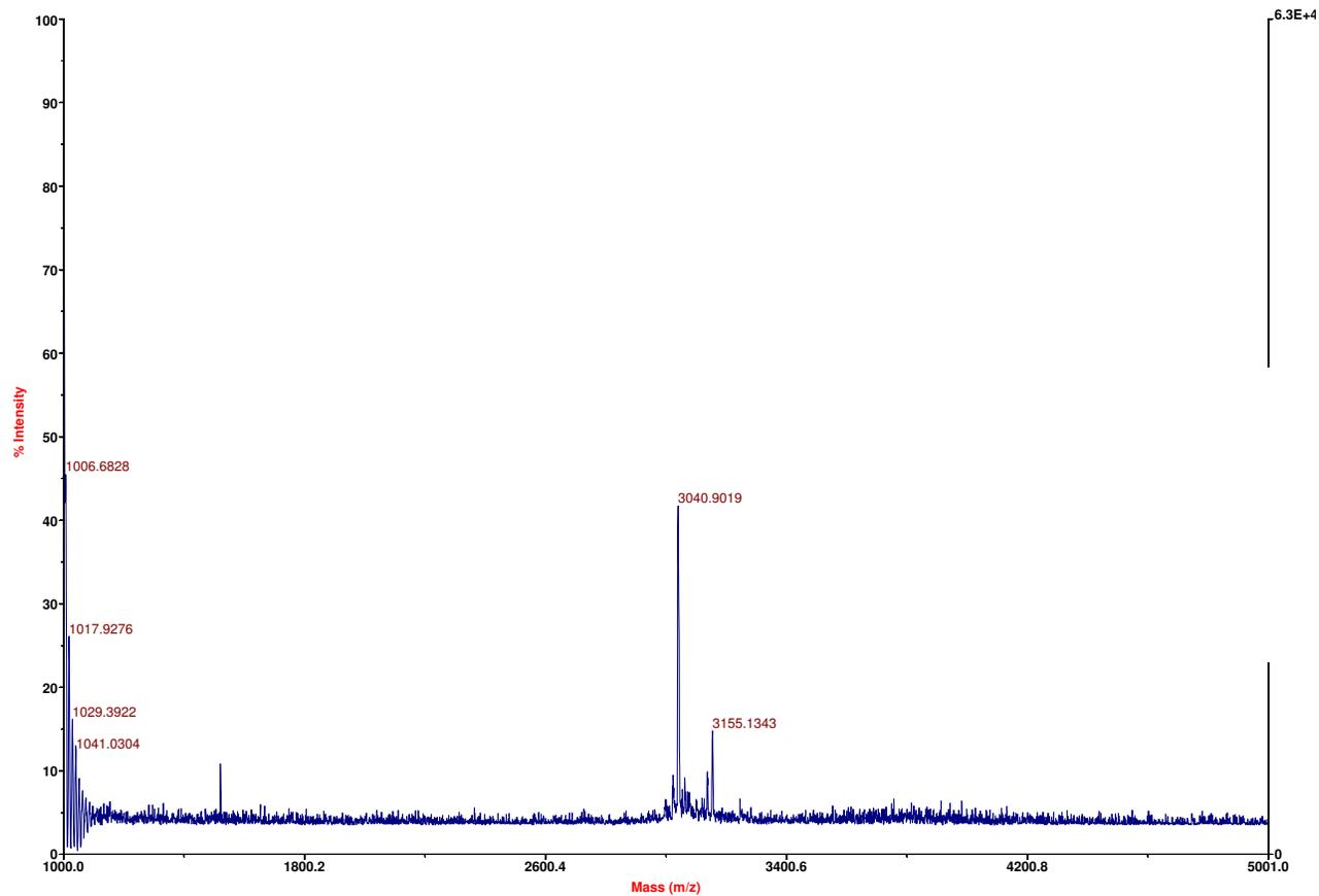
*Tris-disulfide formation of residue 24 substitution with glutamine (2) (M(O)24Gln)*
