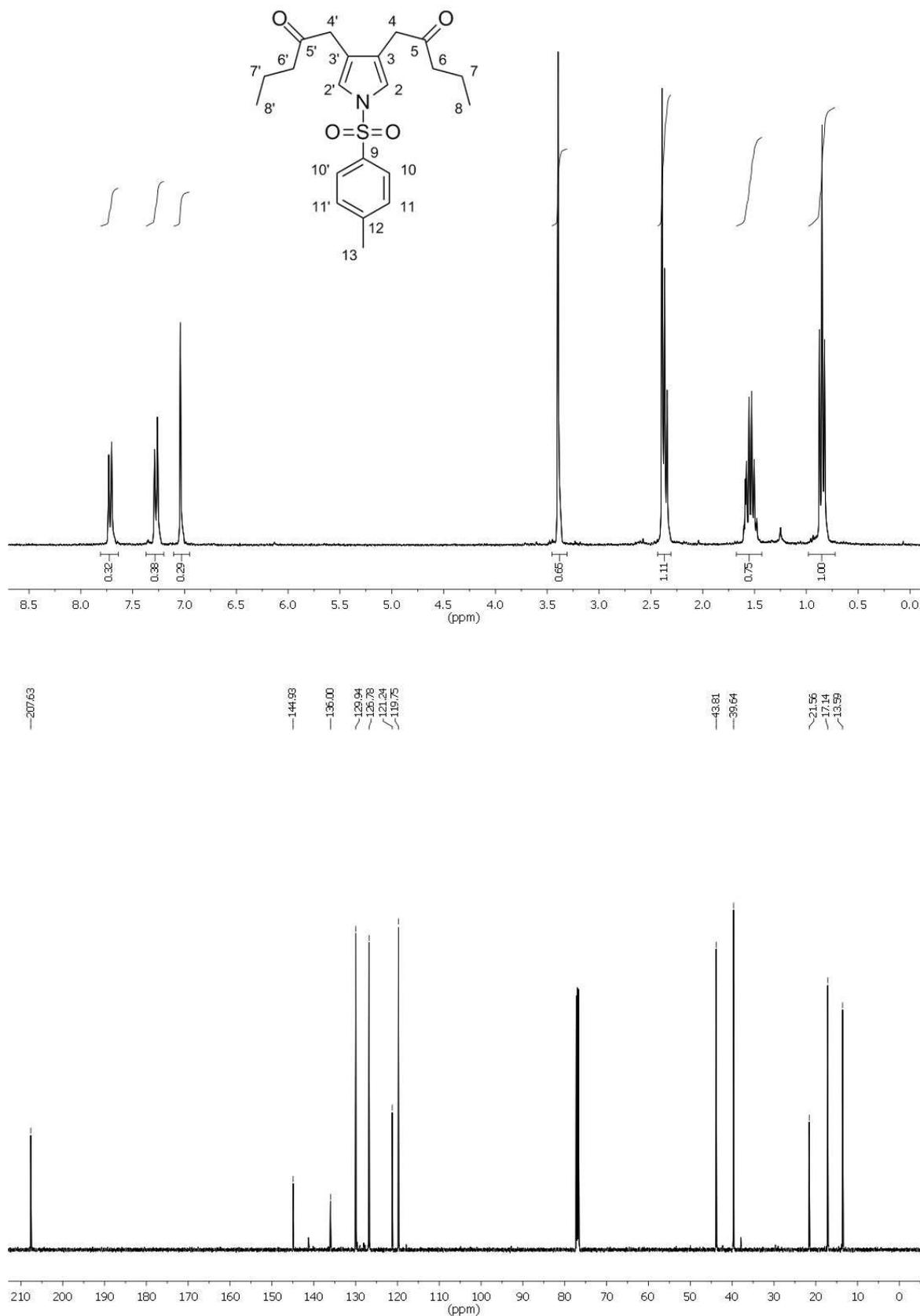
Compound 25ca ( $^1\text{H-NMR}$  (300 MHz,  $\text{CDCl}_3$ ),  $^{13}\text{C-NMR}$  (125 MHz,  $\text{CDCl}_3$ ))
