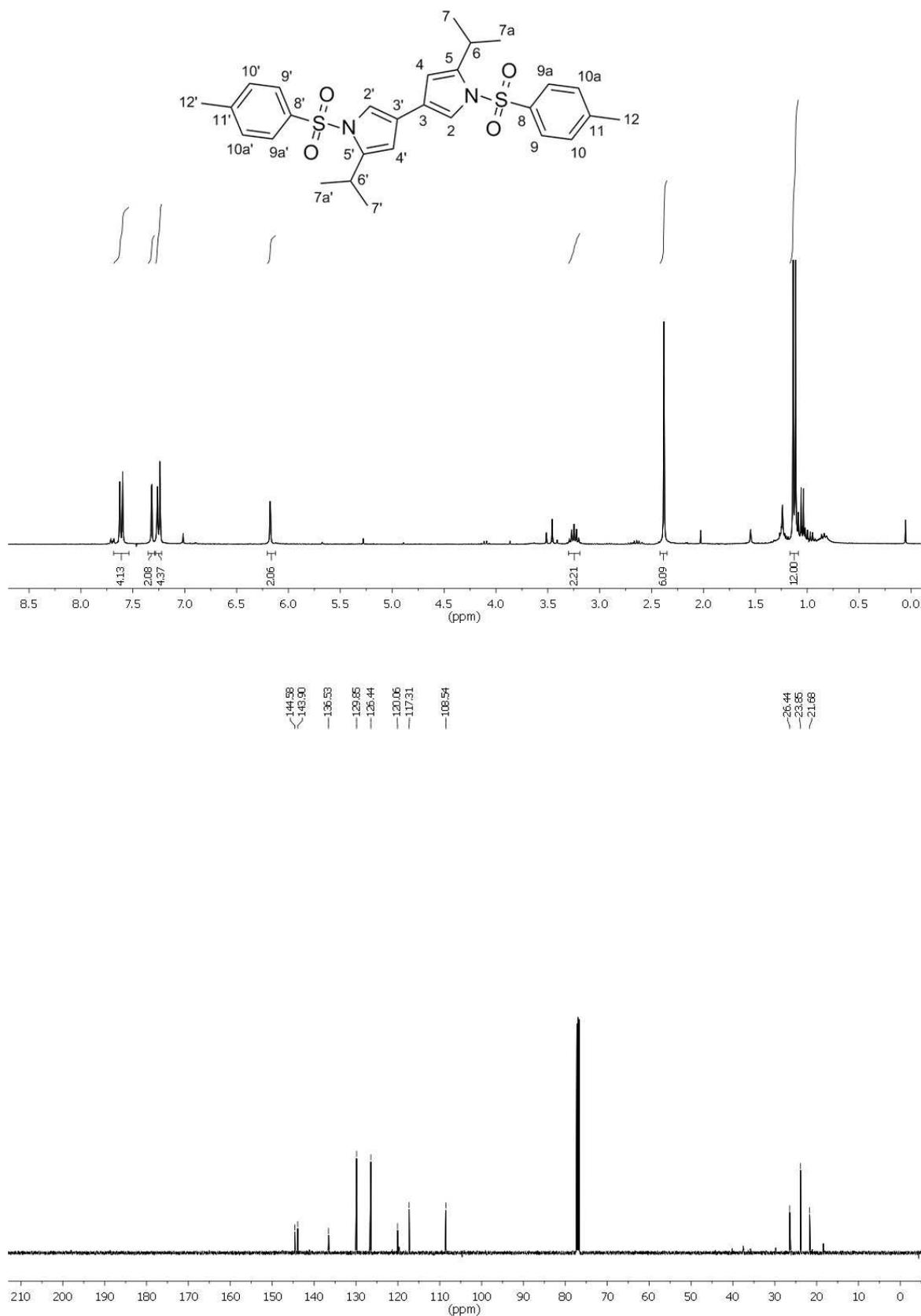
Compound 26cb ( $^1\text{H-NMR}$  (300 MHz,  $\text{CDCl}_3$ ),  $^{13}\text{C-NMR}$  (125 MHz,  $\text{CDCl}_3$ ))
