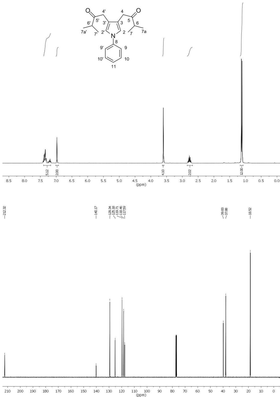
Compound 25cb ( $^1\text{H-NMR}$  (300 MHz,  $\text{CDCl}_3$ ),  $^{13}\text{C-NMR}$  (125 MHz,  $\text{CDCl}_3$ ))
