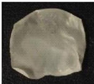
**Figure S1.** An example of a PAMA film obtained from polymer PAMA3 (44% AN, 49% MMA, 7% AA) by phase inversion from acetone to water.
