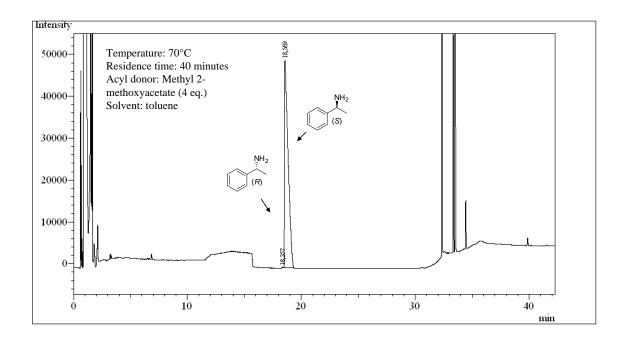
2.1.5. Variation of acyl dono:substrate ratio in the kinetic resolution of (+/-)-1phenylethylamine with Methyl 2-methoxyacetate as acyl donor under continuous flow conditions
