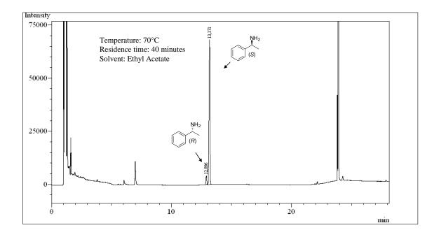
**2.1.6.** Kinetic resolution of (+/-)-1-phenylethylamine with different immobilized enzymes under continuous flow conditions
