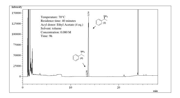
**2.1.8.** Evaluation of continuous flow system capability of operating with high concentration of substrate
