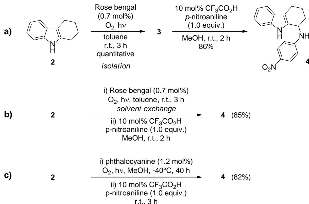
**Supplementary Figure S1 Investigation of the reaction sequence.** **a)** Two-step protocol with isolation of intermediate hydroperoxide **3**. **b)** One-pot, two-step protocol exchanging the solvent without isolation of hydroperoxide **3**. **c)** One-pot, two-step protocol in methanol without need to exchange the solvent.
