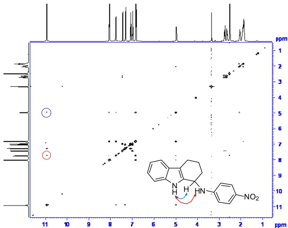
**Supplementary Figure S3: NOESY of 4 in DMSO (to determine the position of the new C-N bond)**
