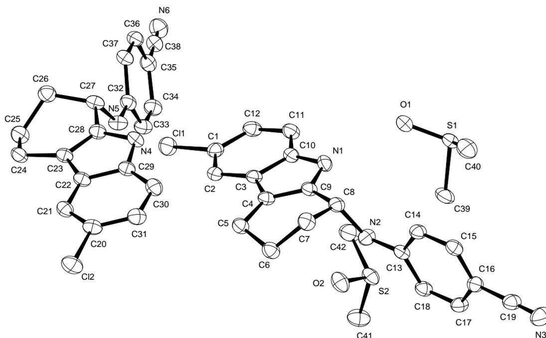
**Supplementary Figure S9** X-ray structure of 4-(6-chloro-2,3,4,9-tetrahydro-1H-carbazol-1-ylamino)benzotrile (21)
