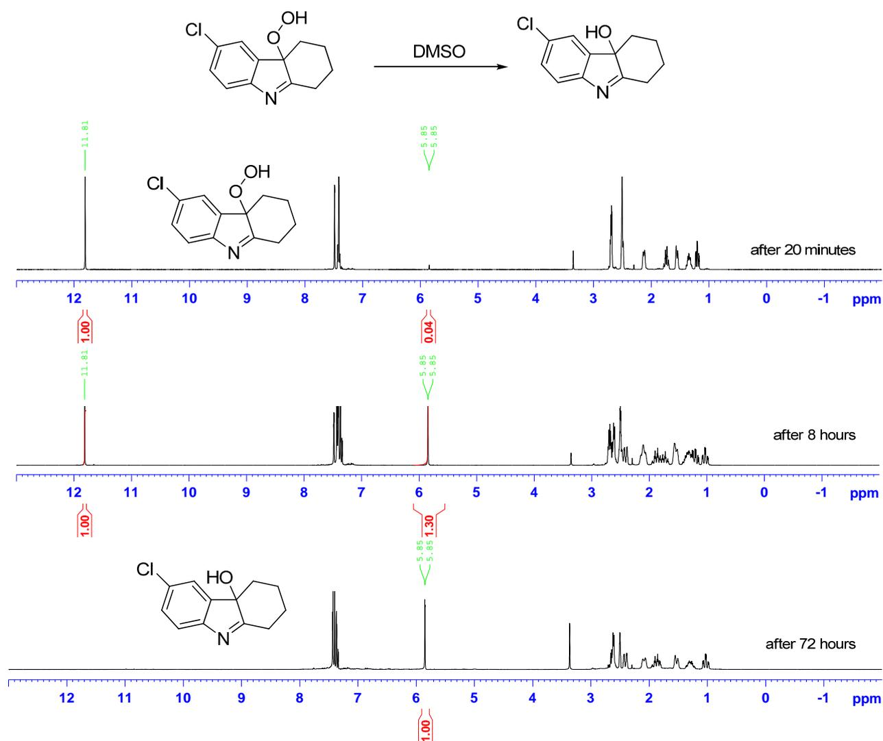
Supplementary Figure S7 Reduction of a tetrahydrocarbazole hydroperoxide in DMSO-d<sub>6</sub>
