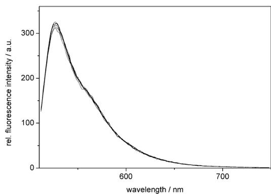
**Figure S4.** Fluorimetric detection of the displacement of TO (0.5 μM) from duplex DNA (0.25 μM in base pairs) by ligand **2<sup>PM</sup>**.
