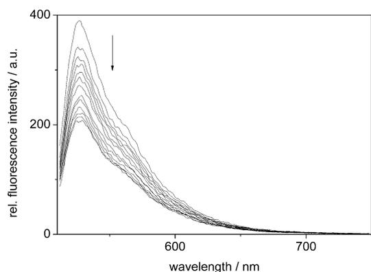
**Figure S3.** Fluorimetric detection of the displacement of TO (0.5 μM) from duplex DNA (0.25 μM in base pairs) by ligand **2<sup>SO</sup>**.
