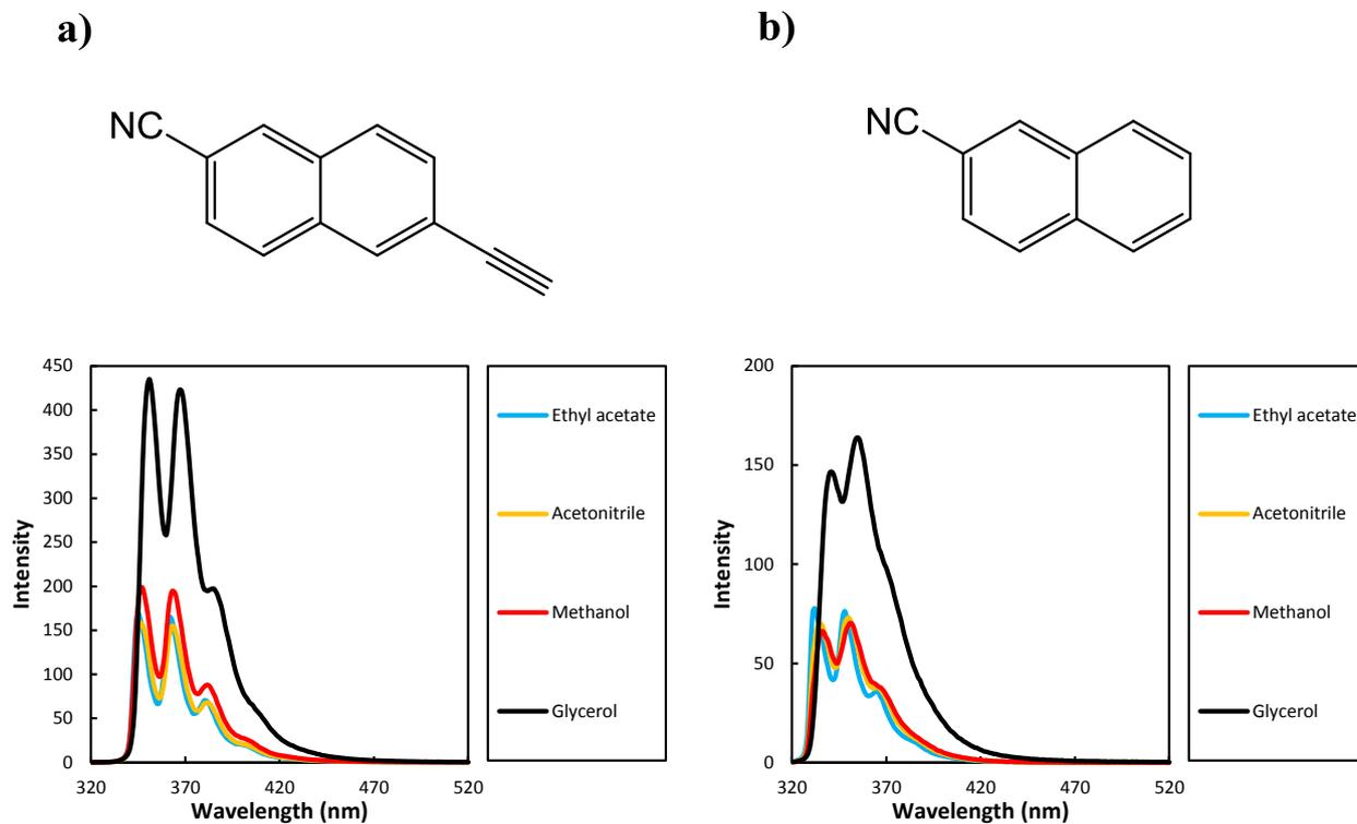
**Figure S2.** Fluorescence spectra of (a) 6-ethynyl-2-naphthonitrile (100  $\mu\text{M}$ ) and (b) 2-naphthonitrile (100  $\mu\text{M}$ ) in various solvents.
