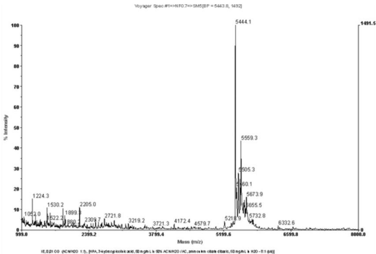
**Supplementary Fig 8** MALDI-TOF spectrum of mt-ASL<sup>Lys</sup> *S.cerevisiae* modified with cmm<sup>5</sup>s<sup>2</sup>U. Experimental monoisotopic mass for [M+H]<sup>+</sup> is 5453.4, the calculated monoisotopic mass is 5452.4 Da.
