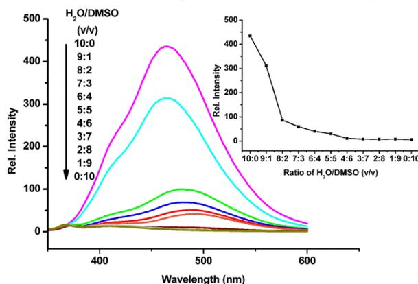
**Figure S4** Fluorescence responds of the reaction between **D-HMSe** (10 μM) and H<sub>2</sub>O<sub>2</sub> (200 μM) in different ratios of DMSO and H<sub>2</sub>O as solvent at ambient temperature for 1 h.
