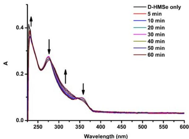
**Figure S8** Time-dependent UV spectra of **D-HMSe** (20  $\mu\text{M}$ ) reacted with  $\text{H}_2\text{O}_2$  (400  $\mu\text{M}$ ) in 60 min at ambient temperature in water (1% DMSO)
