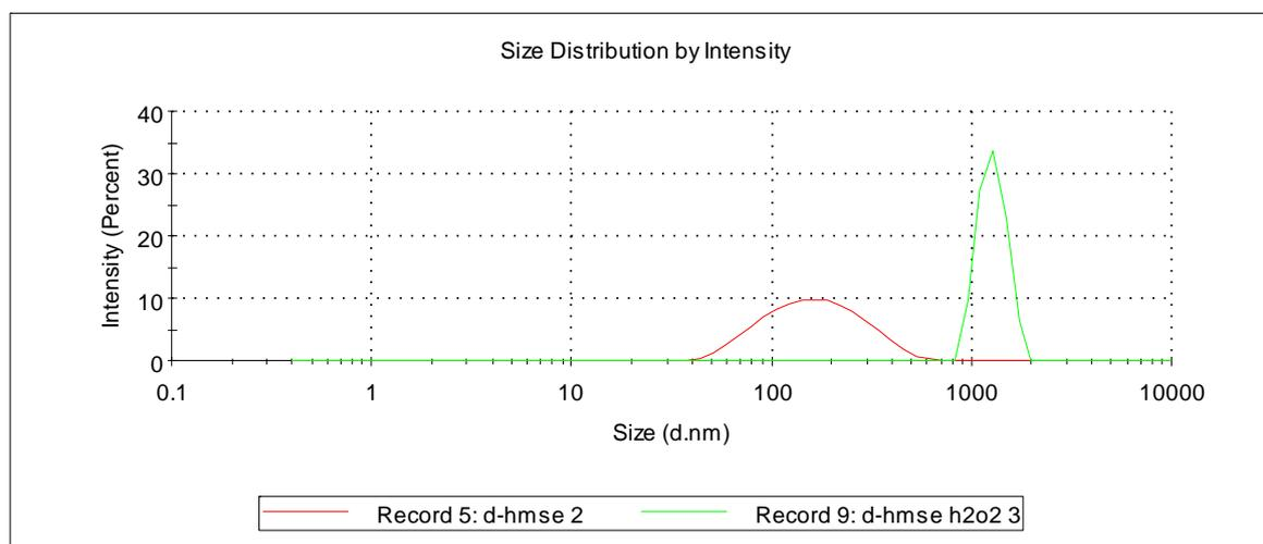
**Figure S6** Dynamic light scattering result of **D-HMSe** (10  $\mu$ M) before and after treated with  $H_2O_2$  (200  $\mu$ M) in DMSO/water (1/99, v/v) buffered by 20 mM HEPES at pH 7.40 at ambient temperature for 1 h.
