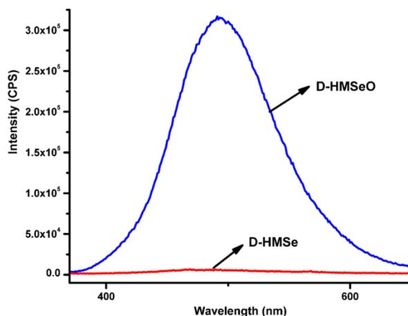
**Figure S3** Fluorescence spectra of **D-HMSe** and **D-HMSeO** in solid state.  $\lambda_{ex}$ =347 nm, slit: 5/5 nm.
