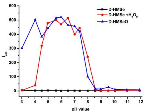
**Figure S7** Effect of pH on the relative fluorescence intensity for 10  $\mu\text{M}$  **D-HMSe** before ( $\bullet$ ), after ( $\blacksquare$ ) treated with 200  $\mu\text{M}$   $\text{H}_2\text{O}_2$  and 10  $\mu\text{M}$  **D-HMSeO** ( $\blacktriangle$ ) in DMSO/water (1/99, v/v) buffered by 20 mM HEPES at pH 7.40 for 1 h at ambient temperature. (The investigated pH values include 3.01, 4.02, 4.51, 4.97, 5.60, 5.97, 6.50, 7.00, 7.38, 7.99, 8.56, 8.97, 9.55, 10.05, 10.95 and 11.91).
