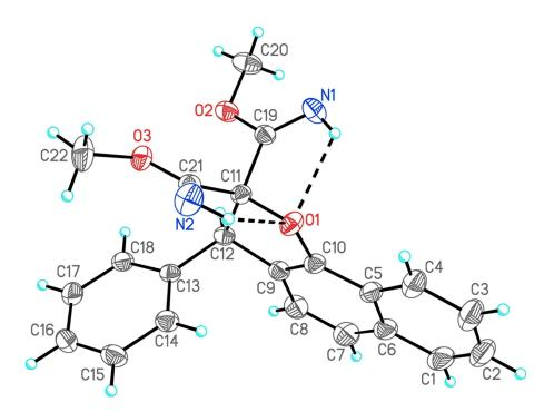
The ORTEP diagram of **6** with the atom-numbering scheme. Displacement ellipsoids are drawn at the 30% probability level and H atoms are shown as small spheres of arbitrary radius. The two intramolecular N-H…O hydrogen bonds are indicated by dotted lines [bond distances N-H, H…O, N…O and angle ∠N-H…O parameters are 0.87 Å, 2.26 Å, 2.722(2)Å, 116° for N1-H1N…O1 and 0.91 Å, 2.21 Å, 2.707(2)Å, 114° for N2-H2N…O1, respectively].
