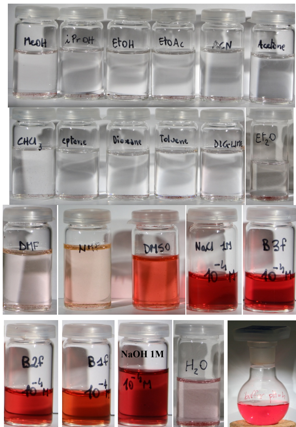
Figure S1. Solubility test for 1a . Legend: B1f → buffer pH = 10 (VWR, H 3 BO 3 /KCl/NaOH); B2f → buffer pH = 10 (Fisher, K 2 CO 3 /K 2 B 8 O 13 /KOH); B3f → buffer pH = 7 (VWR, KH 2 PO 4 /Na 2 HPO 4 ); Buffer pH = 4 (Fisher, C 8 H 5 KO 4 ).
