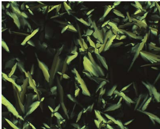
Columnar phase at 137.5 °C (x100 magnification)
