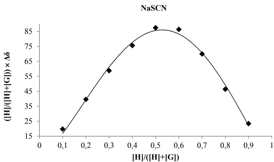
**Figure S9:** Job plot of NaSCN and Biotin[6]juril. Proton b is followed, see figure S1 for proton notation.
