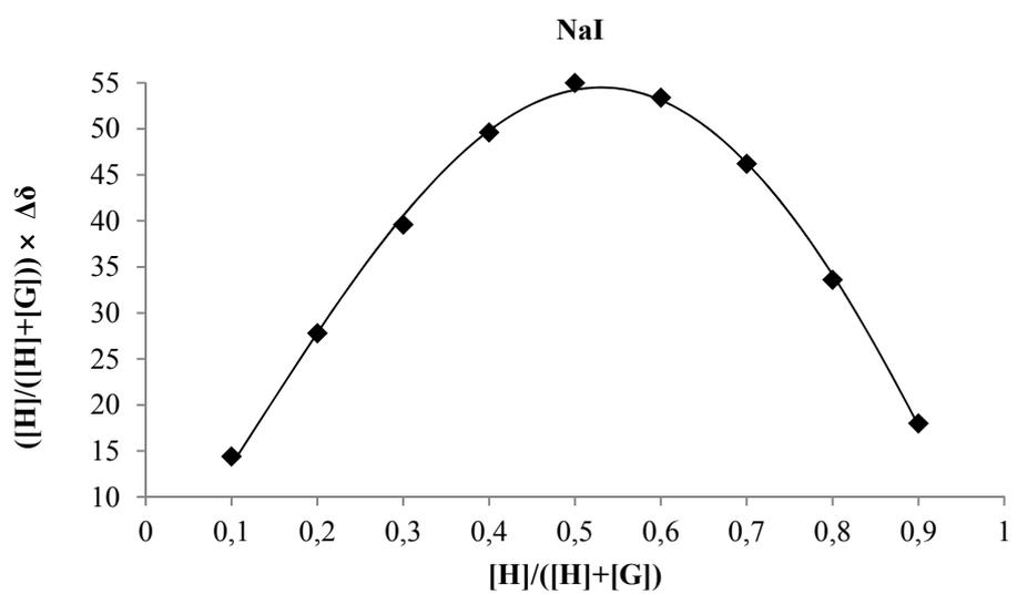
**Figure S6:** Job plot of NaI and Biotin[6]juril. Proton f is followed, see figure S1 for proton notation.
