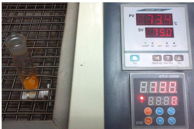
**Figure S4** Air-bath heating shaker.
