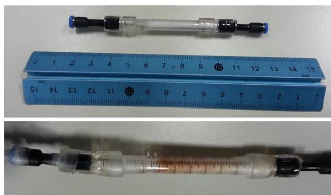
**Fig. S4.** Filters used in the transfer process from the DNP to the NMR to remove the residual radical traces from the hyperpolarized solution.
