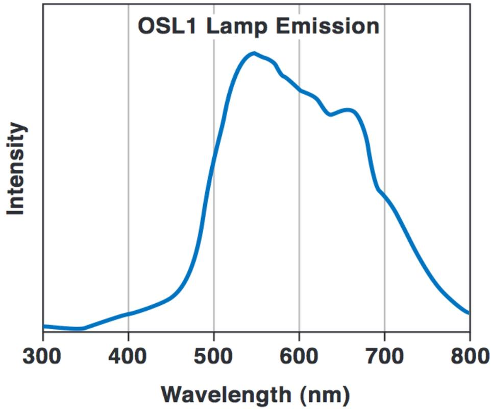
**Figure S1.** Electromagnetic spectrum of the white light source that was used for the white-light irradiation experiments (Thor Labs OSL1-EC Fiber Illuminator). *Source:* [www.thorlabs.de](http://www.thorlabs.de)
