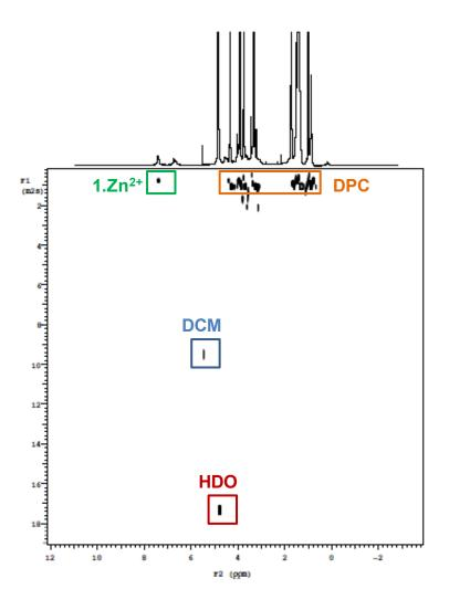
The x- and y- axis represent the regular <sup>1</sup>H chemical shift and the diffusion coefficient, respectively. DCM: residual dichloromethane; HDO: solvent signal chosen as reference for diffusion coefficient determination (D =  $19.02 \times 10^{-10} \text{ m}^2/\text{s}$  at 298 K).
