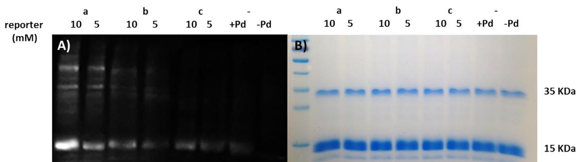
**Figure S24.** Detection of alkenylated histones extracted from RAW 264.7 cells via the oxidative Heck reaction using a biotinylated phenylboronic acid. A) Luminescence imaging on PVDF membrane of histones after 6 h incubation with 5 and 10 mM of a) sodium pent-4-enoate, b) *S*-propyl pent-4-enthioate and c) methyl 4-pentenoate. Control reactions in presence and absence of Pd are also shown. B) Coomassie staining of A).
