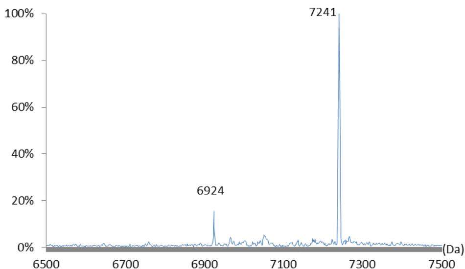
**Figure S4.** Coupling of **1** to **4-OT R61C-1** via the oxidative Heck reaction using 2-amino-4,6-dihydroxypyrimidine as ligand. ESI-MS spectrum: mass expected 7240, mass found 7241.
