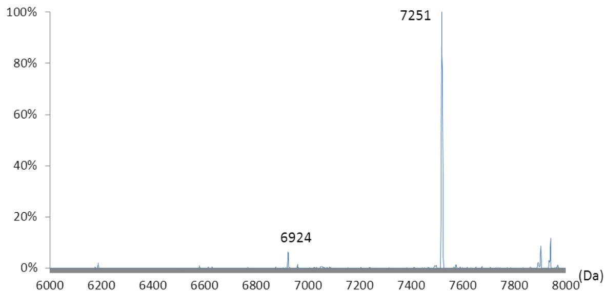
**Figure S6.** Coupling of **2** to **4-OT R61C-1** using the oxidative Heck reaction with EDTA as ligand. ESI-MS spectrum: mass expected 7252, mass found 7251.
