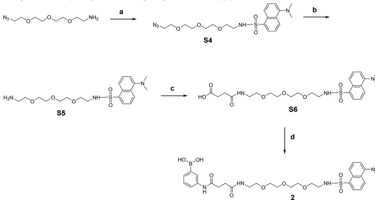
**Scheme S1:** Synthesis of (3-(1-(5-(dimethylamino)naphthalene-1-sulfonamido)-13-oxo-3,6,9-trioxa-12-azahexadecanamido)phenyl)boronic acid (**2**). a) Et<sub>3</sub>N, dansylchloride, CH<sub>2</sub>Cl<sub>2</sub>, 83% yield, b) H<sub>2</sub>, Pd/C 10%, MeOH, 99% yield, c) Et<sub>3</sub>N, succinic anhydride, THF, CH<sub>3</sub>CN, 99% yield, d) Et<sub>3</sub>N, BOP,3-aminophenylboronic acid, DMF, 51% yield.
