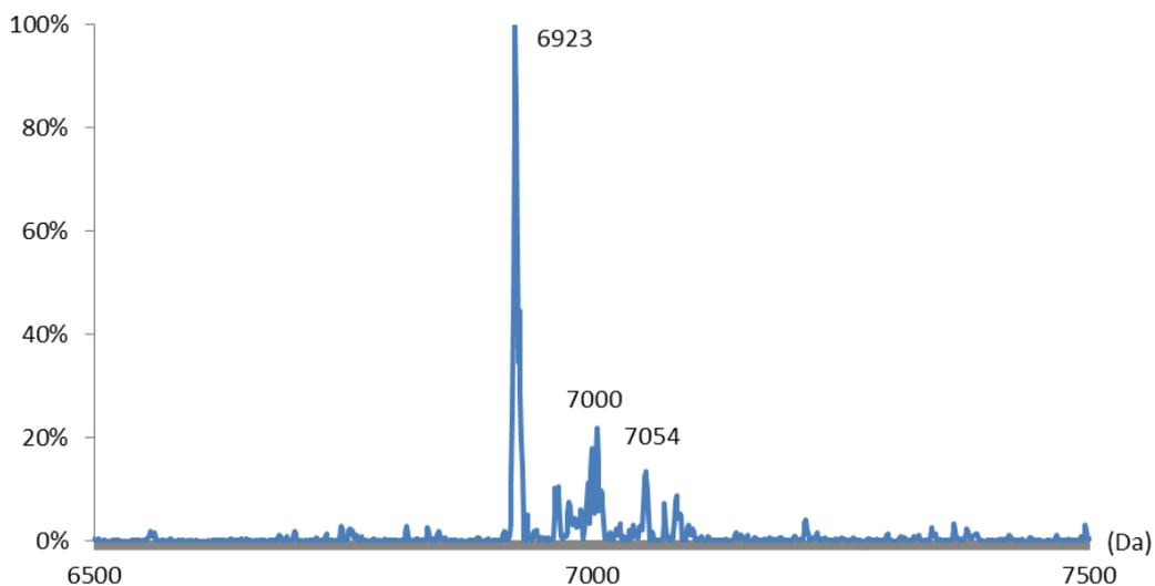
**Figure S12.** Oxidative Heck reaction on **4-OT R61C-1** at pH 3. ESI-MS spectrum: mass expected 7000, mass found 7000 (6923 unreacted protein, 7054 unreacted protein with methionine).
