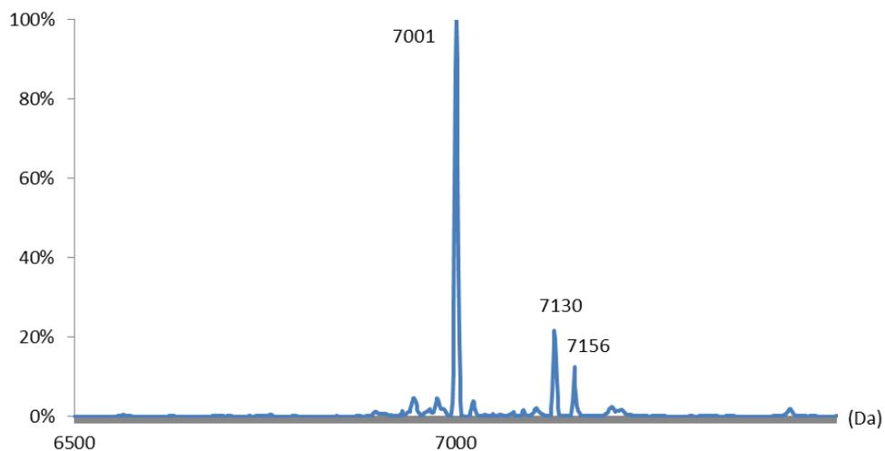
**Figure S14.** Oxidative Heck reaction on **4-OT R61C-1** at pH 7. ESI-MS spectrum: mass expected 7000, mass found 7001 (7130 reacted protein with methionine, 7156 reacted protein with formylated methionine).
