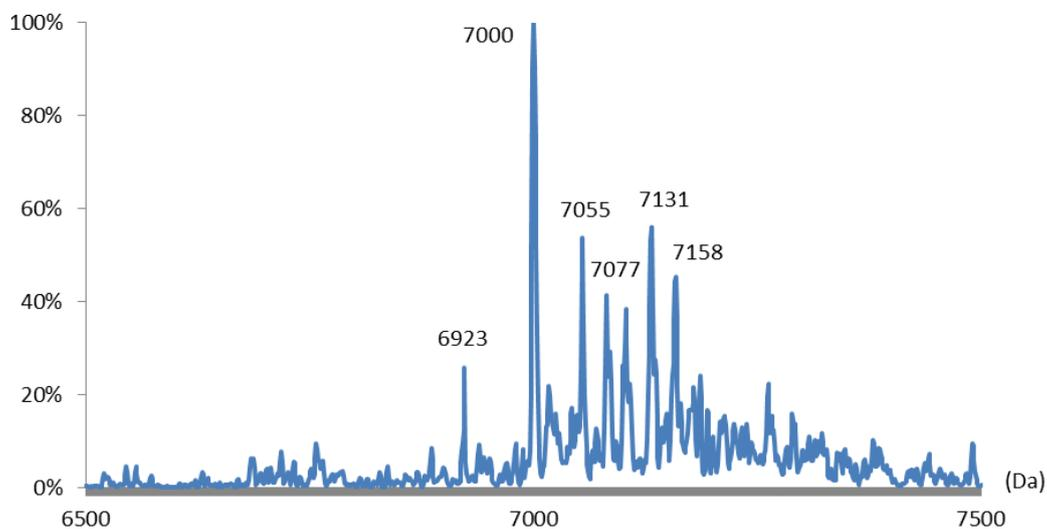
**Figure S15.** Oxidative Heck reaction on **4-OT R61C-1** at pH 9. ESI-MS spectrum: mass expected 7000, mass found 7000 (6923 unreacted protein, 7055 unreacted protein with methionine, 7077 double phenylated protein, 7131 phenylated protein with methionine, 7158 phenylated protein with formylated methionine).
