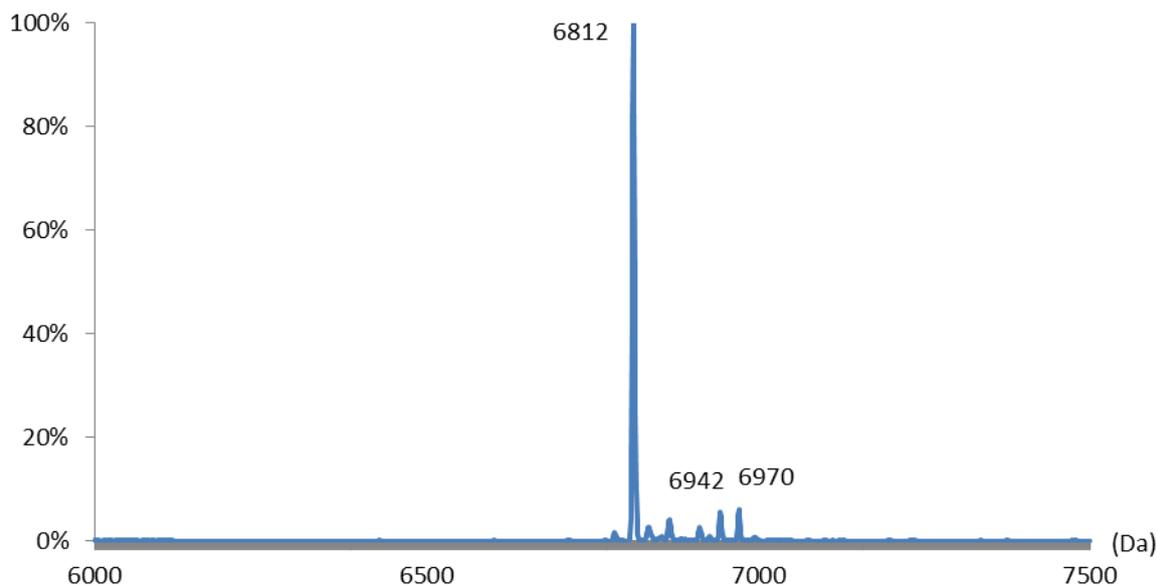
**Figure S17.** Wild type **4-OT** for control reactions on the stability of the enzyme. ESI-MS spectrum **4-OT**: mass expected= 6811, mass found= 6812 (6942: enzyme with methionine, 6970: enzyme with formylated methionine).
