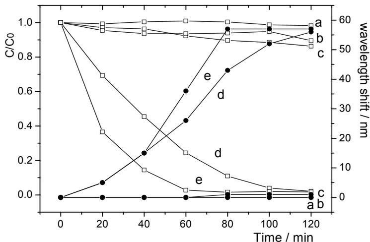
a, without any catalyst under visible light b, PS / TiO<sub>2</sub> (50% PS) composite in dark c, 0.1ml H<sub>2</sub>O<sub>2</sub> under visible light d, PS / TiO<sub>2</sub> (50% PS) composite under visible light e, PS / TiO<sub>2</sub> (50% PS) + 0.1ml H<sub>2</sub>O<sub>2</sub> under visible light. The solid symbols are the results of wavelength.
