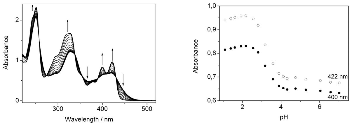
**Figure S5.** Left: Spectrophotometric titration of acid to acridizinium derivative **3** ( $c = 1.0 \times 10^{-4}$  M in Britton-Robinson buffer); arrows indicate the development of absorption bands upon addition of acid (from pH = 7.0 to pH = 1.0); right: plot of the absorption of **3** at 400 and 422 nm vs the pH of the solution (the decrease of absorption at pH < 2 is likely due to partial hydrolysis of the benzimidazole substituent under these conditions).
