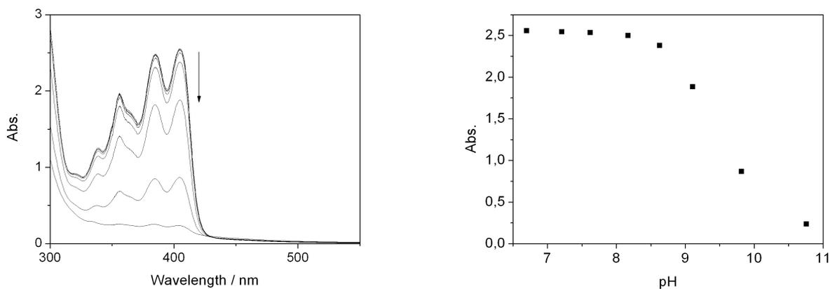
**Figure S2.** Left: Spectrophotometric titration of base to acridizinium derivative **1a** ( $c = 1.8 \times 10^{-4}$  M in Britton-Robinson buffer); arrows indicate the development of absorption bands upon addition of base, right: plot of the absorbance of **1a** vs pH of the solution.
