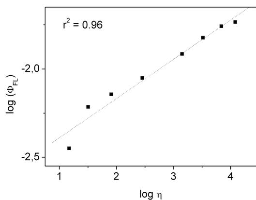
**Figure S4.** Dependence of the fluorescence quantum yield,  $\phi_{\text{Fl}}$ , of the acridizinium derivative **2** on the viscosity,  $\eta$ , of the glycerol solution given as plot of  $\log \phi_{\text{Fl}}$  versus  $\log \eta$ ; different viscosities of the glycerol solution were adjusted by variation of the temperature.
