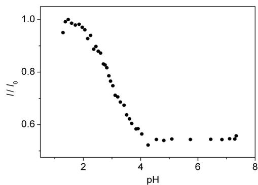
**Figure S3.** Dependence of the pH value on the emission intensity of acridizinium derivative **2** ( $c = 1.0 \times 10^{-5}$  M in Britton-Robinson buffer) presented as plot of the relative fluorescence intensity vs the pH of the solution;  $\lambda_{\text{ex}} = 300$  nm.
