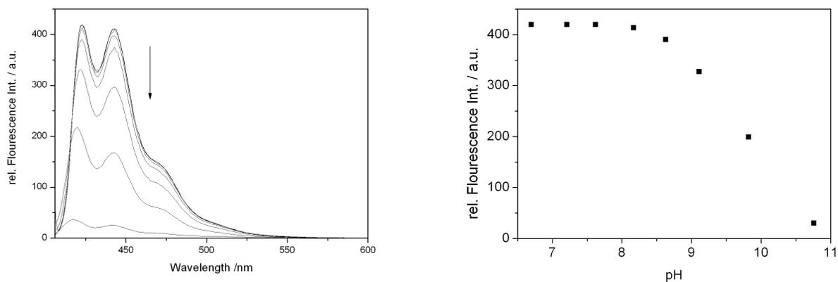
**Figure S1.** Left: Spectrofluorimetric titration of base to acridizinium derivative **1a** ( $c = 1.8 \times 10^{-4}$  M in Britton-Robinson buffer); arrows indicate the development of emission bands upon addition of base; right: plot of the relative emission intensity of **1a** vs pH of the solution.
