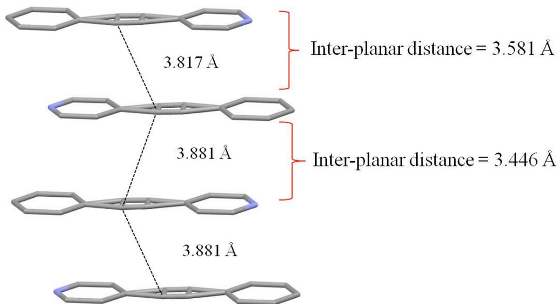
**Figure S25** Packing arrangement of stilbazole.HCl salt. Note the disorder of the olefinic carbons.
