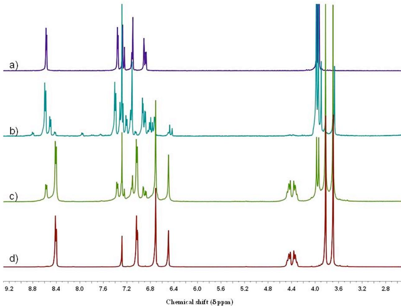
**Figure S11** (a)  $^1\text{H}$  NMR in  $\text{CDCl}_3$  of 3, 4-dimethoxy-stilbazole, **10** (b) after irradiation of 3, 4-dimethoxy-stilbazole for 72 h in solid state, (c) neutral extract of 3, 4-dimethoxy-stilbazole.HCl, irradiated for 168 h in solid state, (d) neutral extract of 3, 4-dimethoxy-stilbazole.HCl irradiated for 72 h as suspension in hexane.
