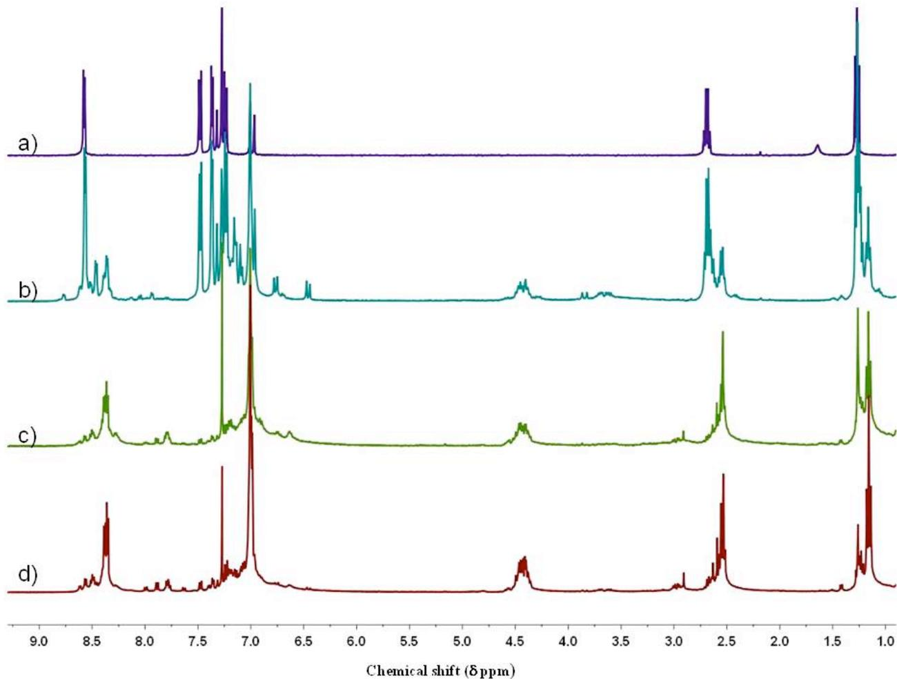
**Figure S9** (a) <sup>1</sup>H NMR in CDCl<sub>3</sub> of 4-ethyl-stilbazole, **8** (b) after irradiation of 4-ethyl-stilbazole for 20 h in solid state, (c) neutral extract of 4-ethyl-stilbazole.HCl, irradiated for 130 h in solid state, (d) neutral extract of 4-ethyl-stilbazole.HCl irradiated for 112 h as suspension in hexane.
