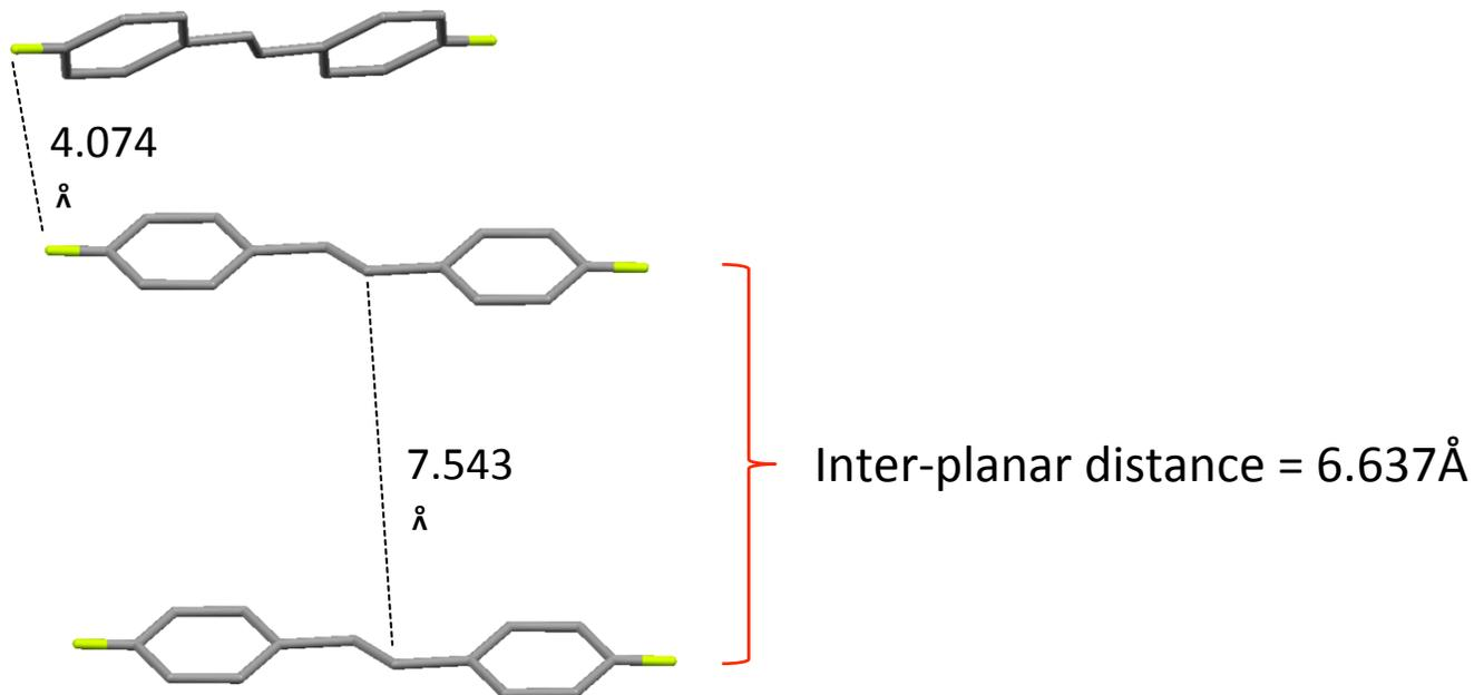
**Figure S20** Packing arrangement of 4-fluoro-stibazole (**2**). (Whole molecule disorder over two orientations, with N and C mixed sites).
