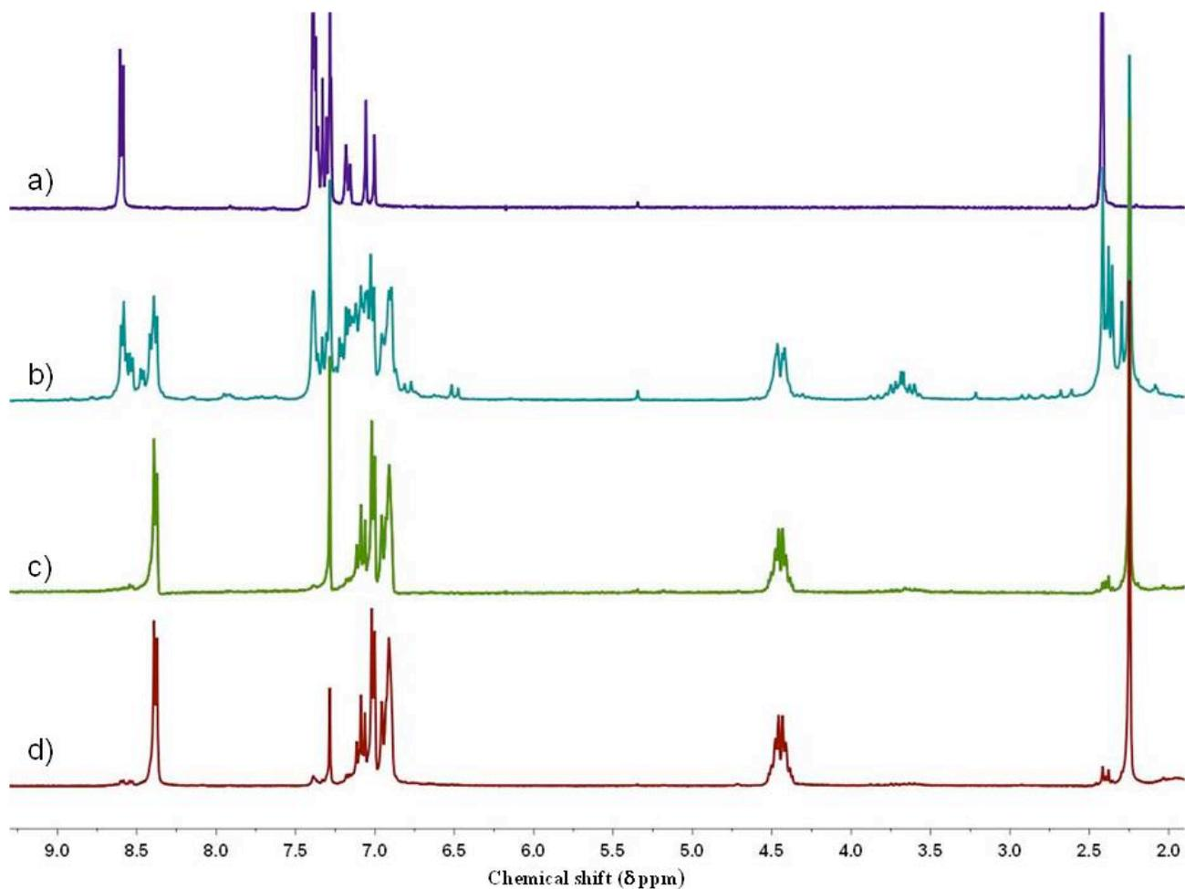
**Figure S8** (a) <sup>1</sup>H NMR in CDCl<sub>3</sub> of 3-methyl-stilbazole, **7** (b) after irradiation of 3-methyl-stilbazole for 37 h in solid state, (c) neutral extract of 3-methyl-stilbazole.HCl, irradiated for 19 h in solid state, (d) neutral extract of 3-methyl-stilbazole.HCl irradiated for 19 h as suspension in hexane.
