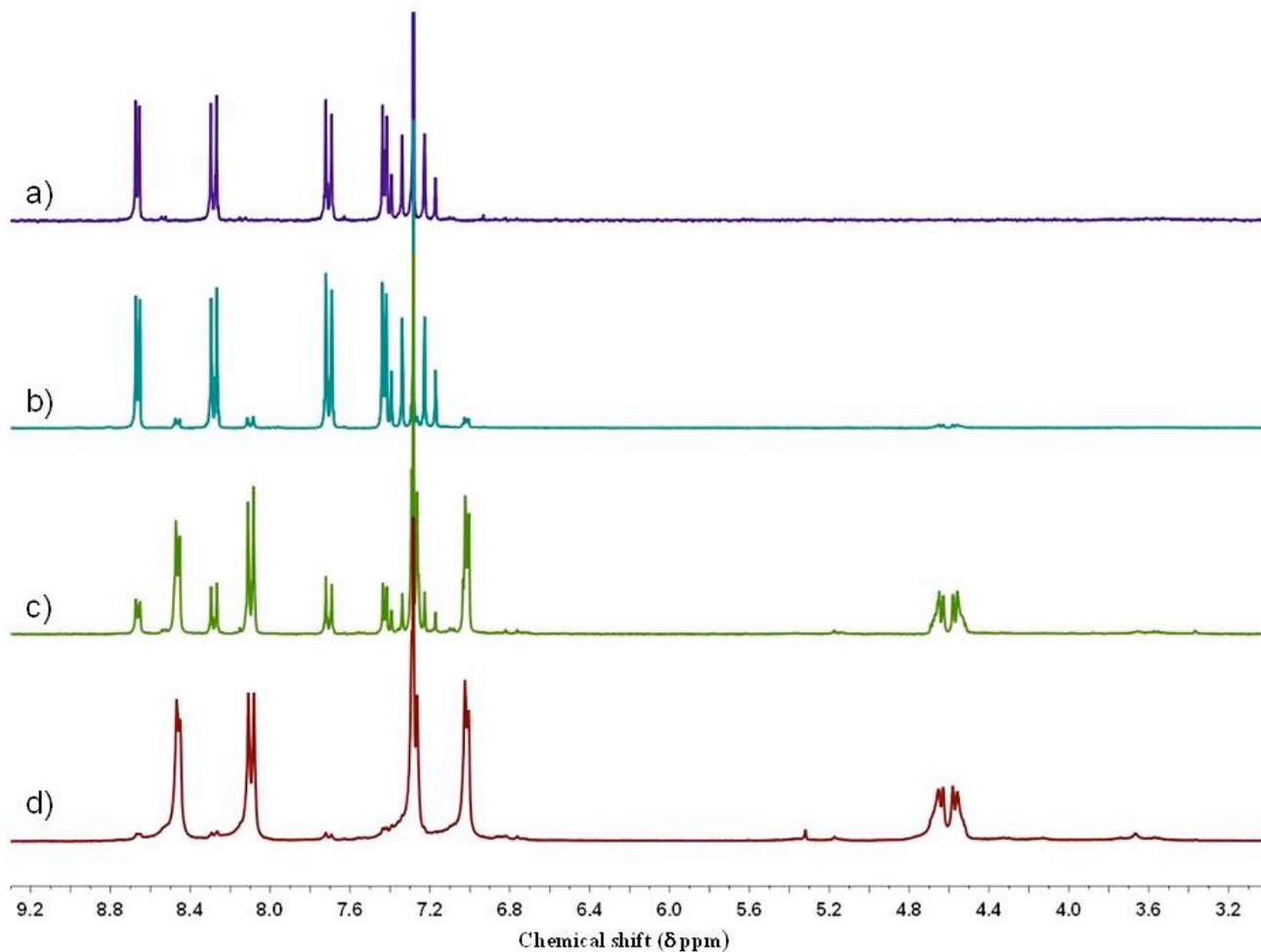
**Figure S13** (a) <sup>1</sup>H NMR in CDCl<sub>3</sub> of 4-NO<sub>2</sub>-stilbazole, **12** (b) after irradiation of 4-NO<sub>2</sub>-stilbazole for 69 h in solid state, (c) neutral extract of 4-NO<sub>2</sub>-stilbazole.HCl, irradiated for 65 h in solid state, (d) neutral extract of 4-NO<sub>2</sub>-stilbazole.HCl irradiated for 150 h as suspension in hexane.
