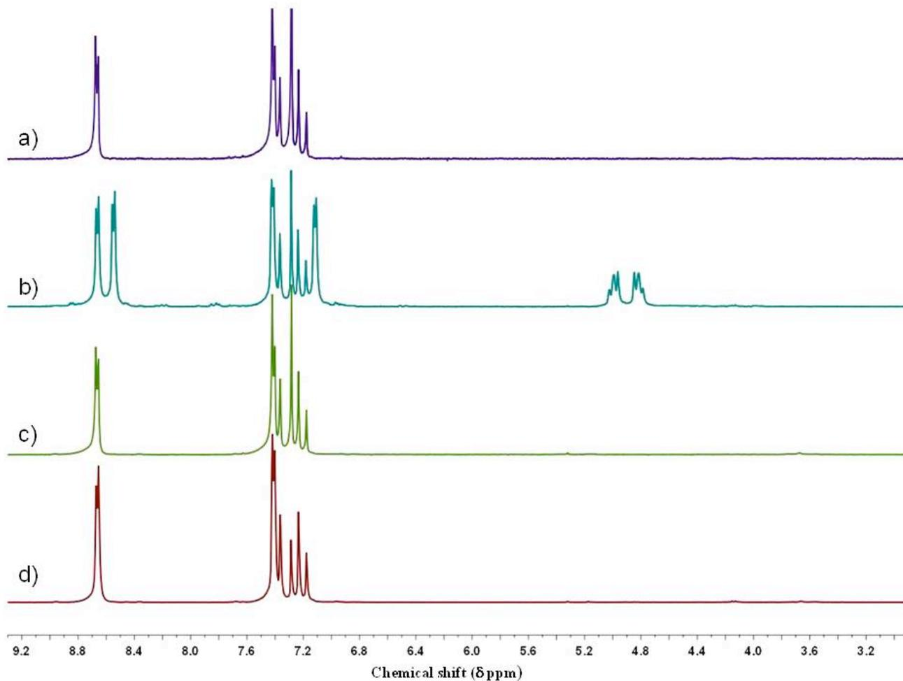
**Figure S17** (a) <sup>1</sup>H NMR in CDCl<sub>3</sub> of 2,3,4,5,6 pentafluoro-stilbazole, **16** (b) after irradiation of 2,3,4,5,6 pentafluoro-stilbazole for 84 h in solid state, (c) neutral extract of 2,3,4,5,6 pentafluoro-stilbazole.HCl, irradiated for 129 h in solid state, (d) neutral extract of 2,3,4,5,6 pentafluoro-stilbazole.HCl irradiated for 84 h as suspension in hexane.
