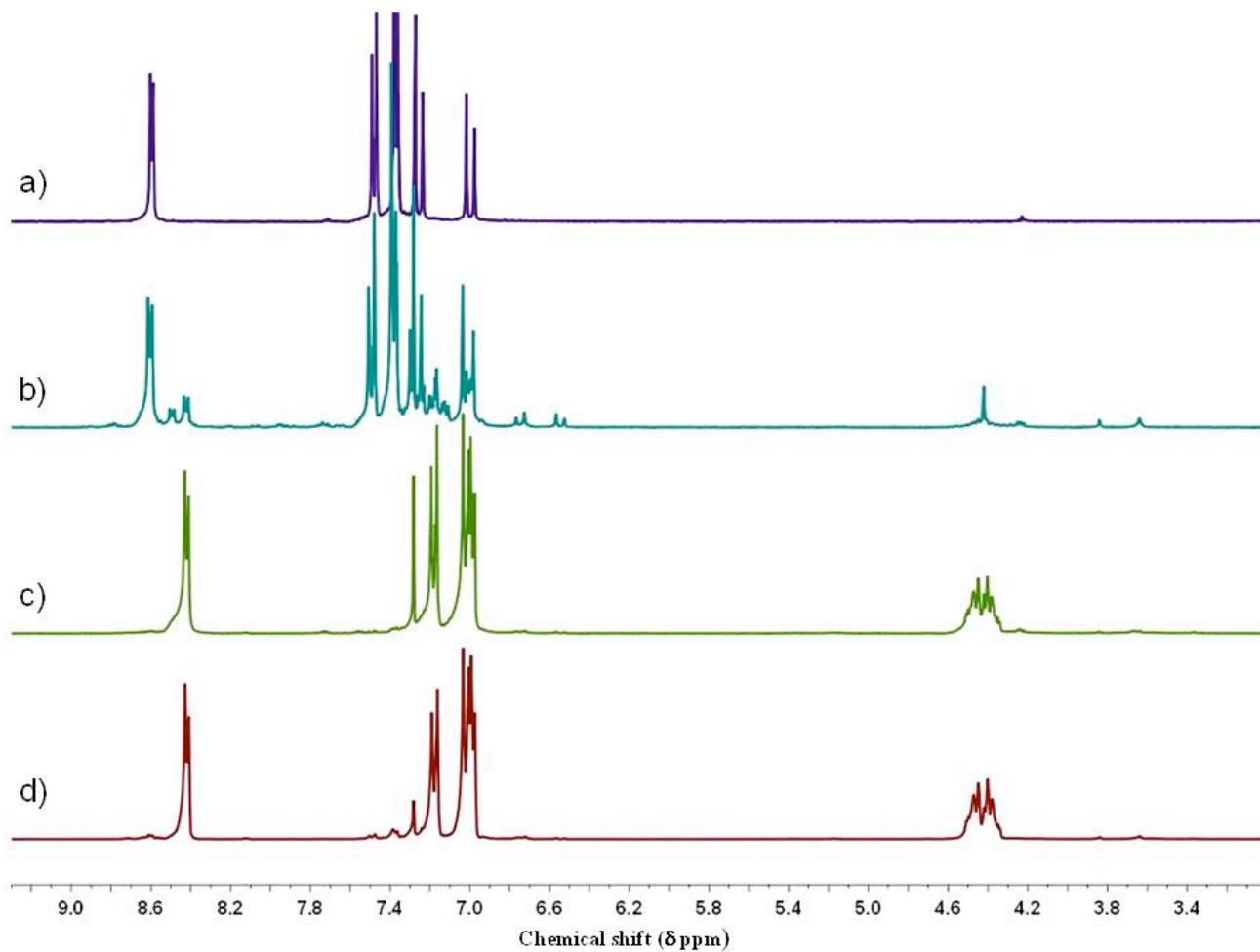
**Figure S4** (a)  $^1\text{H}$  NMR in  $\text{CDCl}_3$  of 4Cl-stilbazole, **3** (b) after irradiation of 4Cl-stilbazole for 52 h in solid state, (c) neutral extract of 4Cl-stilbazole.HCl, irradiated for 44 h in solid state, (d) neutral extract of 4Cl-stilbazole.HCl irradiated for 6 h as suspension in hexane.
