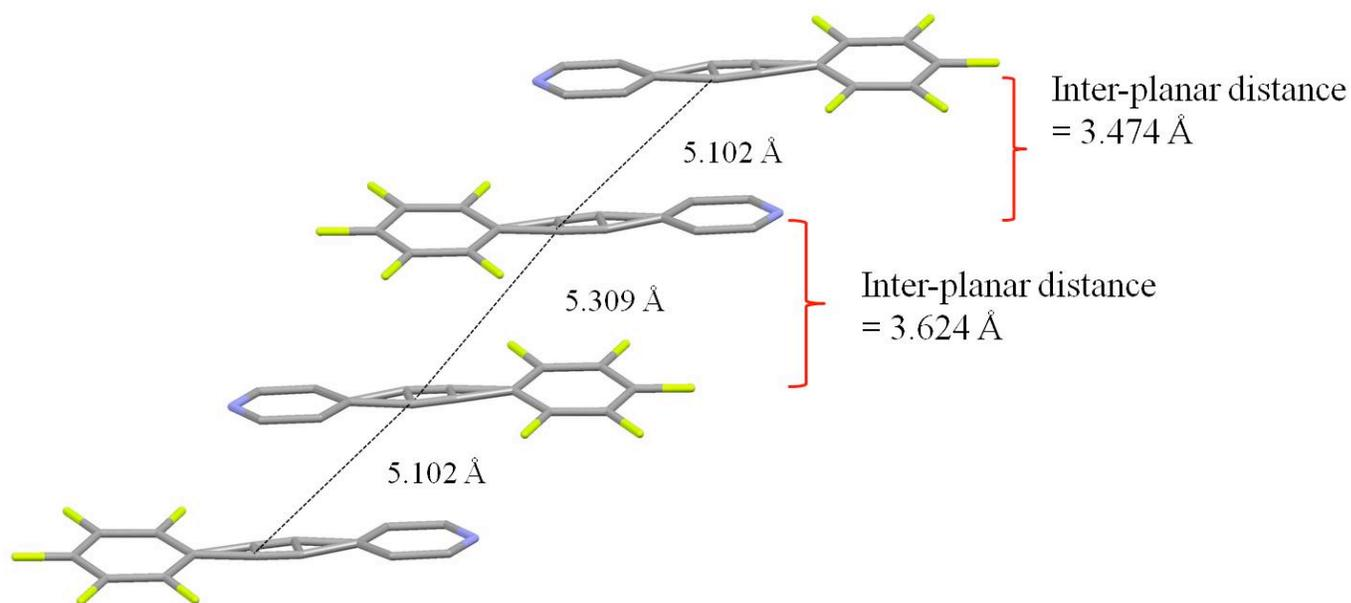
**Figure S28** Packing arrangement of pentafluoro stilbazole.HCl salt. Note the disorder of the olefinic carbons.
