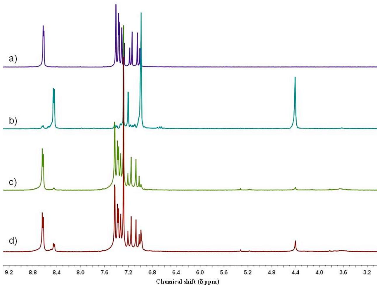
**Figure S15** (a) <sup>1</sup>H NMR in CDCl<sub>3</sub> of 3,5-dichloro-stilbazole, **14** (b) after irradiation of 3,5-dichloro-stilbazole for 96 h in solid state, (c) neutral extract of 3,5-dichloro-stilbazole.HCl, irradiated for 150 h in solid state, (d) neutral extract of 3,5-dichloro-stilbazole.HCl irradiated for 150 h as suspension in hexane.
