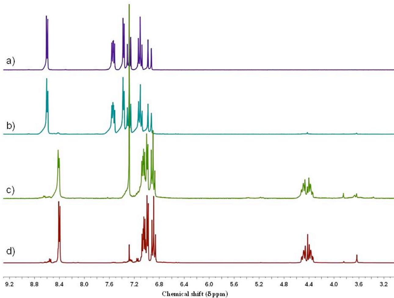
**Figure S3** (a) <sup>1</sup>H NMR in CDCl<sub>3</sub> of 4F-stilbazole, **2** (b) after irradiation of 4F-stilbazole for 52 h in solid state, (c) neutral extract of 4F-stilbazole.HCl, irradiated for 62 h in solid state, (d) neutral extract of 4F-stilbazole.HCl irradiated for 12 h as suspension in hexane.
