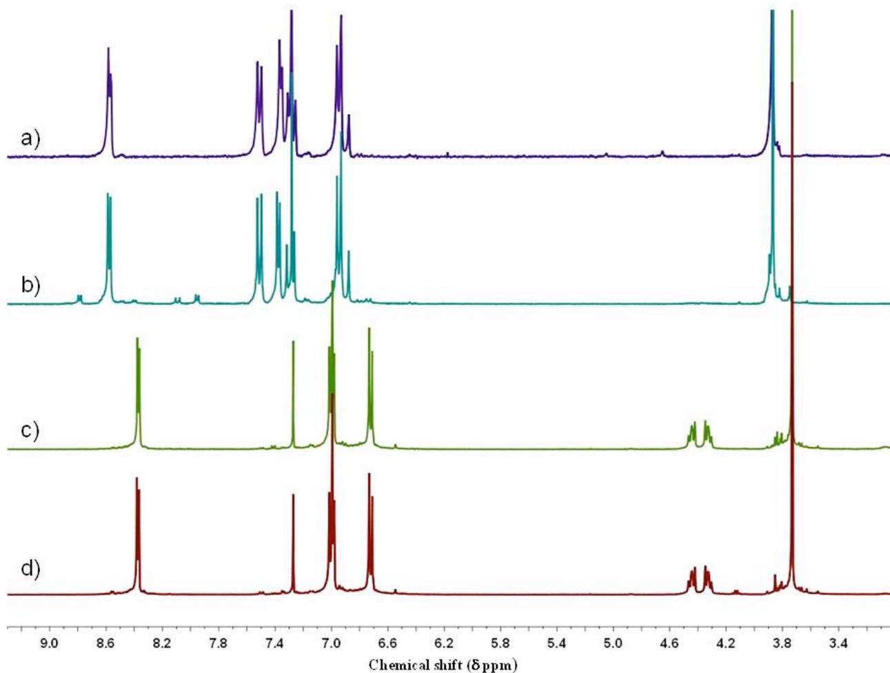
**Figure S10** (a)  $^1\text{H}$  NMR in  $\text{CDCl}_3$  of 4-methoxy-stilbazole, **9** (b) after irradiation of 4-methoxy-stilbazole for 52 h in solid state, (c) neutral extract of 4-methoxy-stilbazole.HCl, irradiated for 60 h in solid state, (d) neutral extract of 4-methoxy-stilbazole.HCl irradiated for 46 h as suspension in hexane.
