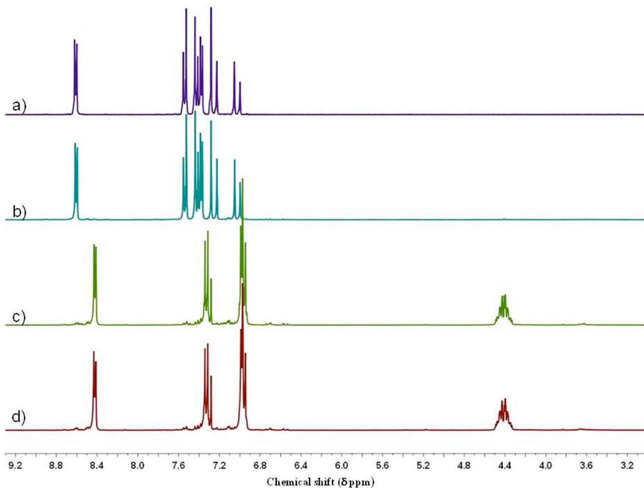
**Figure S5** (a)  $^1\text{H}$  NMR in  $\text{CDCl}_3$  of 4Br-stilbazole, (b) after irradiation of 4Br-stilbazole for 10 h in solid state, (c) neutral extract of 4Br-stilbazole.HCl, irradiated for 5 h in solid state, (d) neutral extract of 4Br-Stilbazole.HCl irradiated for 3 h as suspension in hexane.
