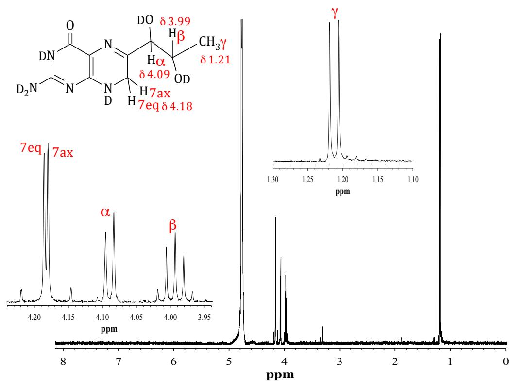
**Fig. 1S** <sup>1</sup>H-NMR spectrum of H<sub>2</sub>Bip in D<sub>2</sub>O (H<sub>2</sub>O signal at 4.8 ppm relative to tetramethylsilane used as an internal reference).
