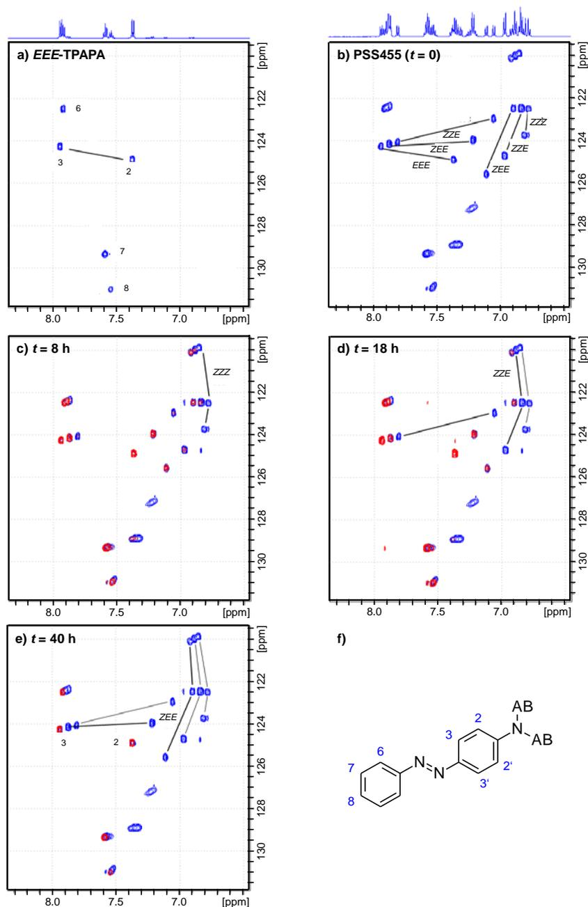
Fig. S2: 2D-HSQC NMR spectra of TPAPA in  $\text{CD}_3\text{CN}$  at  $T = 35^\circ\text{C}$  at different times. a) Spectrum of the pure all-*E* isomer. b) Spectrum of TPAPA in the photostationary state PSS455 ( $t = 0$ ). c) - e) Spectra after  $t = 8, 18,$  and  $40$  h (red), respectively, together with the spectra in the PSS455 (blue) from panel a) for reference. f) Assignments to the five chemically different proton sites for the all-*E* isomer identified by the labels 2, 3, and 6 – 8.
