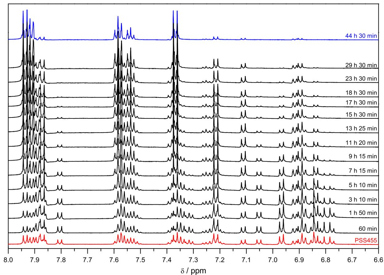
Fig. S1:  $^1\text{H}$  NMR spectra of TPAPA in  $\text{CD}_3\text{CN}$  at  $T = 35^\circ\text{C}$  as function of time after excitation to the photostationary state PSS455 at  $t = 0$ .
